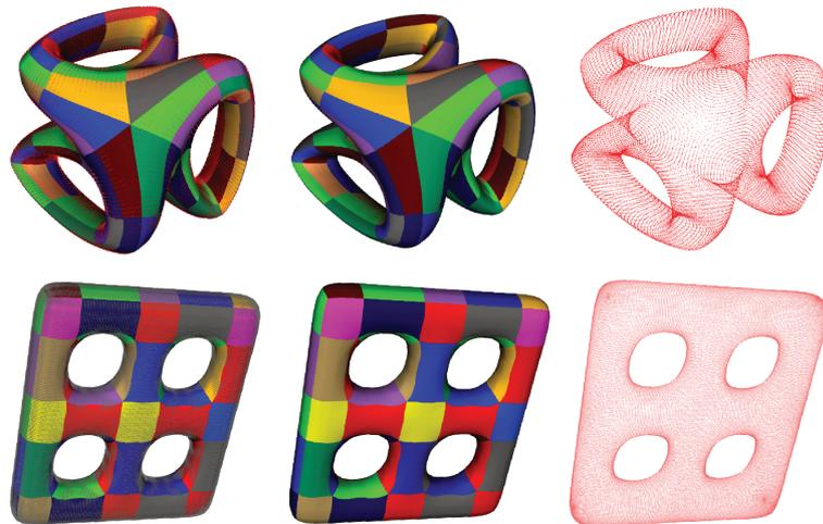
Figure 5.2: Fitting of 3d-geometric objects. The first column is for the cloud of points and the fitting smooth surface, the second one for the fitting surfaces, and the last one is for the cloud of points alone. We use the same basis types as in Fig. 5.1e, with  $F = 144$ ,  $N = 2808$ ,  $P = 36860$ ,  $e_{ave} = 0.00748197$ ,  $e_{max} = 0.0324516$  for the first line example.
