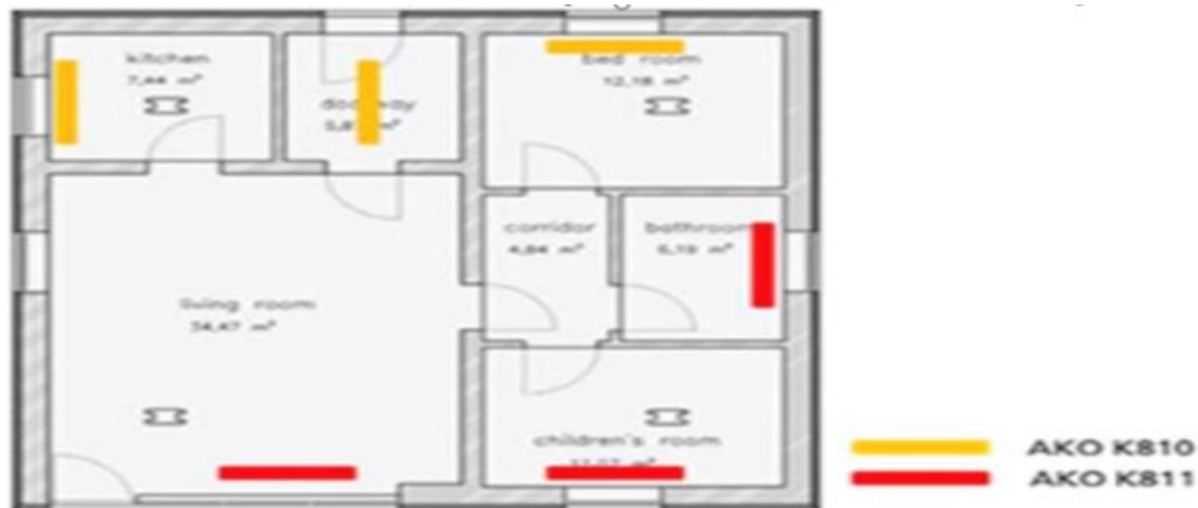
Figure 11.3: Heater locations in Twin house
