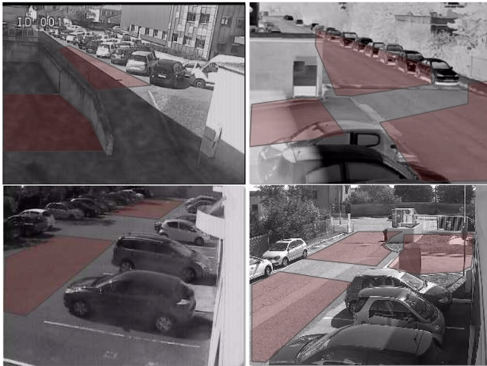
Figure 8.4.1: Four outdoor camera views. Red polygons describe motion analysis areas.
