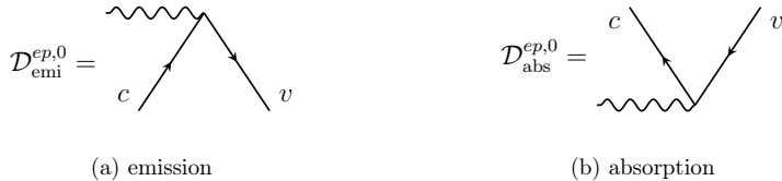
Figure 5.3.1: Single-photon interband transitions: absorption (left diagram) and emission (right diagram). Here, c and v denote an electron (conduction) state and a hole (valence) state respectively.
