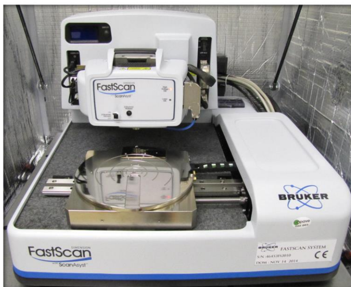
Figure 31: AFM equipment with FastScan system mounted.
