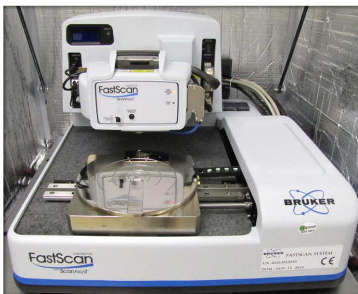
Figure 31: AFM equipment with FastScan system mounted.
