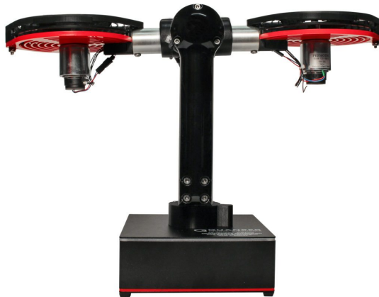
Figure 3.4: Quanser Aero platform in half-quadrotor configuration.
