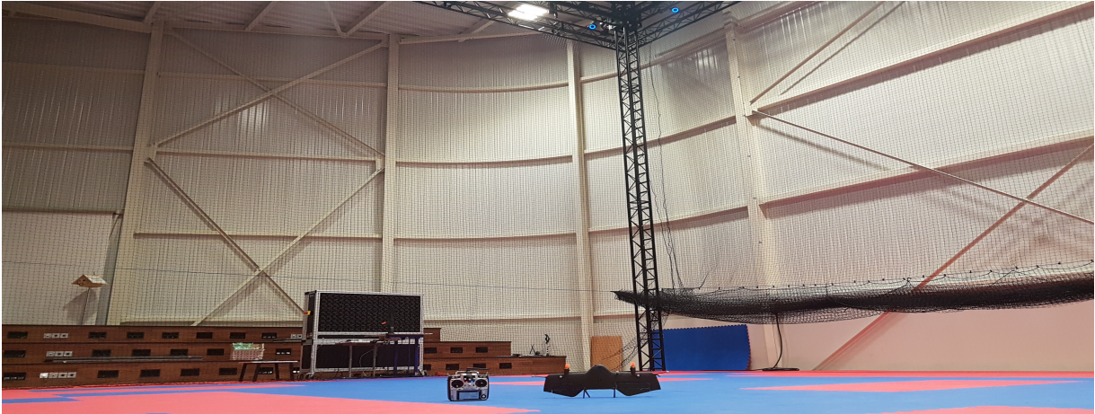
Fig. 15 DarkO Tailsitter MAV at rest in the ENAC's flying arena showing two of sixteen Optitrack cameras in the top and the WindShape wind generator in the background.
