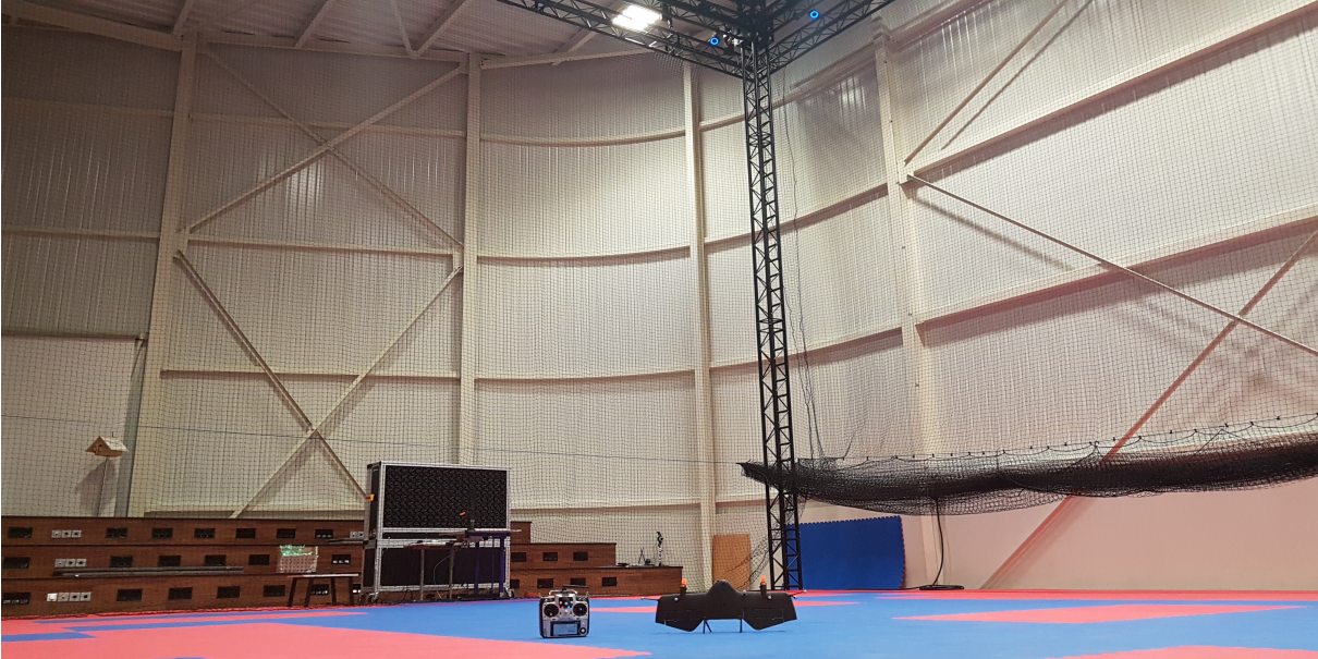
Figure 5.8: Dark0 MAV at rest in the ENAC flying arena showing two of sixteen Optitrack cameras in the top and the WindShape wind generator in the background.
