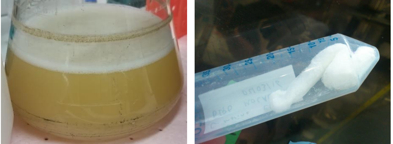
Annexes I.1: EPS obtained after all the production process. On the left, dense bacterial culture, and on the right, lyophilised EPS
