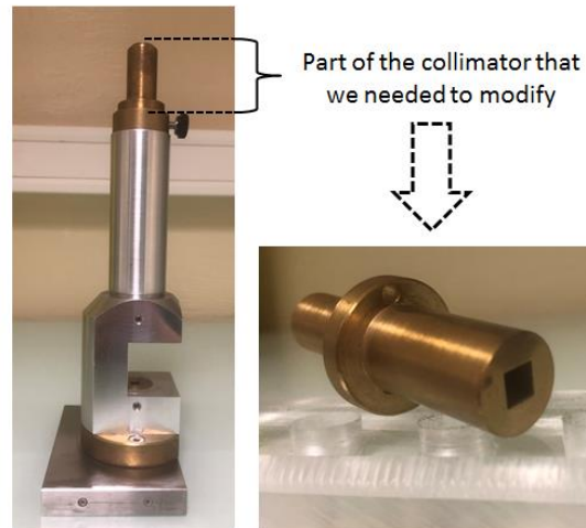
Figure 1: photo of the SARRP collimator (left) and the designed collimator.
