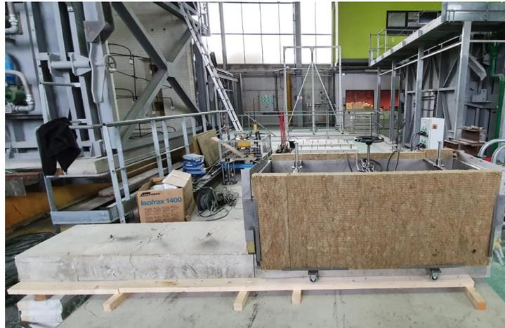
Fig. 120: Heating system on top of a test slab in the fire resistance laboratory at CSTB.
