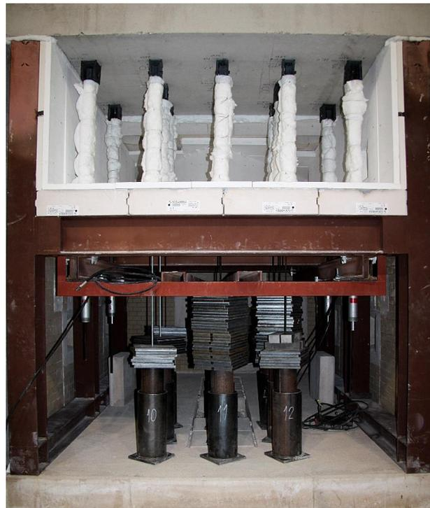
Fig. 95: TU Kaiserslautern's furnace and loading system for fire tests on bonded anchors [20]
