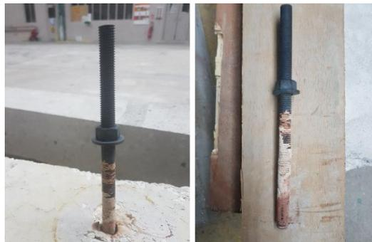
Fig. 55: Illustration of pull-out failure at the steel/resin interface of loaded bonded anchors under fire
