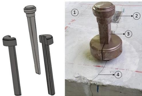
Fig. 115: Wedges used for cracking concrete with: (1) lower side of the slab, (2) thin steel plate, (3) wedges and (4) hairline crack.
