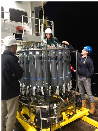
Figure 1: Titanium rosette getting prepared for deployment (on the left) and coming back on deck (on the right). © Lise Artigue
