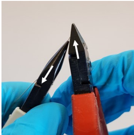
Figure 2.11: Cut-and-pull technique to prepare STM tips. Arrows illustrating the movement to be performed. The flat nose pliers pull back at the same time as the wire cutter cuts and pulls in the indicated direction.
