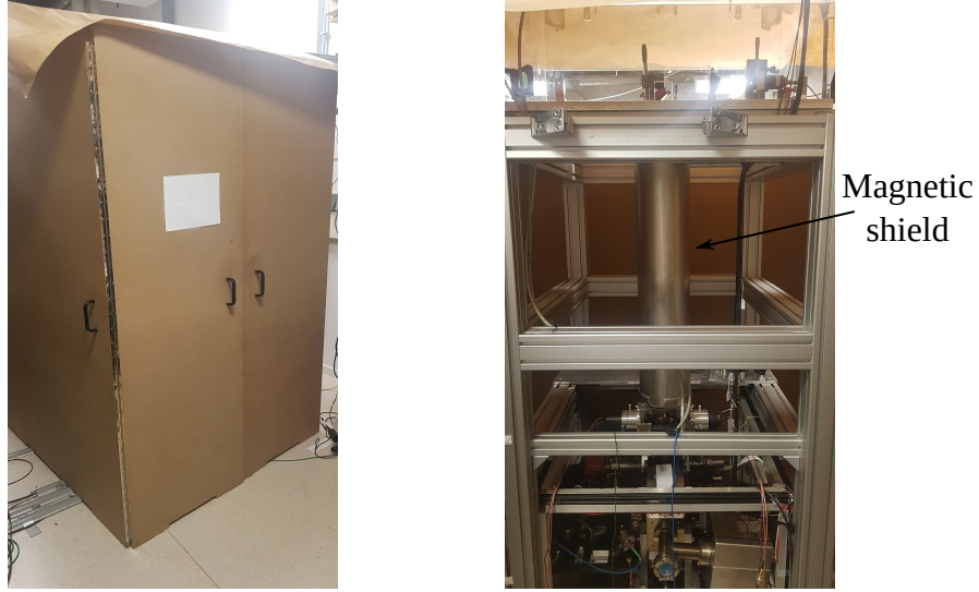
Figure 3.2: Pictures of the experimental setup. On the left: the wood panel box that shields to experiment from environment induced perturbation (mainly the air conditioning system). On the right: inside the wood panels: the interferometry area solenoid is hidden by the magnetic shield. Furthermore, the vacuum cell is surround by Elcom aluminum bars that allow for agile access.
