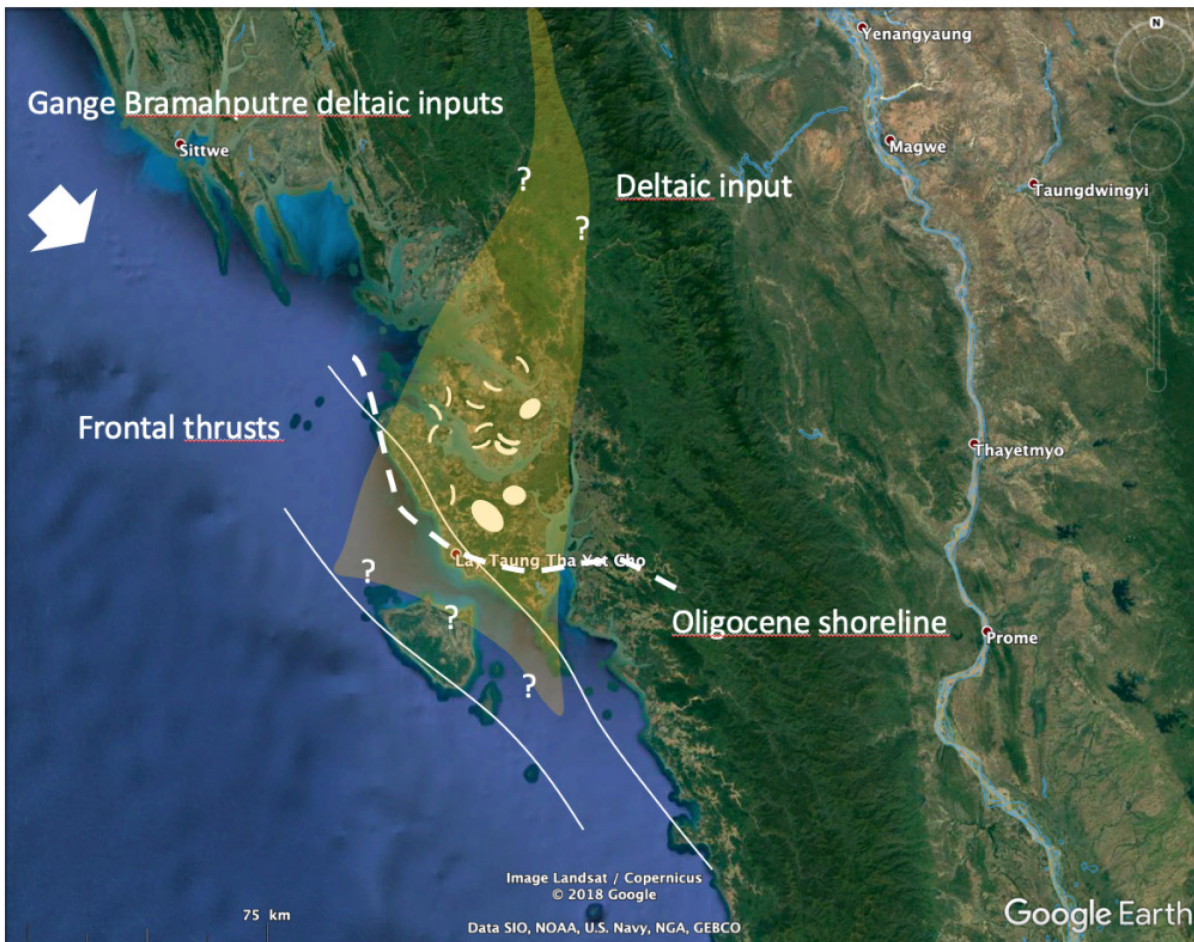
Figure 190: Possible paleo-geographic path related to a northerly directed source of clastics super-imposed on Bengal / Bramahputre clastics forming minibasin-like depo-centers onto the mobile Eocene clays.
