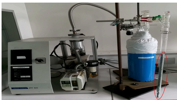
Figure 4.1: A two-stage vacuum pump, consisting of an oil pump and a turbo molecular pump where the silica ampoule (filled with glass materials as highlighted by the red circle) is pumped to achieve vacuum.
