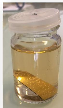
Figure 18: Chemical grafting of carboxybenzene diazonium on gold surface.
