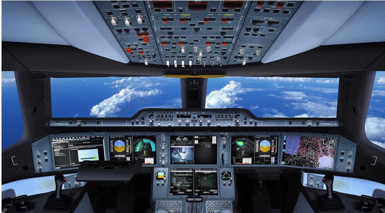
*Figure 2.* Airbus A350 Glass Cockpit
