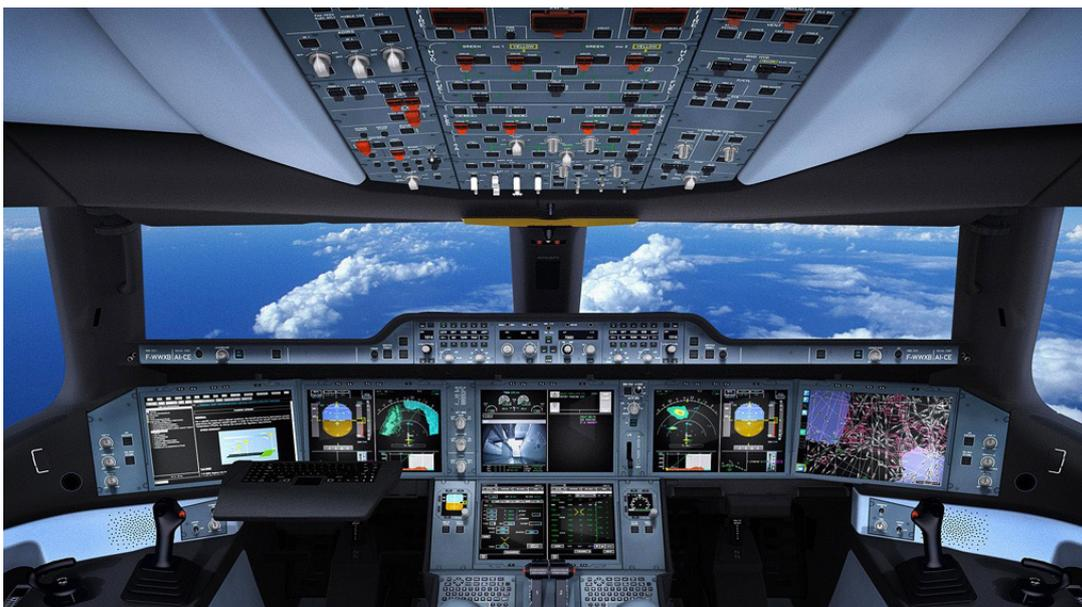
*Figure 2.* Airbus A350 Glass Cockpit
