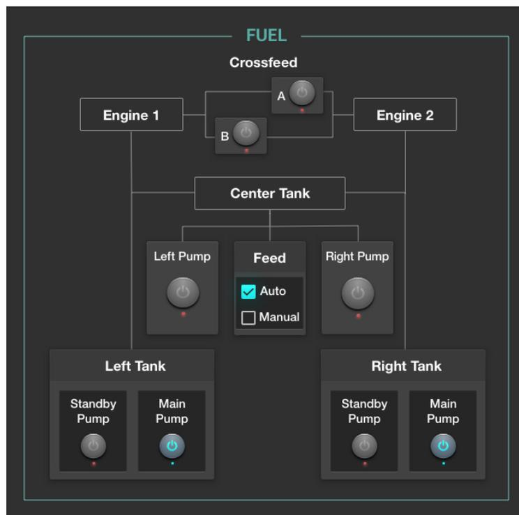
Figure 49. Fuel Zone Architecture in Interface of Experiment 3
