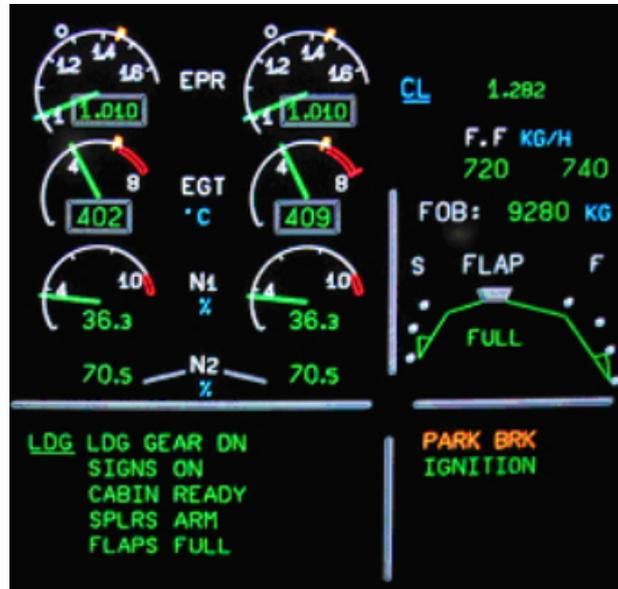
Figure 11. Example of A320 ECAM monitor
