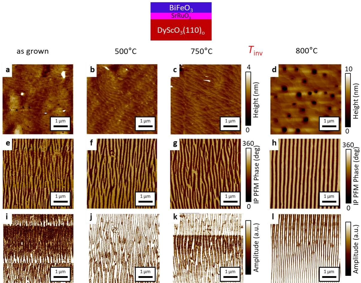
Figure 71 : Experimental observation of the inverse phase transition in the third annealing step at 800°C from the left to the right. **a-d** Topography images, **e-h** in-plane PFM phase and **i-l** corresponding amplitude images.
