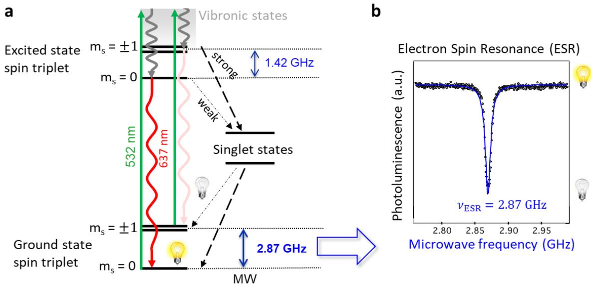
Figure 40 : Optically detectable magnetic resonance (ODMR) explained with **a**, the electronic level structure of the NV centre and **b**, the optical detection of the electron spin resonance spectrum.
