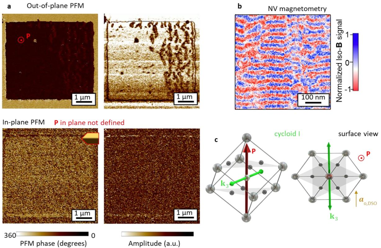
Figure 92 : **a** Written ferroelectric domain, pointing upwards. The absence of the in-plane PFM signal is in line with a vertical polarization. **b** Scanning NV-magnetometry image of a scan inside the written zone and **c** sketches for the corresponding configuration of the polarization  $\mathbf{P}$  and cycloid propagation direction  $\mathbf{k}$ .
