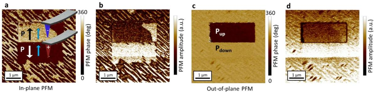
Figure 38 : Illustration of the in-plane control of polarization with the trailing field. **a** In-plane phase and **b** amplitude, **c** out-of-plane phase and **d** amplitude images recorded after trailing the AFM tip first upward (blue arrow in **a**) with a positive bias voltage at the bottom electrode (negative voltage at the tip) and then upward on the bottom half of the square with negative voltage at the bottom electrode (positive voltage at the tip).
