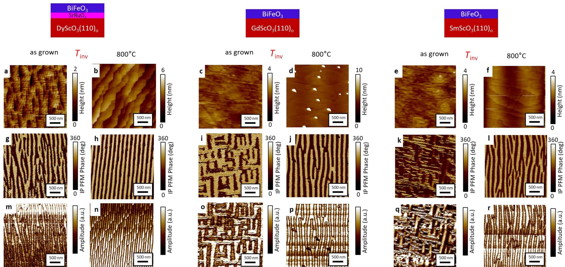
Figure 74 : Generalization of the inverse phase transition in  $\text{BiFeO}_3$  thin films grown on  $\text{DyScO}_3$ ,  $\text{GdScO}_3$  and  $\text{SmScO}_3$  substrates. **a-f** Topography, **g-l** in-plane PFM phase, and **m-r** corresponding amplitude images.
