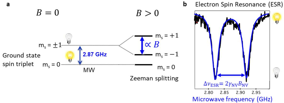
Figure 41 : Magnetic field sensing with a single NV centre. **a** Zeeman splitting of the NV centre ground state in an external magnetic field. **b** The resulting splitting of the dip in the ESR spectrum is proportional to the external magnetic field.
