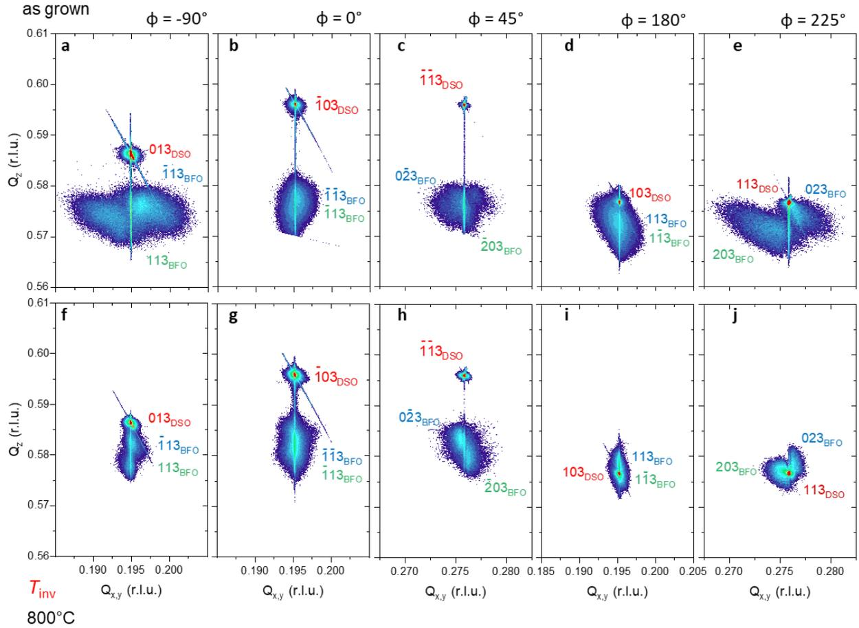
Figure 80 : Asymmetrical reciprocal space maps of a Nd:YAG BiFeO<sub>3</sub> thin film before (a-e) and after annealing (f-j).
