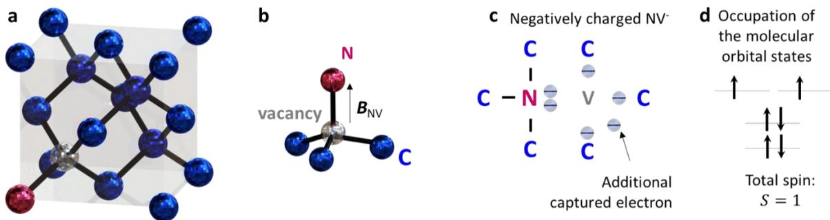
Figure 39 : **a** Nitrogen-vacancy centre in a diamond lattice. **b** Direction of the magnetic field of the NV-centre. **c** Negatively charged colour centre  $\text{NV}^-$ . **d** Occupation of the molecular orbital states.
