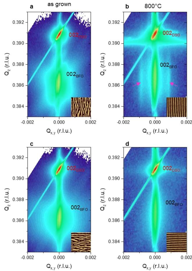
Figure 73 : Reciprocal space maps around the orthorhombic  $\text{DyScO}_3$  ( $002$ )<sub>o</sub> and the monoclinic  $\text{BiFeO}_3$  ( $002$ )<sub>m</sub> peak, before (a,c) and after (b,d) the inverse phase transition for two different orientations of the sample (as shown in inset).
