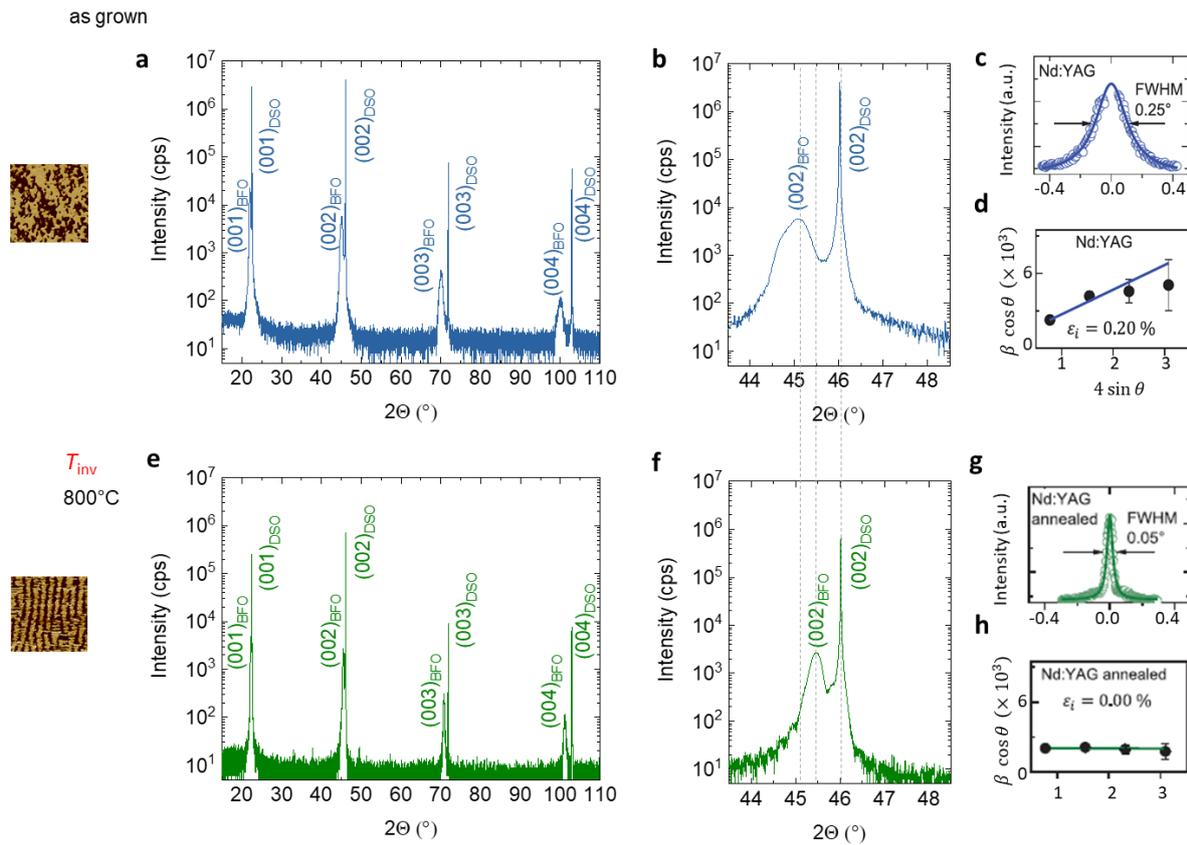
Figure 78 : **a, b, e, f**  $2\theta$ - $\omega$  scans, **c, g** rocking curve and **d, h** out-of-plane Williamson-Hall plots of a mosaic BiFeO<sub>3</sub> film. **a-d** As-grown film and **e-h** annealed sample. The zoomed-in view (**b, f**) around the (002)-BFO-peak shows the change of the form of the film peak after the annealing step. **c, d, g, h** Adapted from reference [128].
