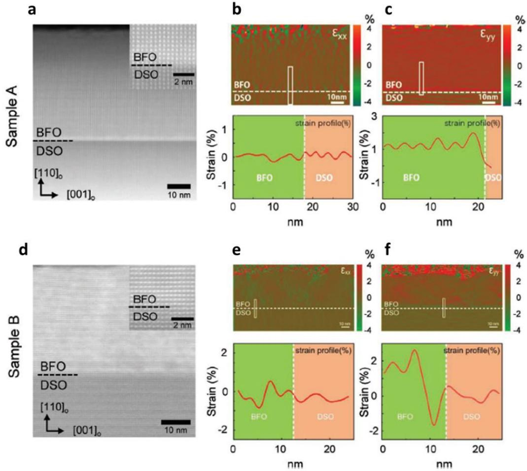
Figure 49 : Determination of strain profiles by HAADF-STEM imaging. **a–c** HAADF image, in-plane strain ( $\epsilon_{xx}$ ), out-of-plane strain ( $\epsilon_{yy}$ ) and corresponding line profiles of marked areas for sample A (excimer). **d–f** HAADF image, in-plane strain ( $\epsilon_{xx}$ ), out-of-plane strain ( $\epsilon_{yy}$ ) and corresponding line profiles of marked areas for sample B (Nd:YAG). Adapted from [128].
