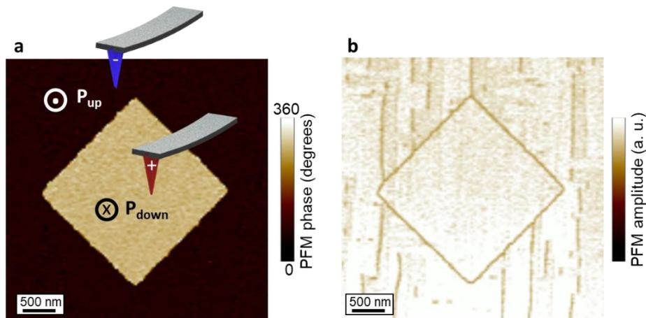
Figure 36 : Switched ferroelectric domains detected by out-of-plane PFM: **a** Out-of-plane PFM phase and **b** amplitude images. We note that the amplitude of the initial upward polarization and the written downward polarization are similar.
