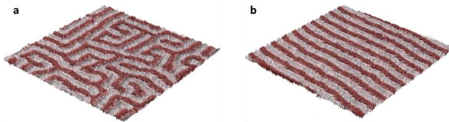
Figure 65 : Fast quenching from the paraelectric state of an ultrathin  $\text{Pb}(\text{Zr}_{0.4}\text{Ti}_{0.6})\text{O}_3$  thin film stabilizes a labyrinthine pattern (a), while slow temperature decrease leads to the parallel striped configuration ground state (b). Adapted from reference [<sup>131</sup>].
