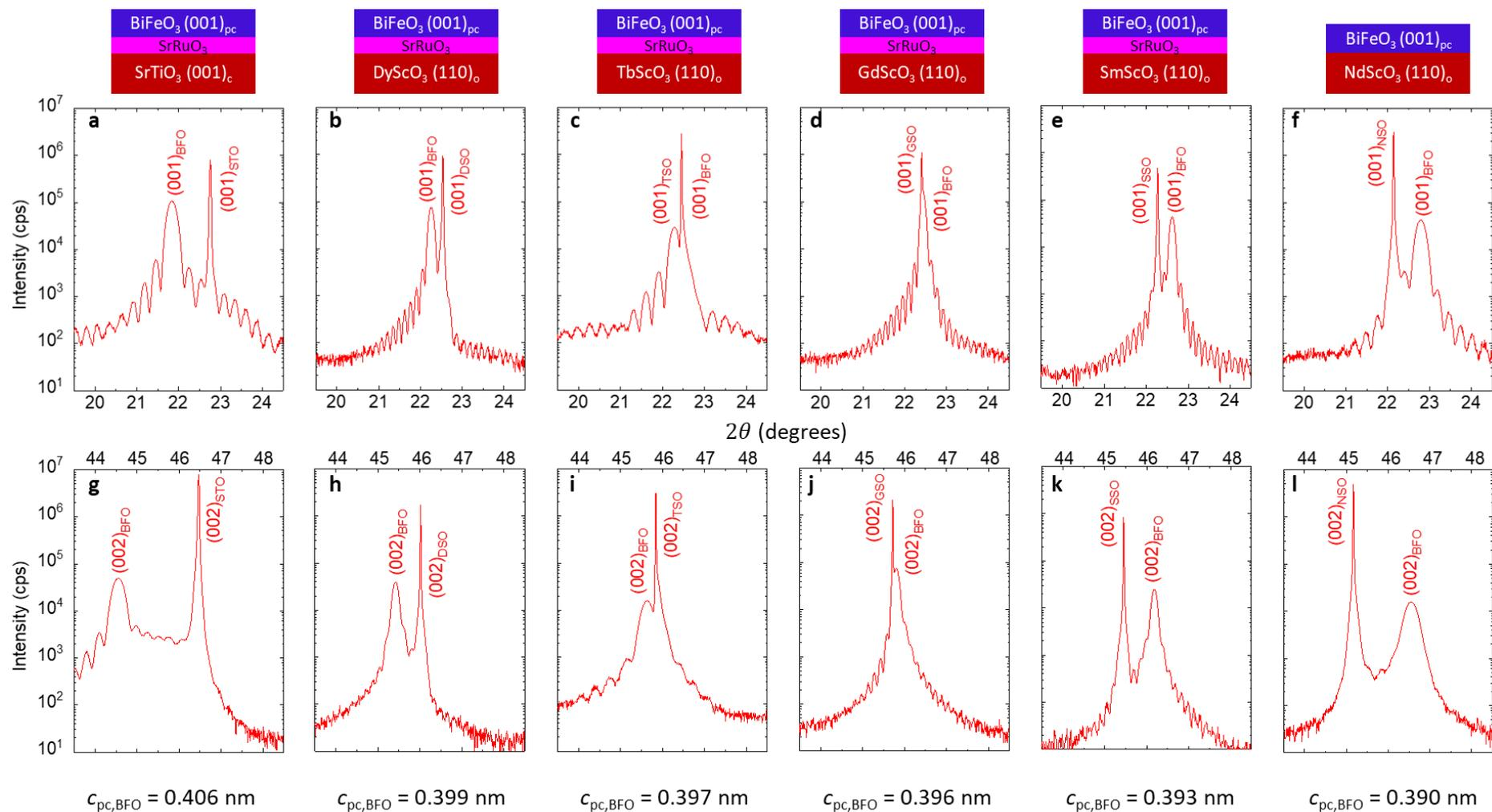
Figure 57:  $2\theta$ - $\omega$  X-ray diffraction patterns around the (001) and (002) pseudo-cubic BFO peaks on the indicated substrates, **a-f** and **g-l**, respectively. The calculated pseudo-cubic out-of-plane lattice parameters are noted below the corresponding measurement.
