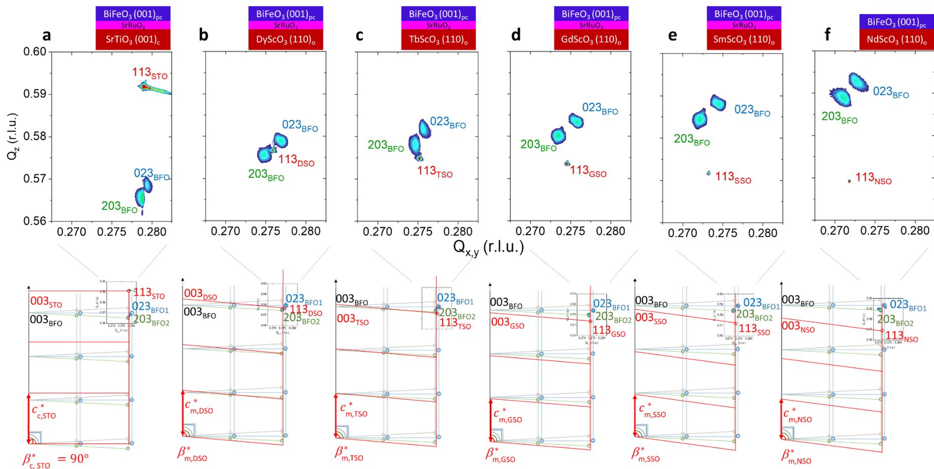
Figure 58: Reciprocal space maps for BiFeO<sub>3</sub> (BFO1 and BFO2) monoclinic domains on SrTiO<sub>3</sub>, DyScO<sub>3</sub>, TbScO<sub>3</sub>, GdScO<sub>3</sub>, SmScO<sub>3</sub> and NdScO<sub>3</sub> around the (113) monoclinic substrate peaks.
