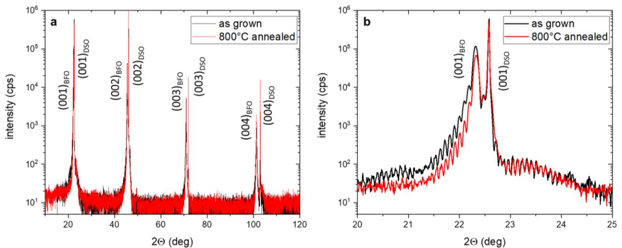
Figure 72 : **a** Full-range  $2\theta$ - $\omega$  scans of the sample in the as-grown state, as well as after the annealing step at 800°C. **b** zoom-in at the orthorhombic  $\text{DyScO}_3$  (001)<sub>o</sub> and the monoclinic  $\text{BiFeO}_3$  (001)<sub>m</sub> peak.
