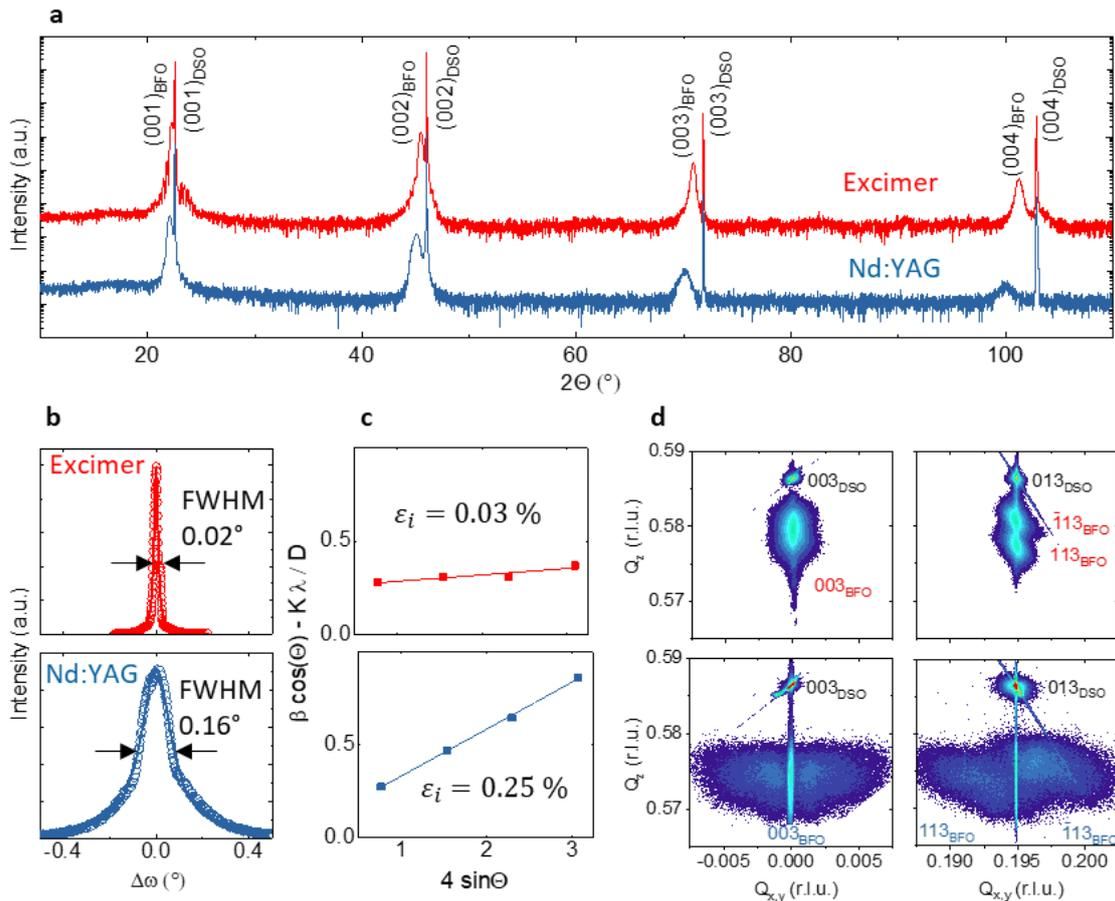
Figure 48 : Structural properties of  $\text{BiFeO}_3$  films grown by the KrF excimer laser and the Nd:YAG laser. **a**  $2\theta$ - $w$  scans, **b** rocking curves, **c** Williamson-Hall plots and **d** reciprocal space maps.
