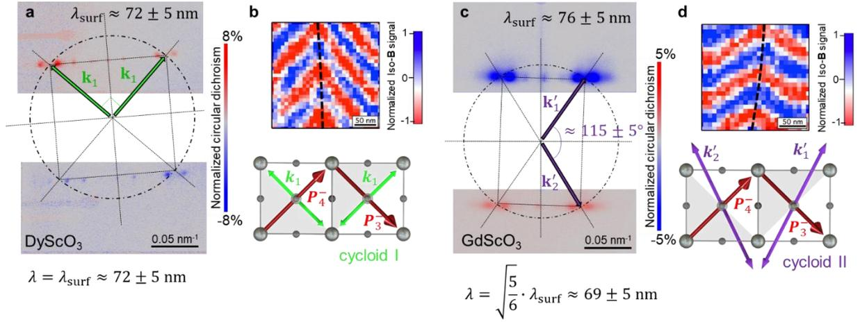
Figure 84 : The two types of spin cycloids in real and reciprocal spaces. **a, c** X-ray resonant magnetic scattering at the Fe L-edge for BiFeO<sub>3</sub> grown on DyScO<sub>3</sub> and GdScO<sub>3</sub>, respectively. **b, d** Corresponding NV magnetometry image zoomed in, with the propagation vectors sketched for both polarization variants. Figure adapted from reference [136].
