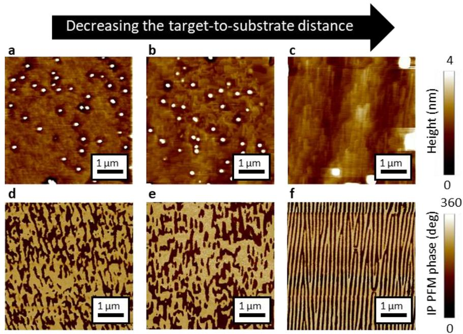
Figure 52 :  $\text{BiFeO}_3/\text{SrRuO}_3$  heterostructures deposited on  $\text{DyScO}_3(110)_0$  while decreasing the target-to-substrate distance. **a-c** Topography, **d-f** in-plane PFM phase. The target-to-substrate distance is decreased by 1.5 cm at each step.
