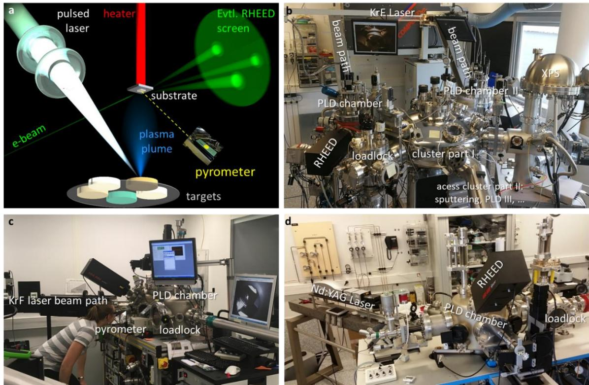
Figure 21 : **a** Schematic representation of the PLD process. **b-d** Four different growth chambers in our lab.
