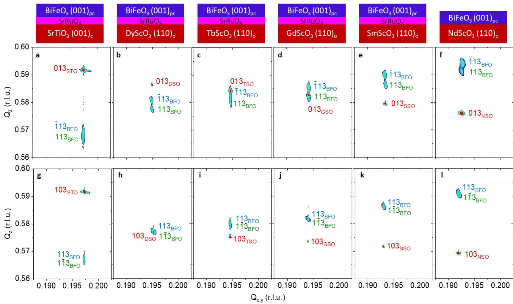
Figure 59 : Reciprocal space maps along around **a-f** the (013) and **g-l** (103) substrate peaks of  $\text{SrTiO}_3$ ,  $\text{DyScO}_3$ ,  $\text{TbScO}_3$ ,  $\text{GdScO}_3$ ,  $\text{SmScO}_3$  and  $\text{NdScO}_3$ .
