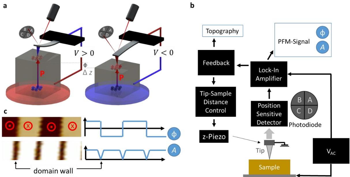
Figure 33: Schematic **a** and working principle **b** of a piezoresponse force microscope. **c** Output phase and amplitude on four domains with alternated up and down polarization states.
