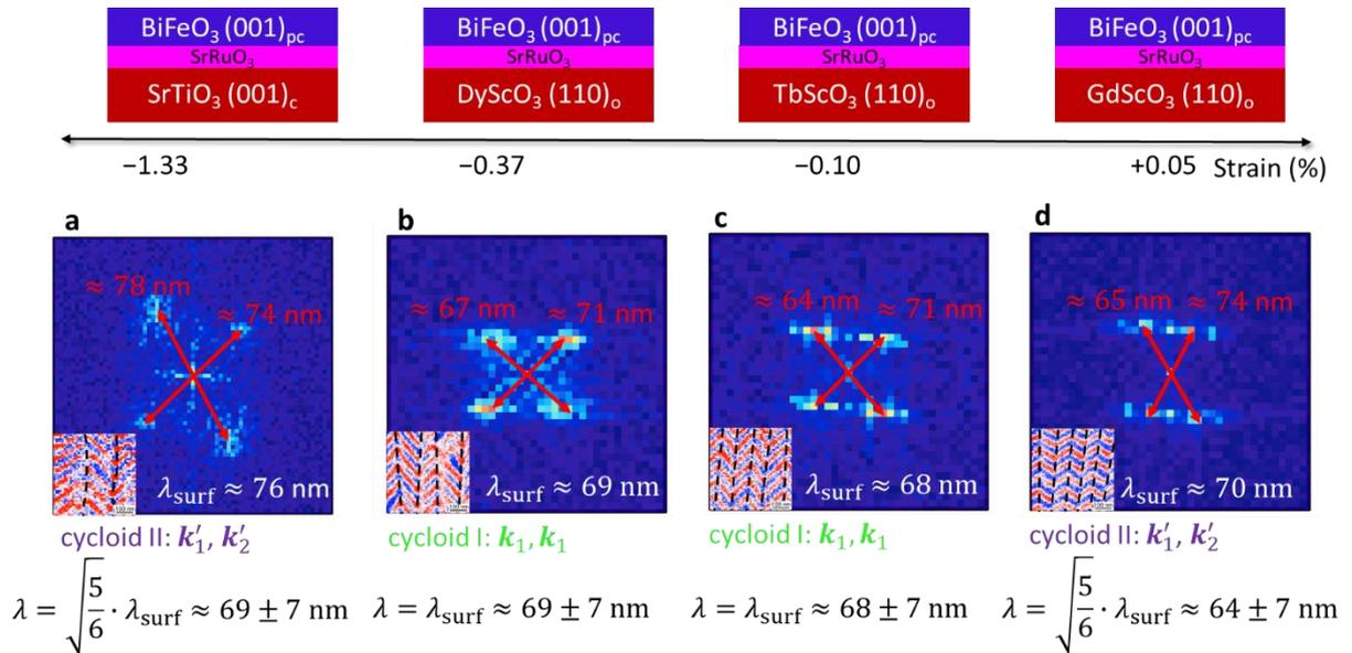
Figure 83 : Fourier transformations of the scanning NV magnetometry images on cycloidal states in Figure 82g-j. Calculated cycloid wavelengths  $\lambda$  from the projections on the surface ( $\lambda_{surf}$ ) for samples grown on **a** SrTiO<sub>3</sub>, **b** DyScO<sub>3</sub>, **c** TbScO<sub>3</sub> and **d** GdScO<sub>3</sub>.
