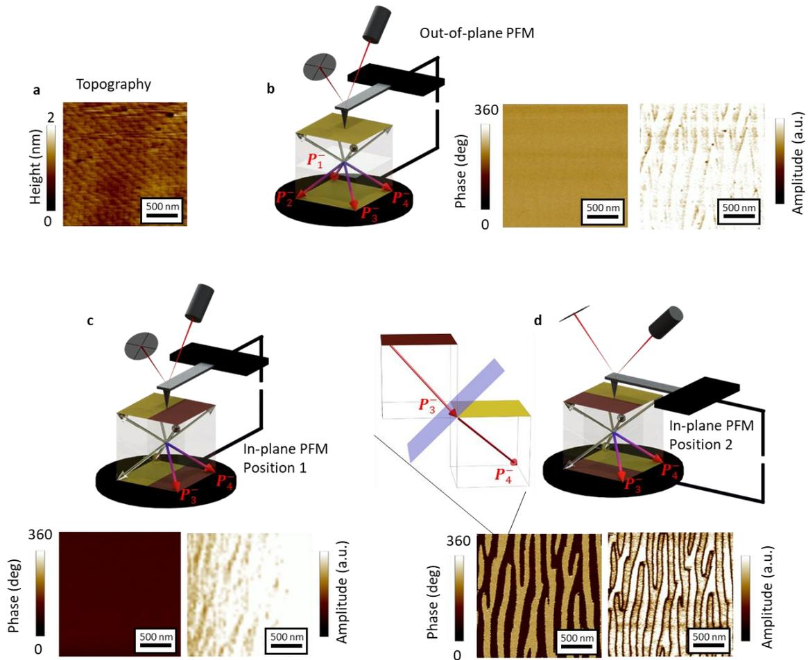
Figure 46: Vectorial PFM analysis of a striped  $\text{BiFeO}_3$  thin film grown on  $\text{DyScO}_3(110)_o$  with an excimer laser. **a** Surface topography, **b** out-of-plane PFM phase and amplitude, **c**, **d** in plane PFM phase and amplitude for two different probe-to-sample configurations, show  $\mathbf{P}_3^-$  and  $\mathbf{P}_4^-$  polarization directions.
