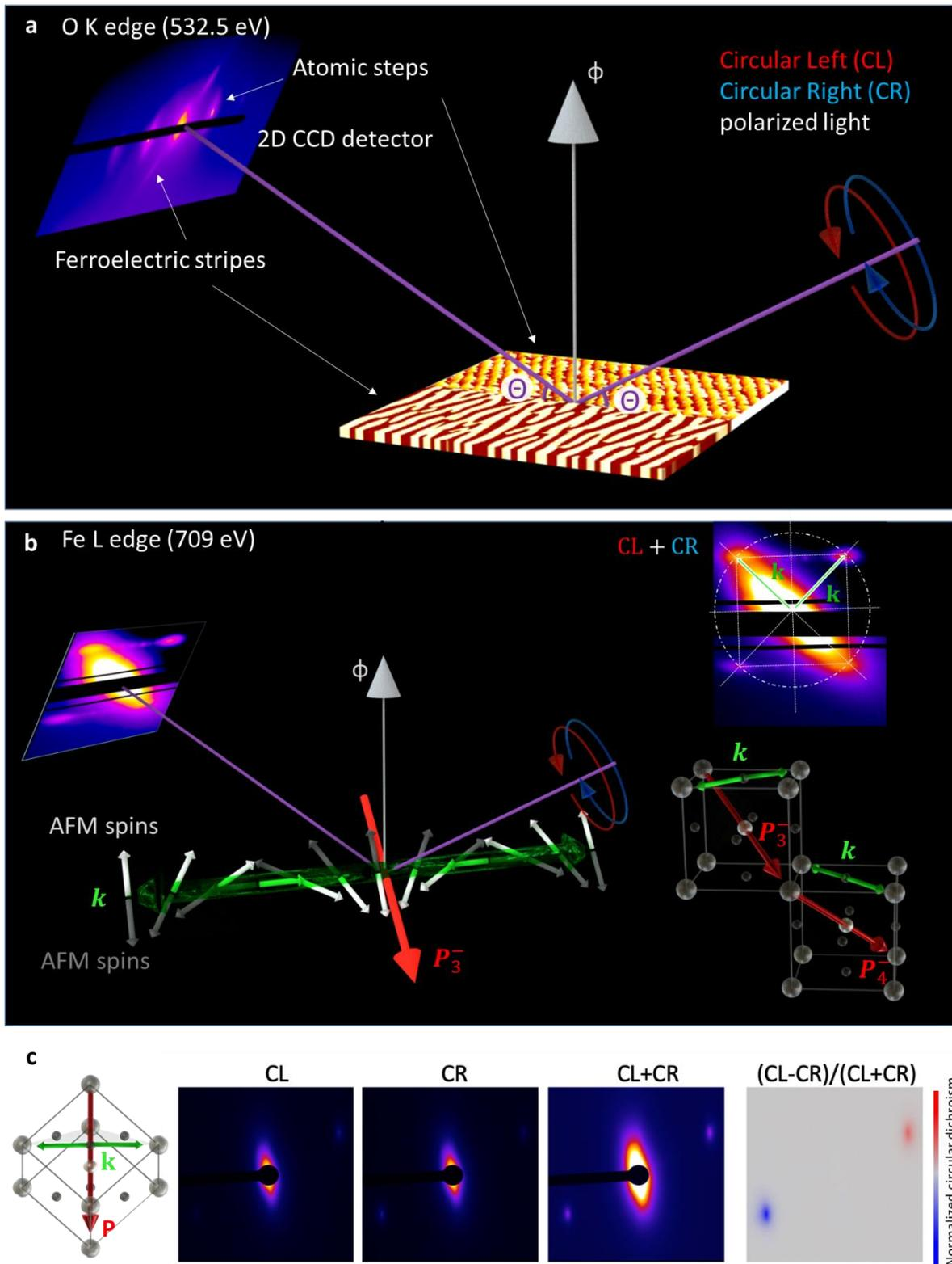
Figure 43 : Resonant elastic X-ray scattering experiment at **a** the oxygen K edge to investigate the structural/ferroelectric domains and domain walls and **b** at the iron L edge to determine the magnetic properties of the sample, such as the spin cycloid in  $\text{BiFeO}_3$ . **c** Normalization of the dichroic pattern to determine the circular dichroism (blue and red contrast in the last picture) at the iron L edge. Example shown for a single cycloid propagation direction.
