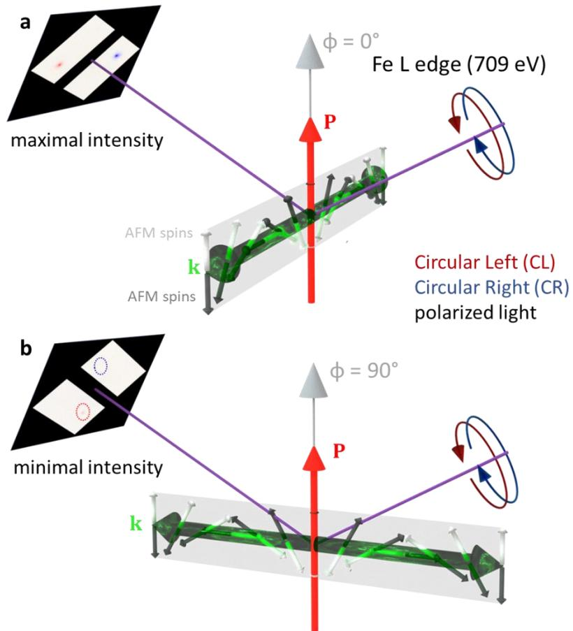
Figure 45 : Circular dichroism measured at the Fe L-edge for different azimuthal orientations  $\Phi$ , illustrated for a (111)  $\text{BiFeO}_3$  sample with polarization perpendicular to the sample surface and a cycloid propagating along  $k$  in the film plane. The image on the detector is the calculated normalized dichroism. **a** Maximal intensity in the diffraction pattern and horizontal spots, **b** minimal intensity and vertical spots (dotted circles indicate the positions).
