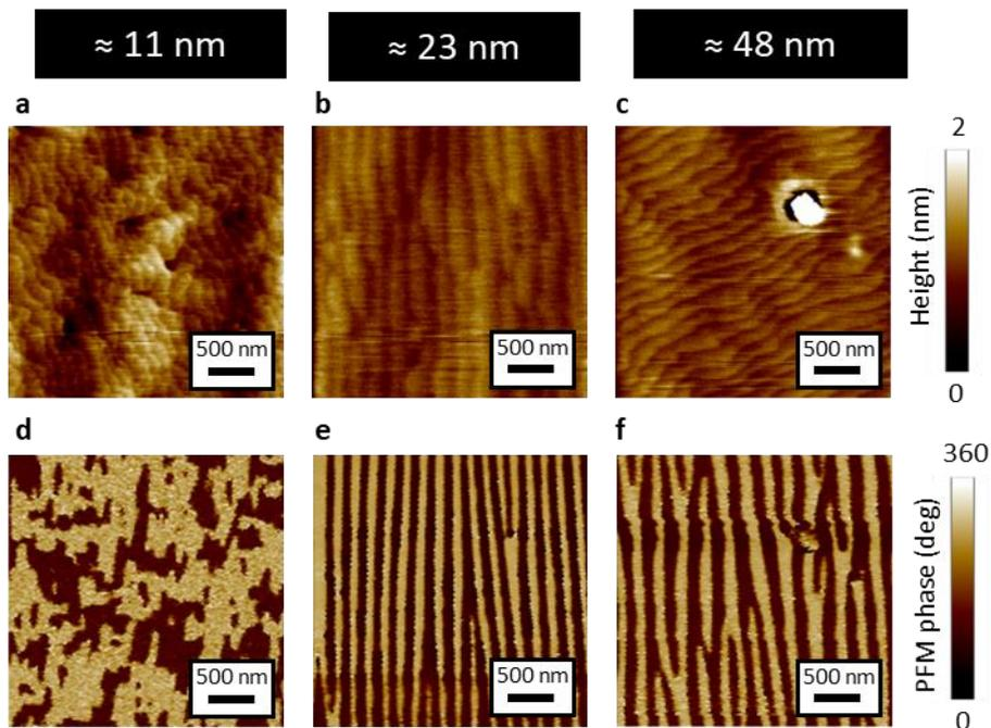
*Figure 54 : BiFeO<sub>3</sub>/SrRuO<sub>3</sub> heterostructures deposited on DyScO<sub>3</sub>(110)<sub>0</sub> while increasing the thickness of BiFeO<sub>3</sub>. **a-e** Topography, **f-j** in-plane PFM phase.*
