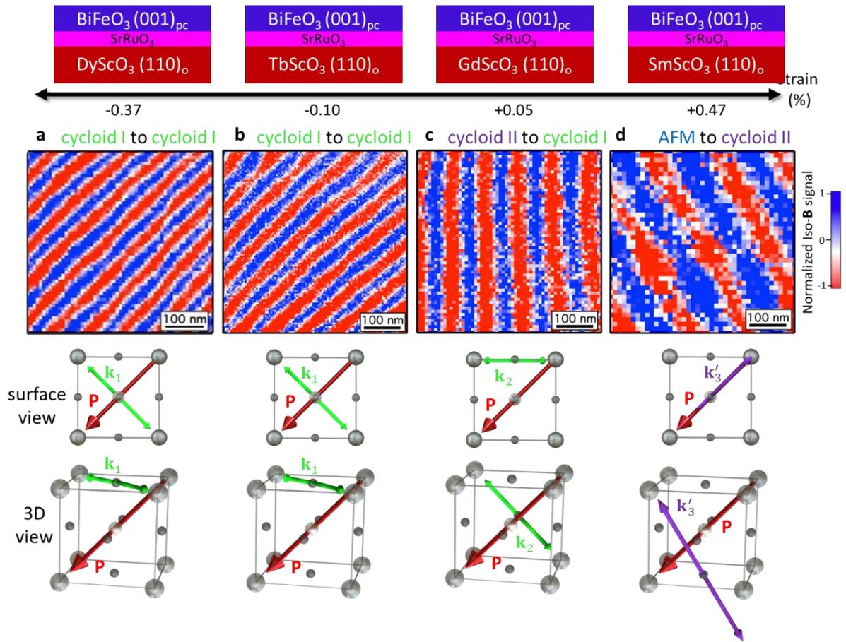
Figure 88 : Magnetic textures in electrically written single ferroelectric domains. **a-d** Corresponding NV magnetometry images and sketches of the propagation vectors in the written zones of the BiFeO<sub>3</sub> thin films grown on DyScO<sub>3</sub>, TbScO<sub>3</sub>, GdScO<sub>3</sub> and SmScO<sub>3</sub>, shown in Figure 86 and Figure 87, respectively. Figure adapted from reference [<sup>136</sup>].
