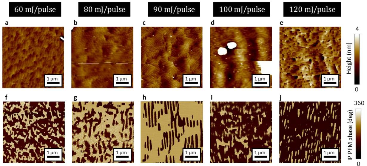
Figure 50:  $\text{BiFeO}_3/\text{SrRuO}_3$  heterostructures deposited on  $\text{DyScO}_3(110)_o$  while increasing the laser energy per pulse for  $\text{BiFeO}_3$ . **a-e** Topography, **f-j** in-plane PFM phase.
