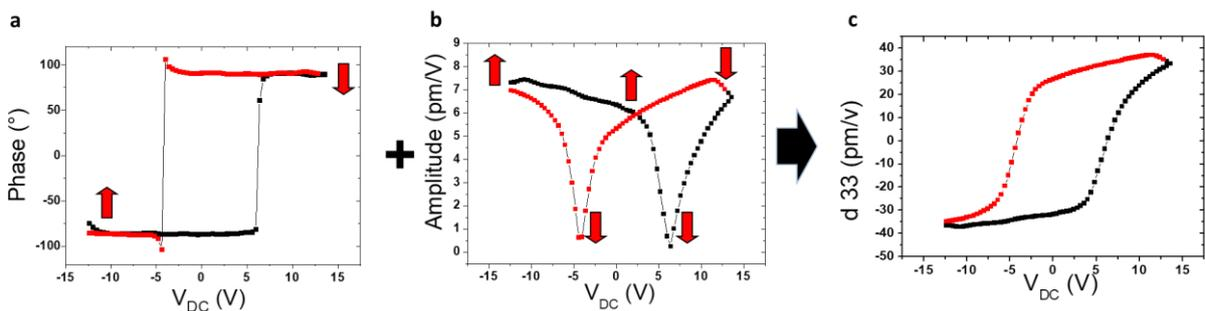
Figure 34: Local piezoelectric hysteresis loop collected with PFM. **a**, PFM phase and **b**, amplitude after applying rectangular voltage pulses of varying amplitude. The red arrows denote the polarization direction. **c**, Combined  $d_{33}$  vs. voltage.
