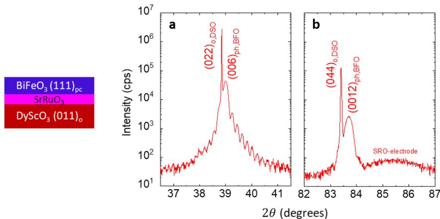
Figure 62 : 2θ-ω X-ray diffraction patterns around the pseudo-hexagonal (006)<sub>ph</sub> and (0012)<sub>ph</sub> BiFeO<sub>3</sub> peaks on the orthorhombic DyScO<sub>3</sub> (011)<sub>o</sub> substrate.
