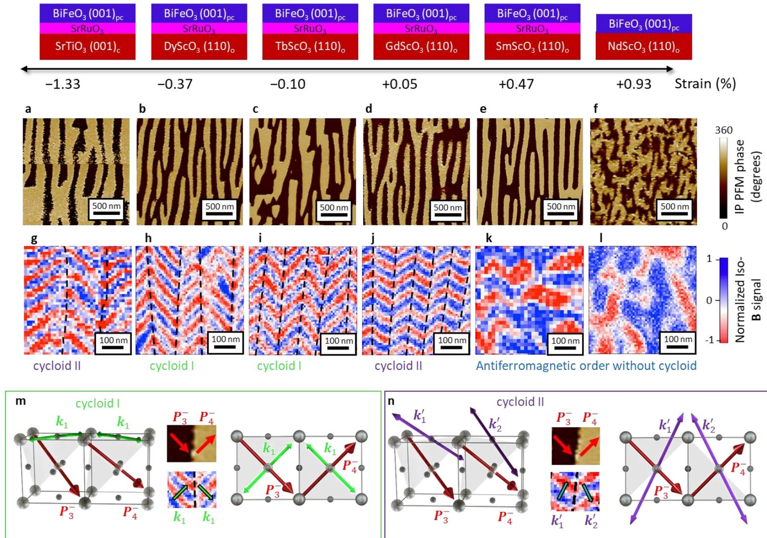
Figure 82 : **a-f** In-plane PFM phase images of BiFeO<sub>3</sub> films grown on substrates imposing different epitaxial strain. **g-l** Corresponding NV-magnetometry images. **m,n** Sketches in side and top views to explain the relation between the ferroelectric variants  $P_3^-$  and  $P_4^-$  and the magnetic zig-zag patterns for cycloid type I and II, respectively. Figure adapted from reference [136].
