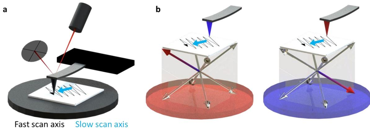
Figure 37 : **a** Fast scan axis of a moving tip (black arrow) and slow scan axis (blue arrow). **b** Switching of the polarization with a trailing field. The in-plane polarization component becomes parallel to the slow scan axis for positive bias at the bottom electrode (negative voltage at the tip) and antiparallel to it for negative bias at the bottom electrode (positive voltage at the tip).
