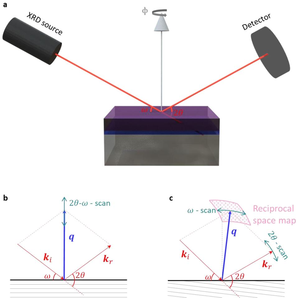
Figure 22 : **a** Measurement geometry of the X-ray diffractometer. **b** Symmetric  $2\theta$ - $\omega$  scan. **c** Asymmetric reciprocal space map, spanned by the  $2\theta$  and  $\omega$  scan direction.
