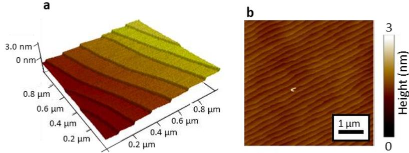
Figure 31 : AFM measurements of terraces and atomic steps on the surface of single crystalline  $\text{DyScO}_3$  substrate. **a** 3D-view of a  $1 \times 1 \mu\text{m}^2$  sample, **b** 2D-view of a  $5 \times 5 \mu\text{m}^2$  scan.
