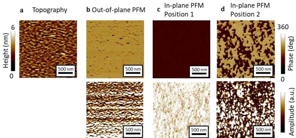
Figure 47: Vectorial PFM analysis of a  $\text{BiFeO}_3$  thin film grown on  $\text{DyScO}_3(110)_o$  with a Nd:YAG laser. **a** Surface topography, **b** out-of-plane PFM phase and amplitude, **c**, **d** in plane PFM phase and amplitude for two different probe-to-sample configurations, show as well  $\mathbf{P}_3^-$  and  $\mathbf{P}_4^-$  polarization directions, but ordered in a mosaic pattern.
