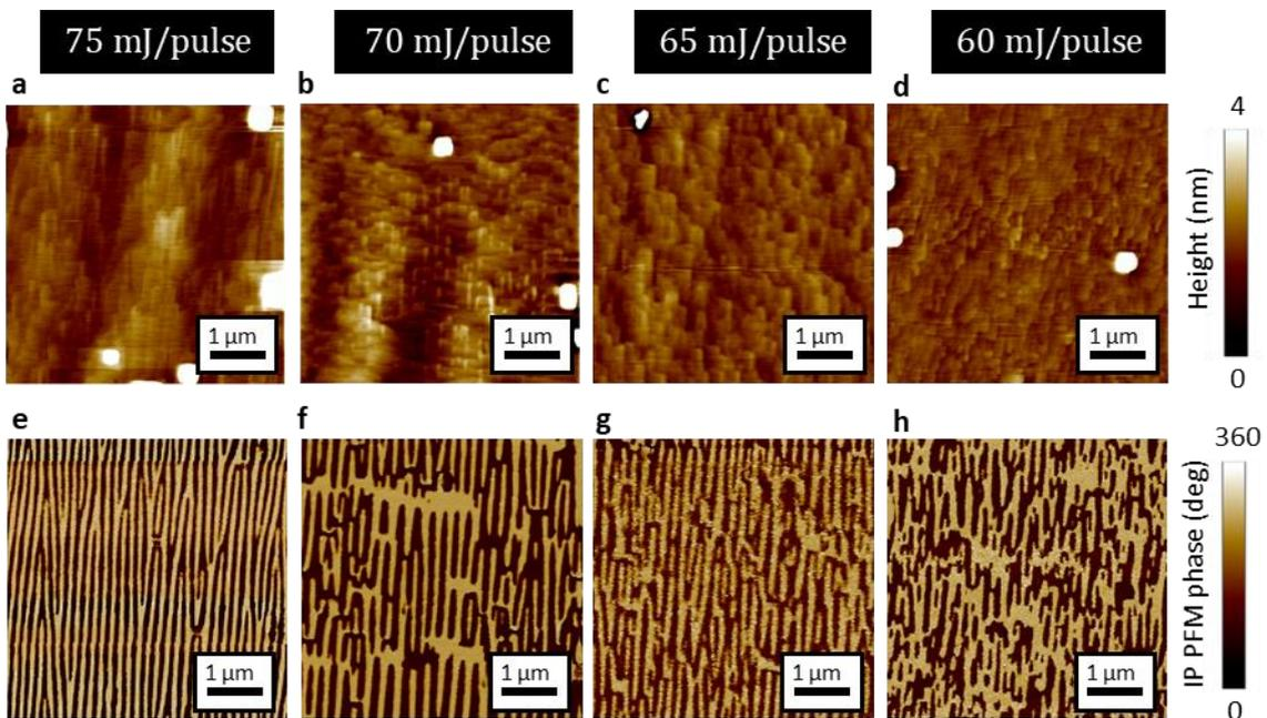
Figure 53:  $\text{BiFeO}_3/\text{SrRuO}_3$  heterostructures deposited on  $\text{DyScO}_3(110)_0$  while decreasing the laser energy per pulse for  $\text{BiFeO}_3$ . **a-e** Topography, **f-j** in-plane PFM phase.
