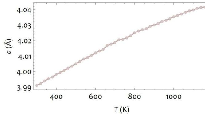
Figure 75 : Out-of-plane lattice parameter vs. temperature of the  $\text{BiFeO}_3$  film on  $\text{DyScO}_3$  extracted from X-ray diffraction measurements up to its decomposition at 1160 K. Adapted from reference [131].
