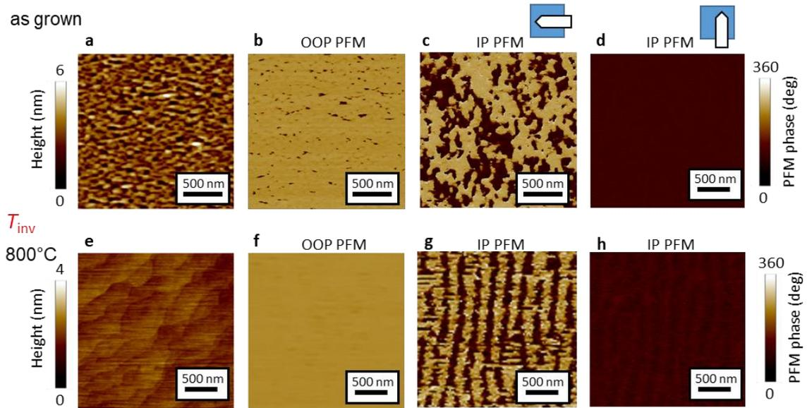
Figure 77 : Transition from a mosaic to a stripe pattern after annealing for one hour at 800°C. **a, e** Topography, **b, f** out-of-plane PFM phase, **c, g** in-plane PFM phase in a first orientation, and **d, h** in-plane PFM phase in a second orientation, as sketched in the upper panel.
