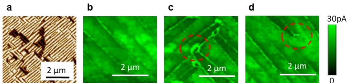
Figure 76 : **a** In-plane PFM image. **b-d** C-AFM images in different zones of **a** to analyse different three-fold junction (**c**) and end-point (**d**) topological defects (red dotted lines) with enhanced conduction compared to the regular ferroelectric domain walls (**b**). Adapted from reference [131].
