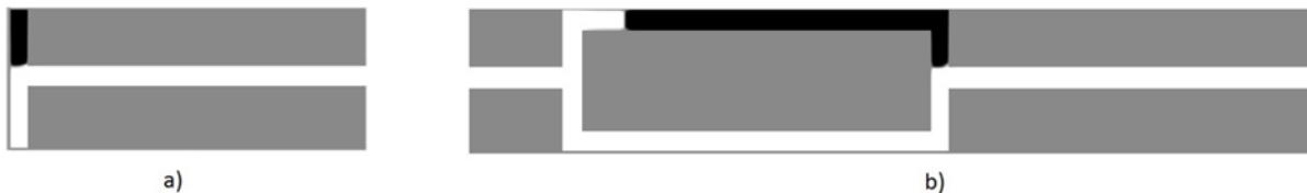
Figure 3.5: a) Standard geometry of the T-junction, b) modified geometry for periodic boundary conditions.
