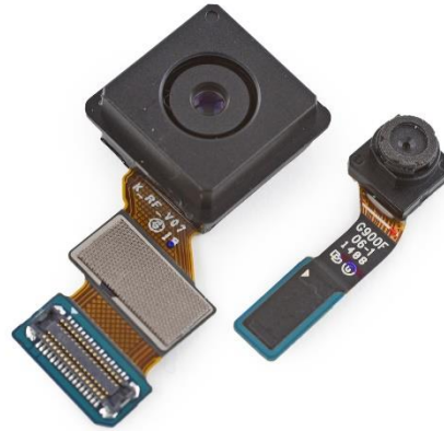
Figure 2-7: Camera module from the Galaxy S5 and a Samsung S5K2P2XX 1/2.6” sensor with an f/2.2 lens [32].
