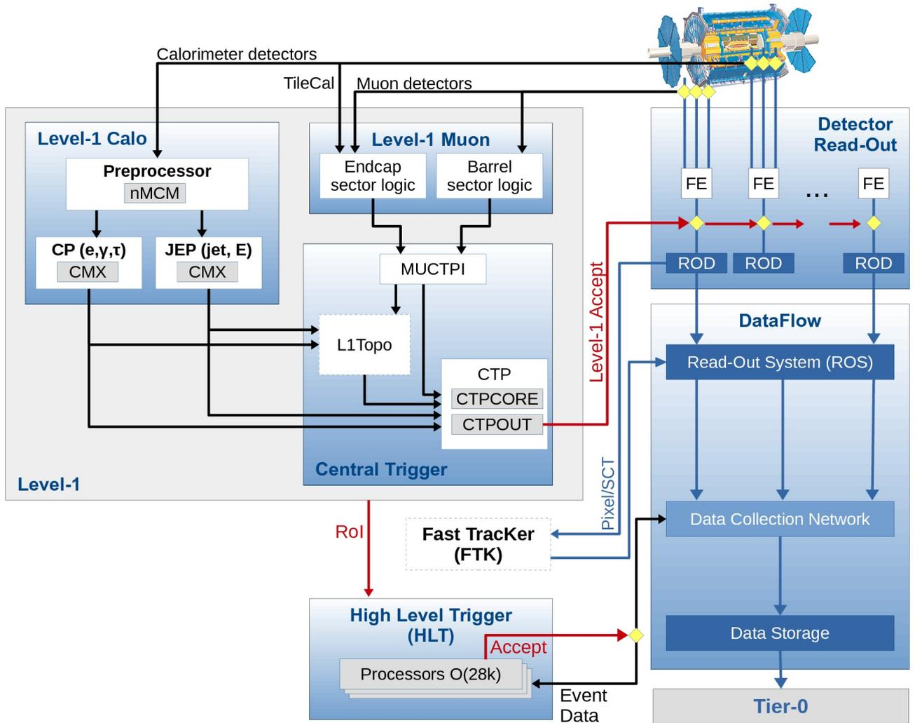
Figure 4.10: The scheme of ATLAS trigger systems
