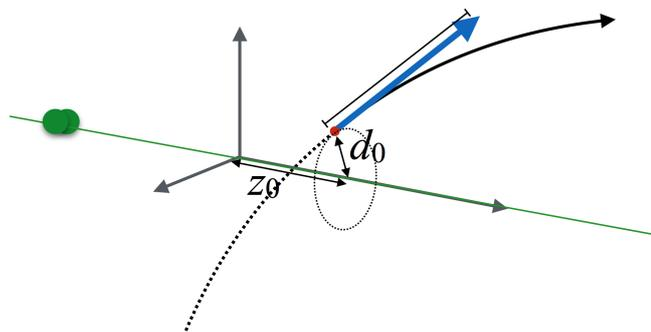
Figure 6.1: Impact parameters  $z_0$  and  $d_0$  [116].
