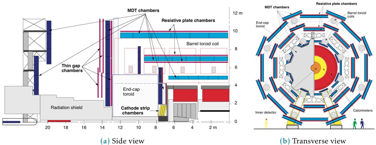
Figure 4.8: Cut views of the muon systems
