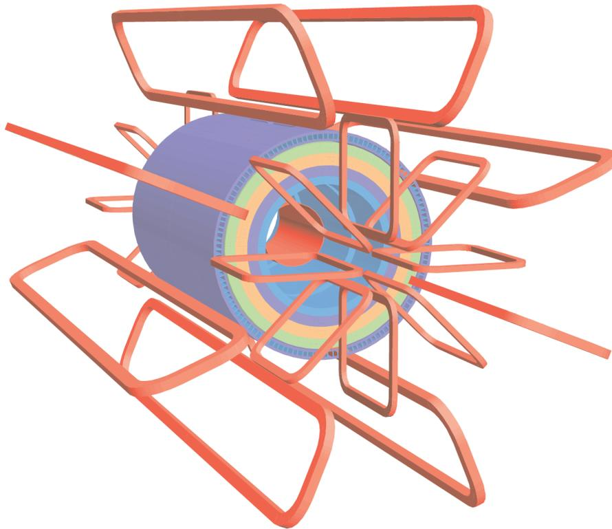
**Figure 4.2:** Geometry of ATLAS magnet windings
