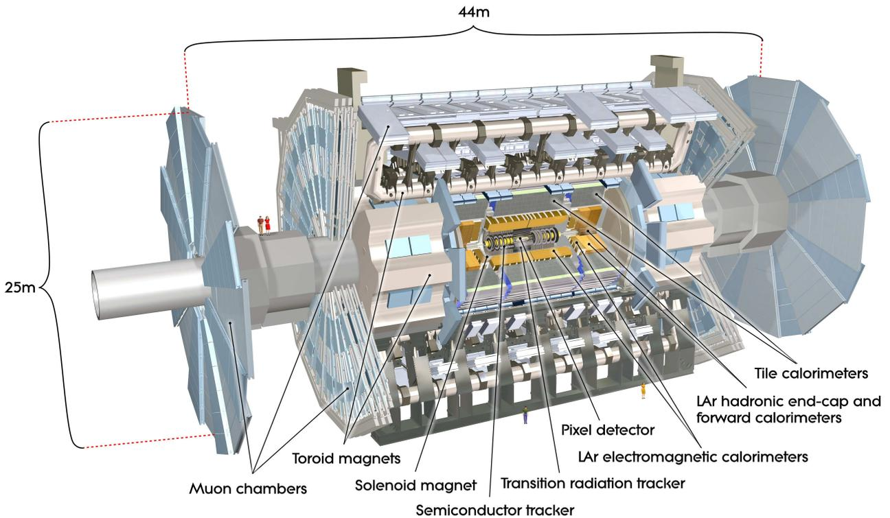
Figure 4.1: ATLAS detector general layout
