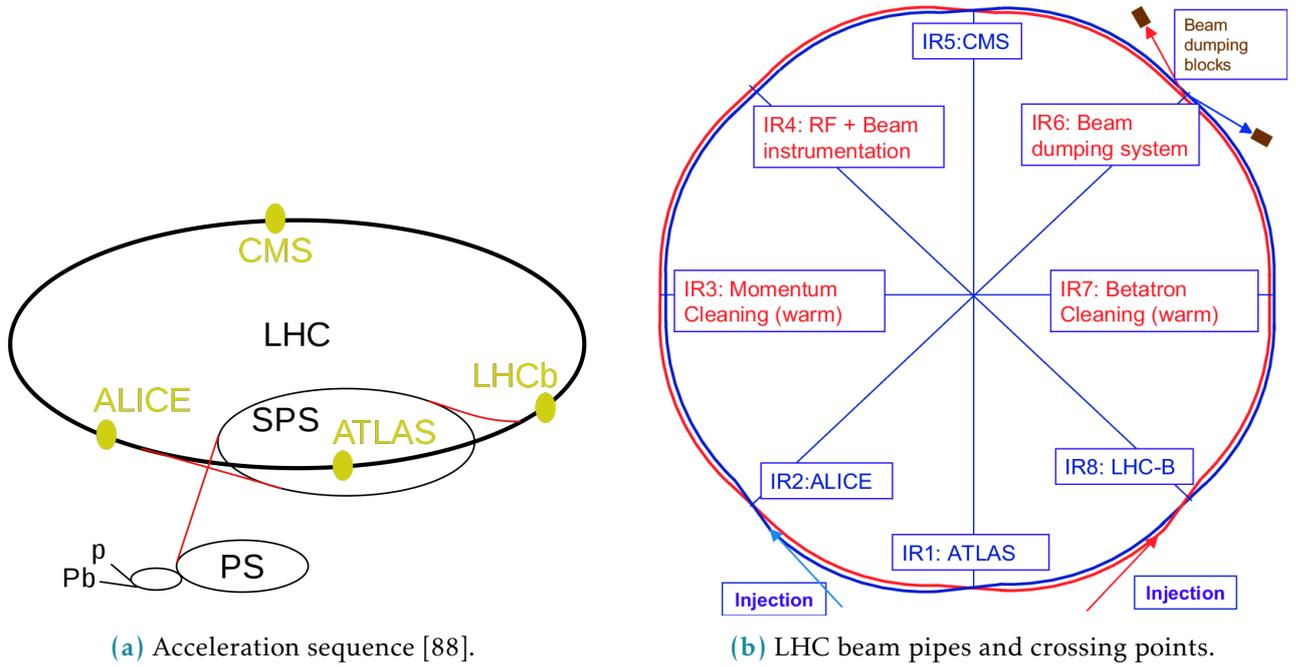
Figure 3.2: Schematic depiction of the LHC ring.
