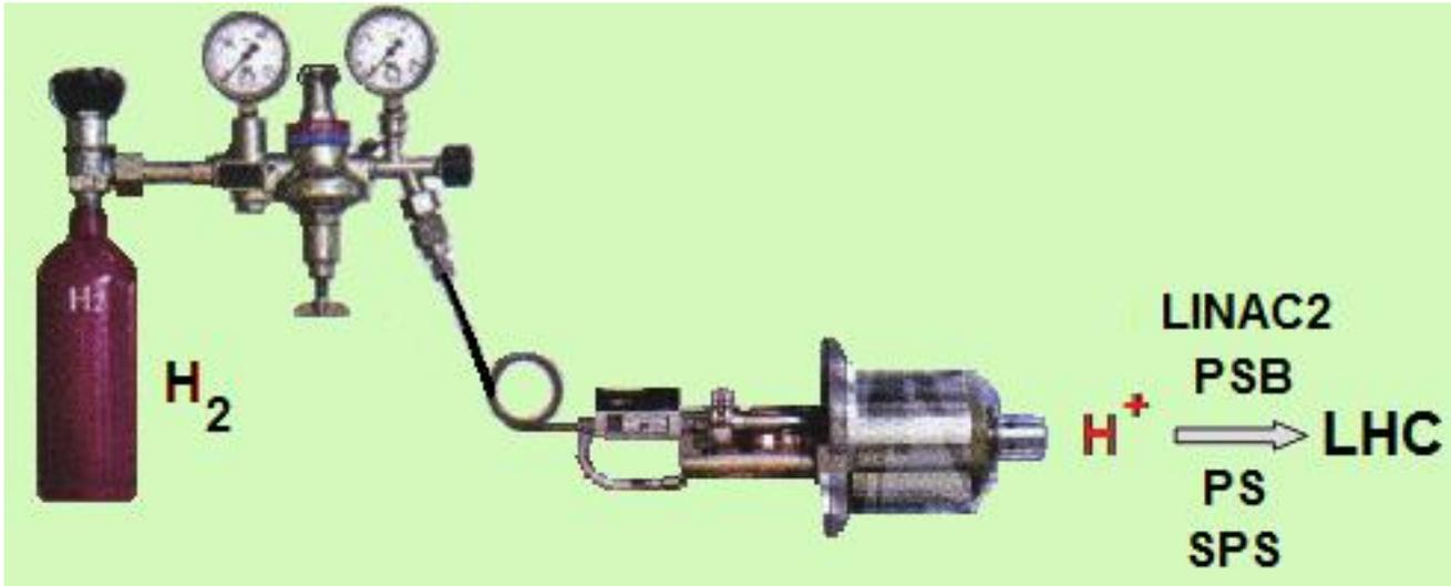
**Figure 3.1:** A hydrogen tank supplies LHC with protons [87].
