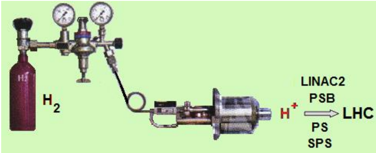
Figure 3.1: A hydrogen tank supplies LHC with protons [87].
