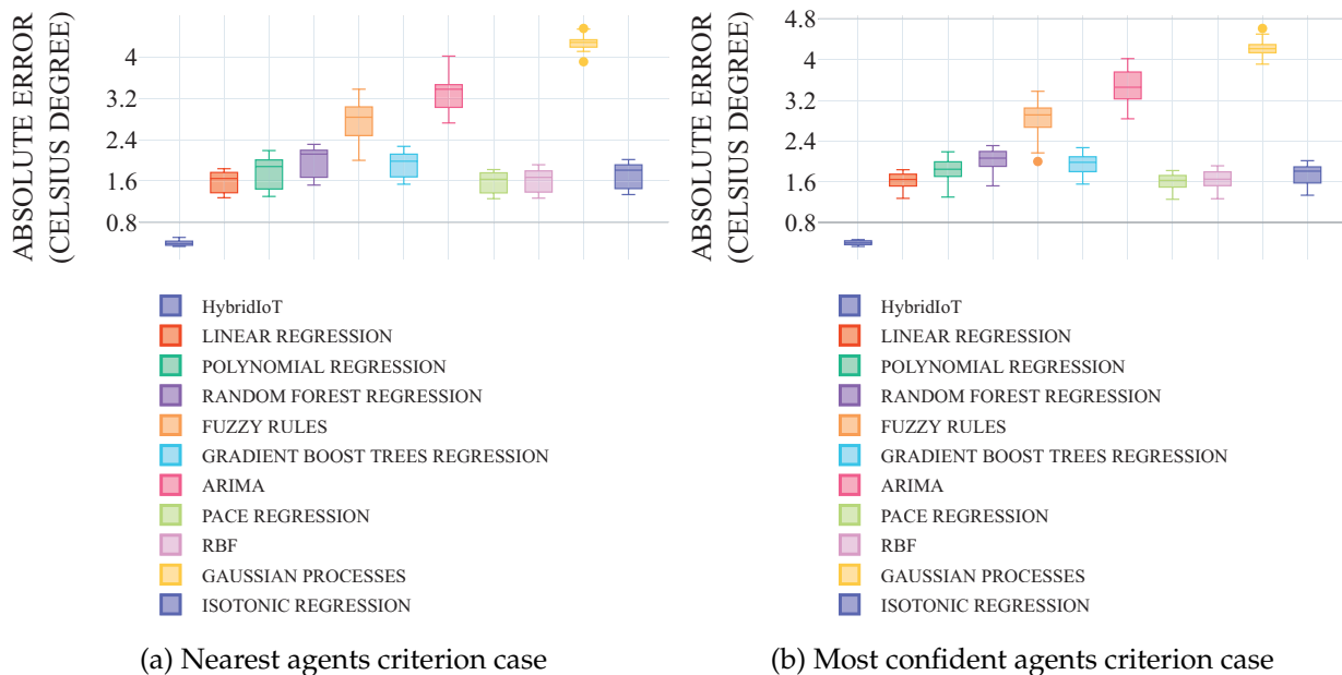
Figure 6.17: Box plot of absolute error (in degree Celsius) obtained by the state of the art techniques on the 15 sensors that gave the worst results using the proposed solution. Figure 6.17a compares the results of the proposed approach using the nearest agents criterion, Figure 6.17b compares the results of the proposed approach using the most confident agents criterion.
