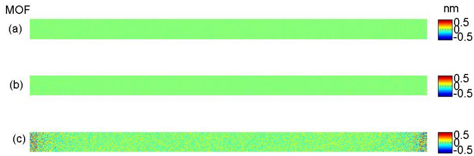
Figure 3.19 : Simulated Fizeau height errors of size 80 x 4 mm 2 , stitched with MOF algorithm with different noise levels; (a) 10x systematic errors, (b) 10x pitch/roll errors and (c) 10x random noise.
