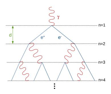
Figure 3.1: Scheme of the first four splits in an EM cascade. Redrawn following [95].
