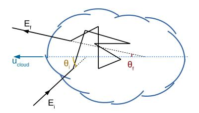
Figure 2.2: Illustration of the second-order Fermi acceleration process.
