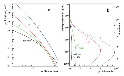
Figure 3.3: Average lateral (a) and longitudinal (b) profiles of vertical showers induced by a proton of energy  $E_0 = 10^{19} \text{ eV}$  simulated with CORSIKA [98]. The number of particles at ground (a) is calculated at depth  $X = 870 \text{ g.cm}^{-2}$  which corresponds to the average ground-level for the Pierre Auger Observatory. From [99].
