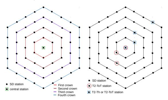
Figure 4.5: Scheme of the SD stations crowns. On the left, the crowns from first to fourth, centered on a central SD station, are represented. On the right, examples of the T3 main trigger geometrical conditions are shown.
