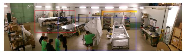
Figure 5.6: Layout of the assembly hall. In the blue rectangle, are the three tables on which the aluminum frames can be put to assemble the detectors. Starting from the right, the second table was used to insert the fibers and make the cookie since it could be tilted via a pressurized air system. In the red rectangle is the testing area, with the test bench at the leftmost table and the table with the computer, DAQ and HV supply beside it.
