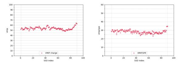
Figure 5.17: Distributions of the SSDs mean VMIP values in pC and VMIP per SPE values by their production number. The mean VMIP values are close to the mean MIP values (see Figure 5.16) but shifted down, as expected since the more vertical muons produce less light as they go through less matter inside the scintillators.
