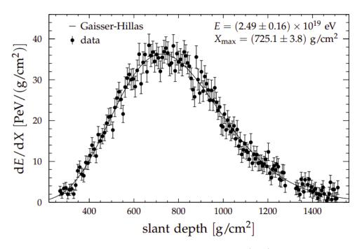
Figure 4.6: Example of a longitudinal profile reconstructed by the FD (dots) as a function of the slant depth in the atmosphere. A Gaisser-Hillas function is fitted to this longitudinal profile to estimate the  $X_{max}$  and the energy of the shower. Taken from [134].
