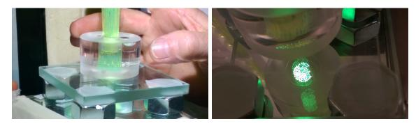
Figure 5.2: Left: Picture of a finished cookie, with the plastic fibers (in green) in place. Right: Picture of the same cookie, taken from above, with a mirror placed below to control the quality of the fibers alignment and gluing.
