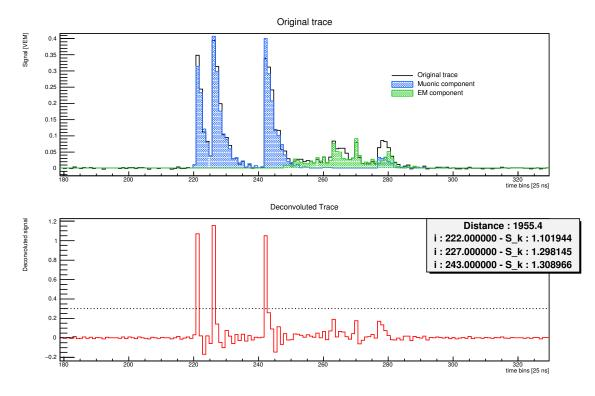
Figure 6.16: The *muonicity* process applied on a simulated VEM trace, with the muonic and EM components highlighted in different colors.
