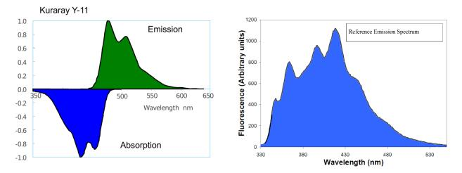
Figure 5.1: Left: Absorption and emission spectrum of the Kurasay Y11(300)M S-type plastic fibers. Right: Reference emission spectrum of the FNAL-NICADD extruded scintillators.
