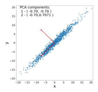
Figure 6.10: A simplified example of a principal component analysis on a 2D gaussian distribution. The blue points are randomnly drawn on a 2D gaussian distribution. The PCA applied on this distribution returns the two axes drawn as red arrows.
