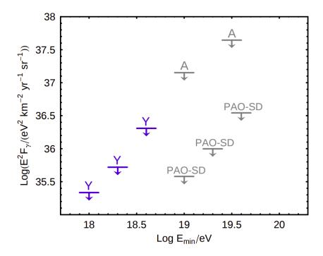
Figure 6.8: Limits (95% CL) on the differential photon flux set by the Yakutsk experiment (Y), the Pierre Auger Observatory (PAO) and the AGASA experiment (A) (results published in 2010). Taken from [191].
