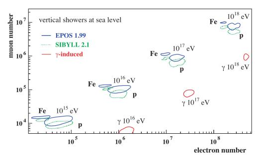
Figure 3.6: Number of electrons and muons on ground (sea-level) predicted for vertical showers initiated by proton, iron and photon primaries with energies  $E_0 = 10^{15} \text{ eV}$ ,  $10^{16} \text{ eV}$ ,  $10^{17} \text{ eV}$ ,  $10^{18} \text{ eV}$  using CORSIKA. From [99].
