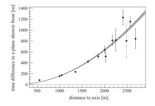
Figure 4.8: Geometrical reconstruction of a shower. As the stations get further away from the core, the time-difference between the expected start time from a planar shower front and the measured one gets larger. From [133].
