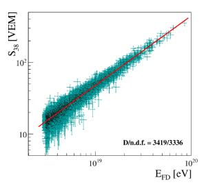
Figure 4.9: Calibration of the SD shower-size estimator  $S_{38}$  using the energy reconstructed by the FD  $E_{FD}$ . The events used to perform the calibration passed very strict quality selection criteria to ensure that the FD energy is reconstructed properly, and that no biases are introduced in the energy of the showers observed by the FD. From [142].
