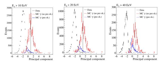
Figure 6.12: The distributions of the projection on the principal component axis of the events above  $E_{\gamma}=10^{19}, 2 \times 10^{19}, 4 \times 10^{19}$  in the Auger-SD photon analysis. In black are the real showers, in red are the MC-photon showers (non-preshowered) and in blue are the preshowered MC-photon showers. Taken from [194]
