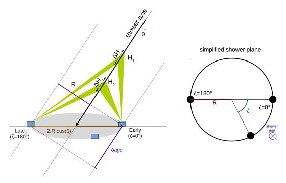
Figure 6.2: Illustrations of the geometry involved in the RiseTime calculations. The secondary particles produced over a given length  $\Delta H$  reach a *late* station with a smaller angle, meaning a shorter time spread than an *early* station located at the same distance r from the shower core.
