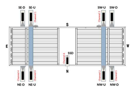
Figure 5.10: Scheme of the setup used to test and characterize the SSDs response at the LPSC. The PMTs on both sides of each scintillator bars making up the external triggers are identified as SE/SW/NE/NW, their localisations on the cardinal axes inside the hall, and -U/-D, whether they are above/below the detectors.
