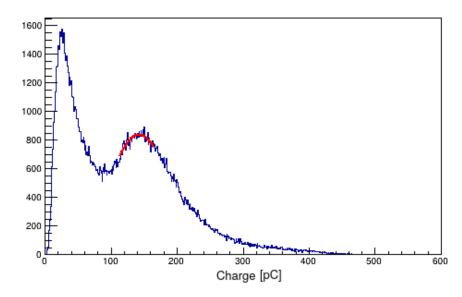
Figure 4.2: Example of a fitted charge histogram. The bin in which the maximum of the peak is reached, around 150 pC, from the fitted part of the histogram, corresponds to the VEM reference.
