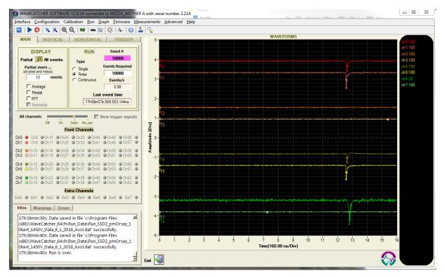
Figure 5.12: A screenshot of the WaveCatcher software, taken during acquisition. This interface allowed us to control that the acquisition was going smoothly and to check for any major lightleaks.
