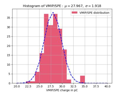
Figure 5.18: Histogram of the mean VMIP/SPE values of the 90 SSDs. The dashed blue line is the fit of the distribution with a gaussian function with parameters  $\mu=27.97$  and  $\sigma=1.92$ .
