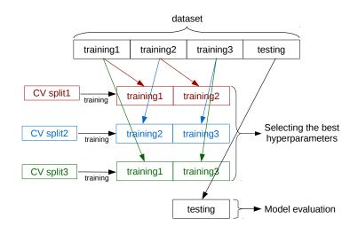
Figure 7.3: Scheme of the cross-validation (CV) process performed on the ML-models to select the best hyperparameters.
