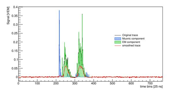
Figure 6.17: The *smoothing* process applied on a simulated VEM trace, with the muonic and EM components highlighted in different colors.
