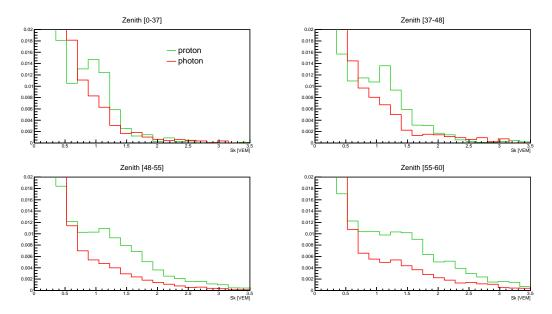
Figure 6.15: Normalized distributions of the  $S_k$  values calculated for MC-protons (in blue) and MC-photons (in red) for showers with  $S_{1000}$  values between 10 VEM and 20 VEM for different ranges of zenith angle.
