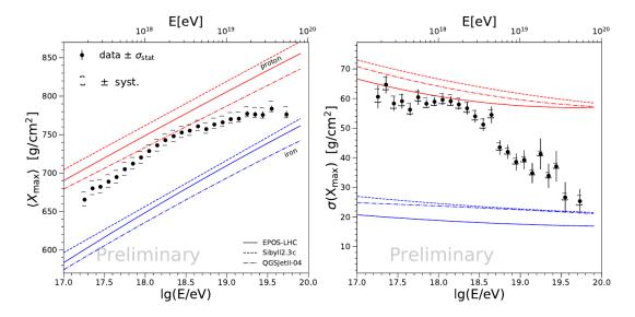
Figure 4.13: Evolution as a function of energy of the primaries mass sensitive observables,  $\langle X_{max} \rangle$  (left) and  $\sigma(X_{max})$  (right). The predictions from proton and iron primaries are represented by red and blue lines respectively, for hadronic models EPOS-LHC, QGSJetII-04 and Sybill 2.3c. From [147]
