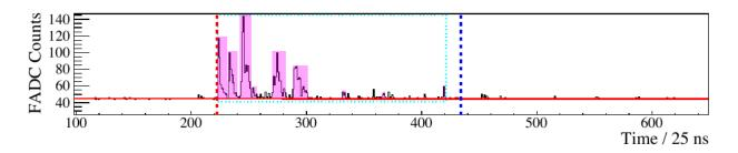
Figure 4.3: Example of a high gain FADC trace from a water cherenkov detector PMT. Signal fragments are highlighted in the purple boxes and the signal merging window is shown as the indigo dashed box. The total signal is the sum of the FADC counts in the bins between the start and stop time represented by the vertical dashed red and blue lines respectively. Taken from [131].
