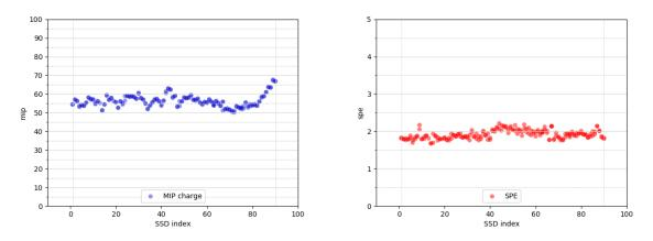
Figure 5.16: Distributions of the SSDs mean MIP and SPE values in pC by their production number. The values themselves are within the specifications set by the collaboration around 55 pC and 1.9 pC respectively. The stability of the values through the construction is also satisfactory, although we observed an increase in the mean MIP values on the last few SSDs tested.
