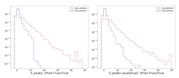
Figure 7.6: Normalized distributions of the relative error of  $S_{peaks}$  for protons (blue) and photons (red). Left: ML models. Right: Analytical models.
