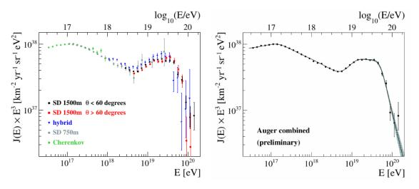
Figure 4.12: Energy spectra measured by the Pierre Auger Observatory (left) and the corresponding combined spectrum fit (right). From [142]
