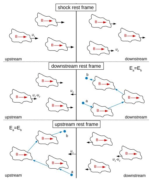
Figure 2.3: Illustration of the first-order Fermi acceleration mechanism.
