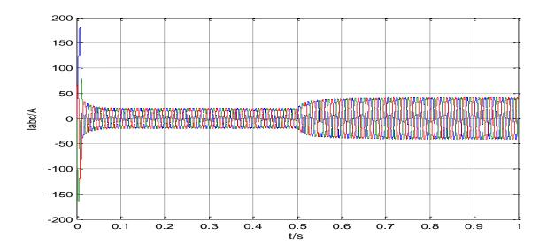
Fig.3. 24: The grid side current during load fluctuation.
