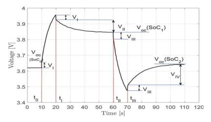
Fig 4.3: Battery voltage during charging and discharging.
