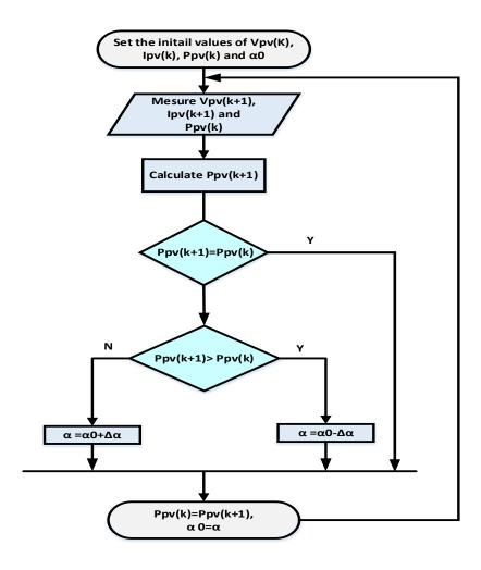
Fig 3. 3: Flow chart for the MPPT control.
