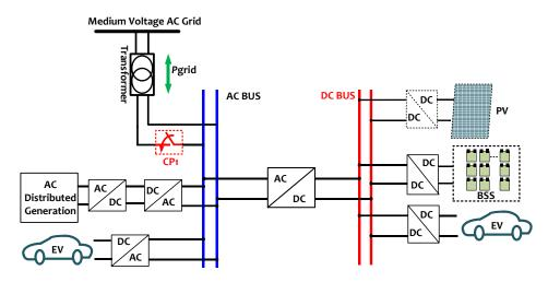
Fig 2. 10: Topology of AC-DC hybrid micro-grid structure.
