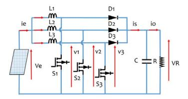
Fig 3. 4: Interleaved (DC/DC) Converter.
