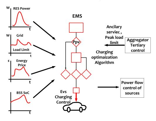
Fig 2. 12: EMS structure for EV charging station.
