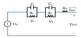
Fig 4.1: Schematic diagram for the DP model.
