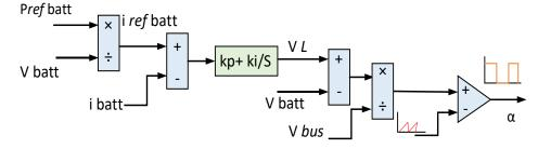
Fig 3. 16b: Controller scheme of IBDC.
