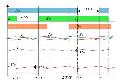
Fig 3. 13: Switches conduction timeline, case 3.
