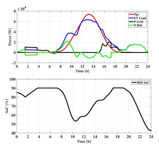
Fig 4.7 B: Power flow of charging system components and BSS SoC 85 % on clear day.
