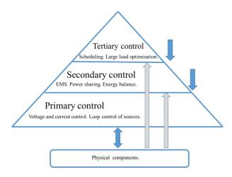
Fig 2. 11: Hierarchical control of EV charging stations.
