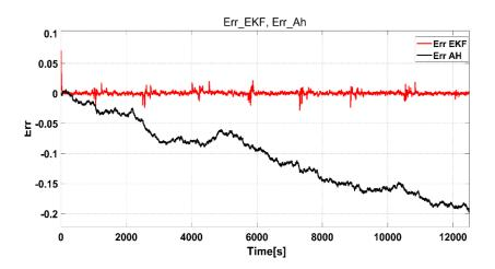
Fig 4.11: EKF SoC estimation 90-20% and SoC estimation Error.
