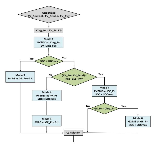
Fig 5.4: Operation at underload situation.
