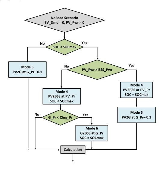
Fig 5.5: Operation at underload situation.
