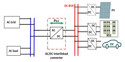
Fig 3. 8: AC/DC micro-grid with DC charging station.
