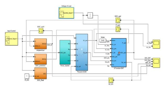
Fig 4.8: Simulink model of ECM and EKF.
