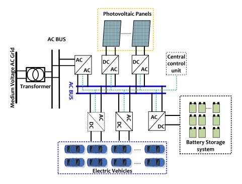
Fig 2. 8: AC micro-grid structure with EVs chargers.
