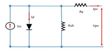
Fig 3. 6: Equivalent circuit model PV panel.
