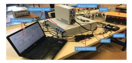
Fig 4.2: Battery test bench.
