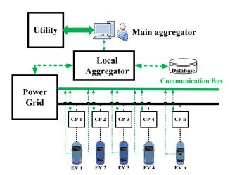
Fig 2. 13: Centralized control architecture.
