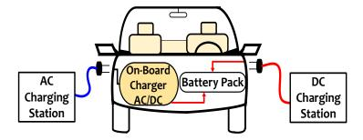
Fig. 1. 3: On-board and off-board of EV chargers.
