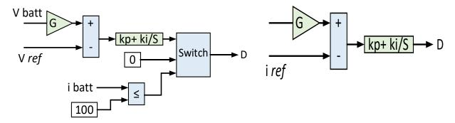
Fig3.18: PI controller scheme of EV c charger.
