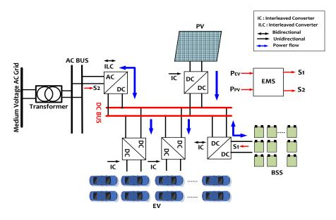
Fig 5. 3: General system structure and EMS of the EV charging station.
