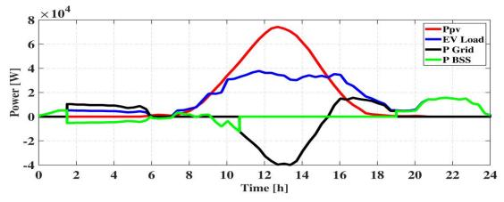
Fig5.8: PV energy to grid in case of SoC high and low EVs load.
