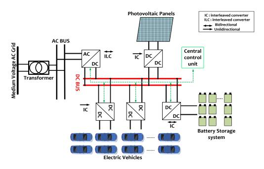
Fig 3. 5: EV charging station module based on DC micro-grid.
