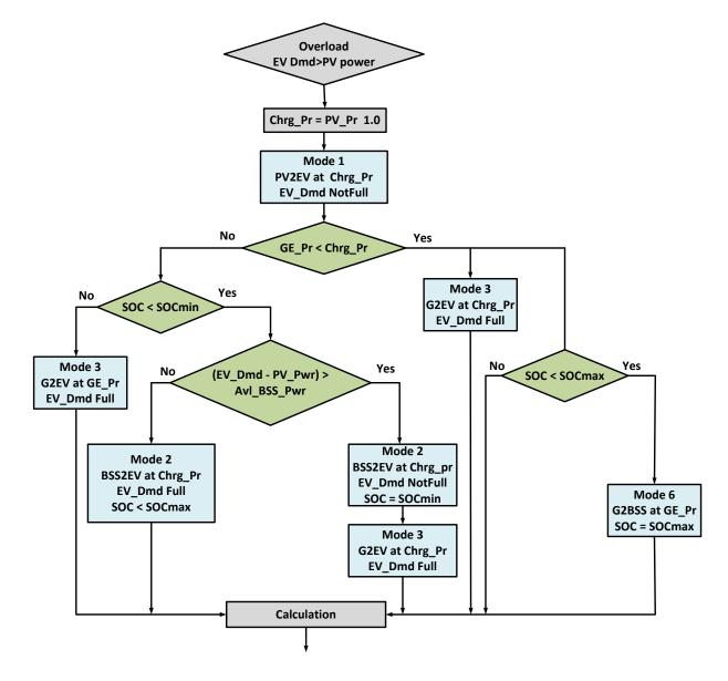
Fig 5.3: Operation at overload situation.
