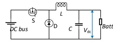
Fig 3.17: buck DC/DC converter.
