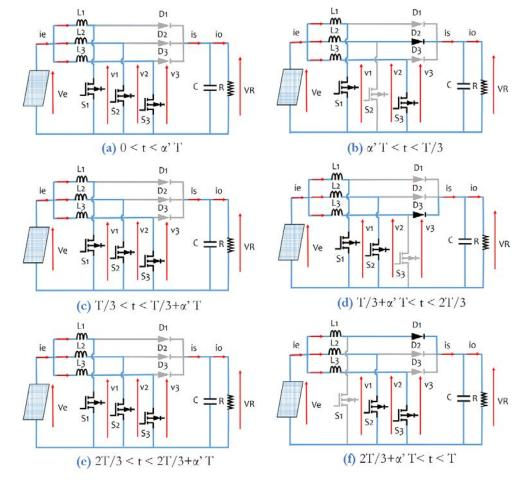
Fig 3.12: Behavior of interleaved converter in each small interval for case 3.
