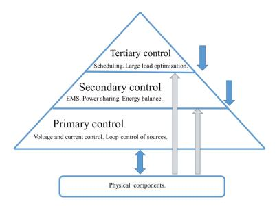
Fig 1. 5: Hierarchical control of EV charging station
