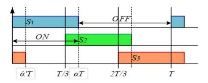
Fig 3. 8: Switches conduction timeline, case 2.
