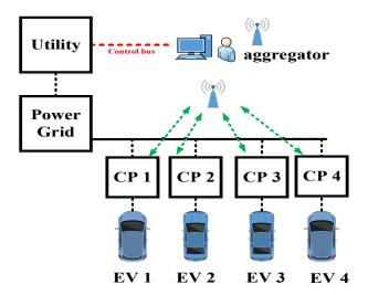
Fig 2. 14: Decentralized control architecture.
