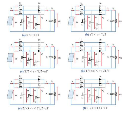
Fig 3. 9: Behavior of interleaved converter in each small interval case 2.
