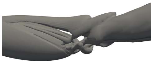
Fig. 10 Detail of the vortical structures in the wake of the prolate spheroid for the unsteady simulation at AoA = 35^\circ .
