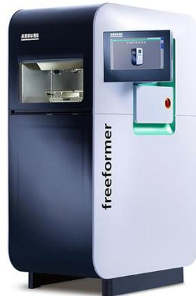
Figure II-4 : Freeformer machine
