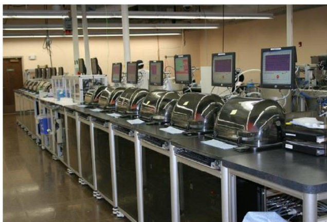
Figure IDT's patented X96 synthesis platform with increased environmental control achieves higher coupling efficiencies. As a result, oligos with more full-length product and longer oligos (up to 200 bases) are obtained.
