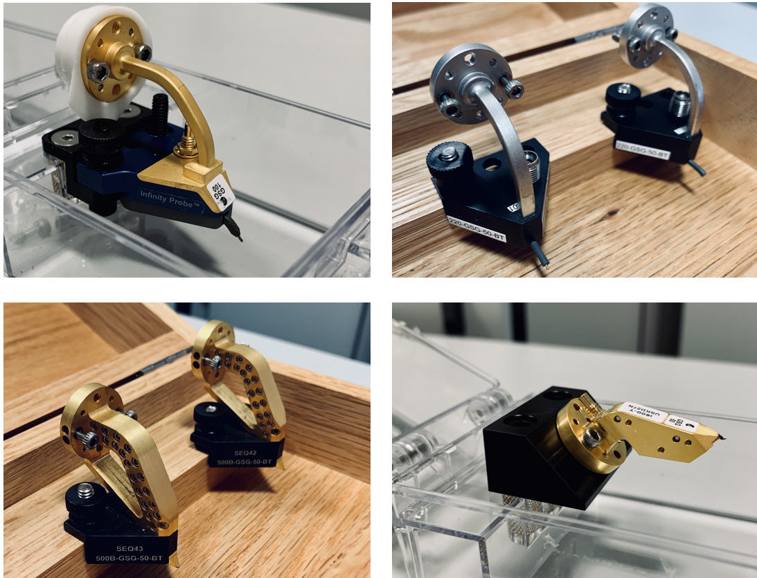
Figure 2.12: Pictures of the used probes for millimeter wave measurements. From top left to bottom right: IP-220, PP-220, PP-500, TW-500.
