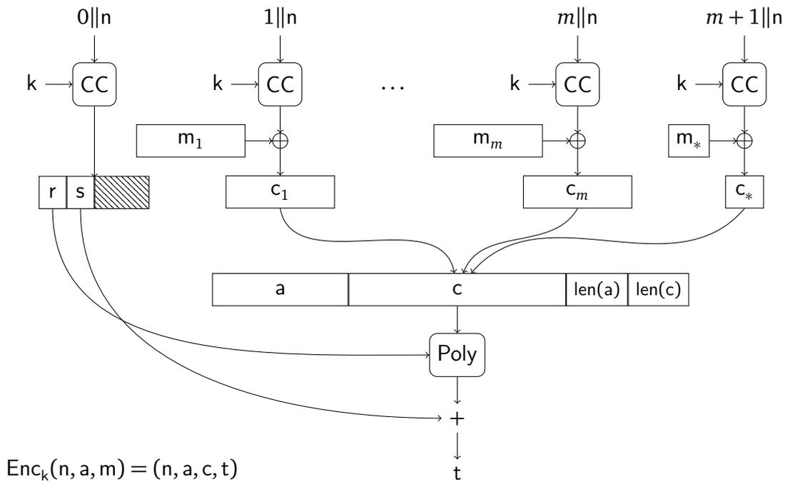
Figure 8.1 – Representation of the encryption algorithm of ChaCha20-Poly1305.
