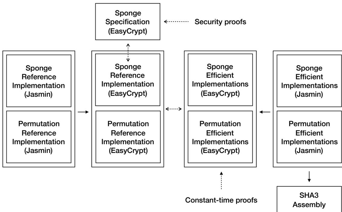
Figure 6.1 – Our results. Full lines represent extraction to EasyCrypt and compilation to assembly by the Jasmin compiler. Dashed lines represent equivalence and security proofs, formalized in EasyCrypt.
