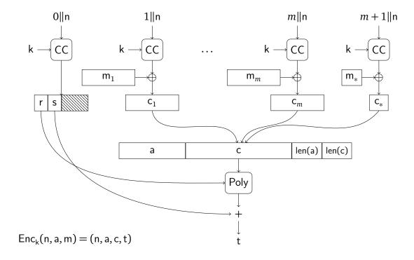
Figure 8.1 – Representation of the encryption algorithm of ChaCha20-Poly1305.
