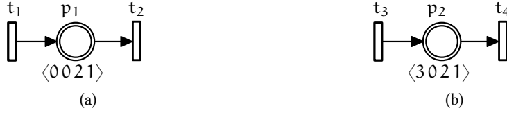
Figure 6.7. – In (a) \mathcal{H}_1 = \langle 0 \ 0 \ 2 \ 1 \rangle satisfies the FIFO condition. In (b) \mathcal{H}_2 = \langle 3 \ 0 \ 2 \ 1 \rangle violates the FIFO condition.
