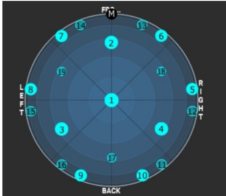
FIGURE F.5 – Visualization of the microphone capsules placement using IEM MultiEncoder.
