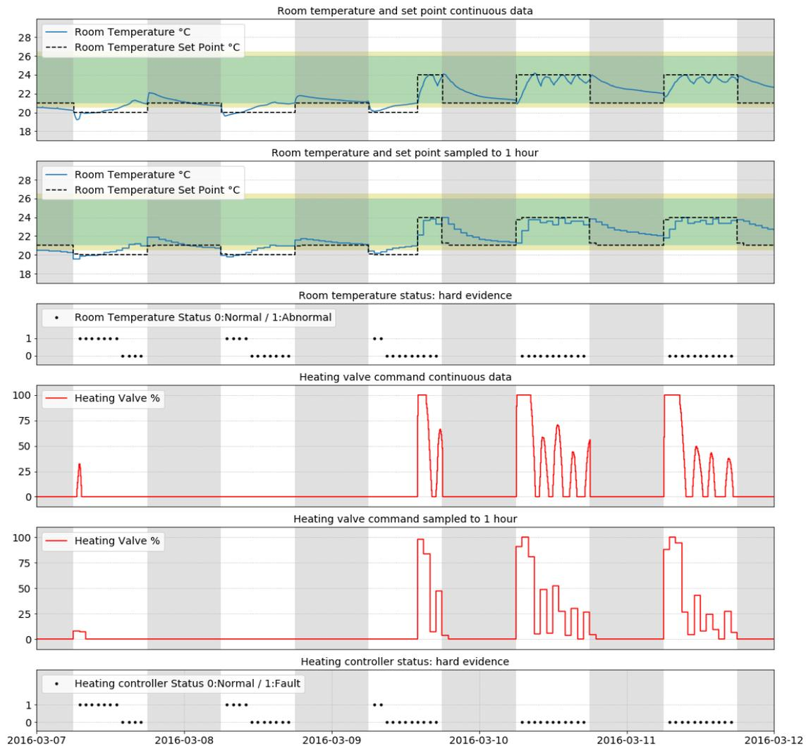
Figure 3.29 – Controller hard evidence: Porte de Retz building FCU28 heating control
