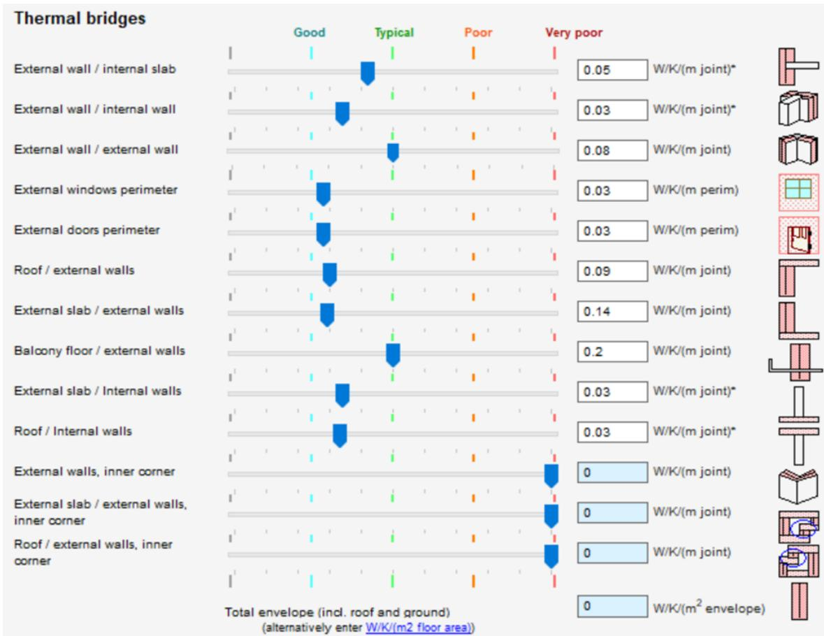
Figure A.3 – Parameters of thermal bridges in Green O Valley building
