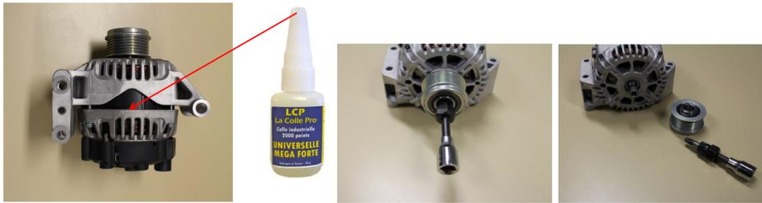
Figure 5.11: Claw-pole machine disassembling
