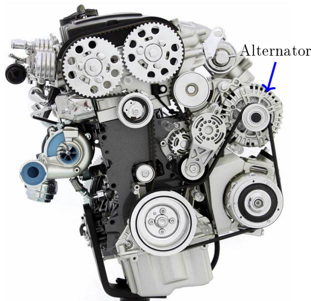
Figure 5.1: Position of claw-pole alternator
