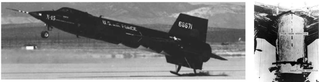
Figure 1.1: An example of aerodynamic heating due to SWBLI. X-15 hypersonic test airplane (left) and Damage in X-15 hypersonic airplane (right). From [8].
