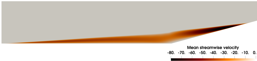
Figure 5.12: SingleRamp: Negative-value contours of the mean streamwise velocity around the separation bubble.
