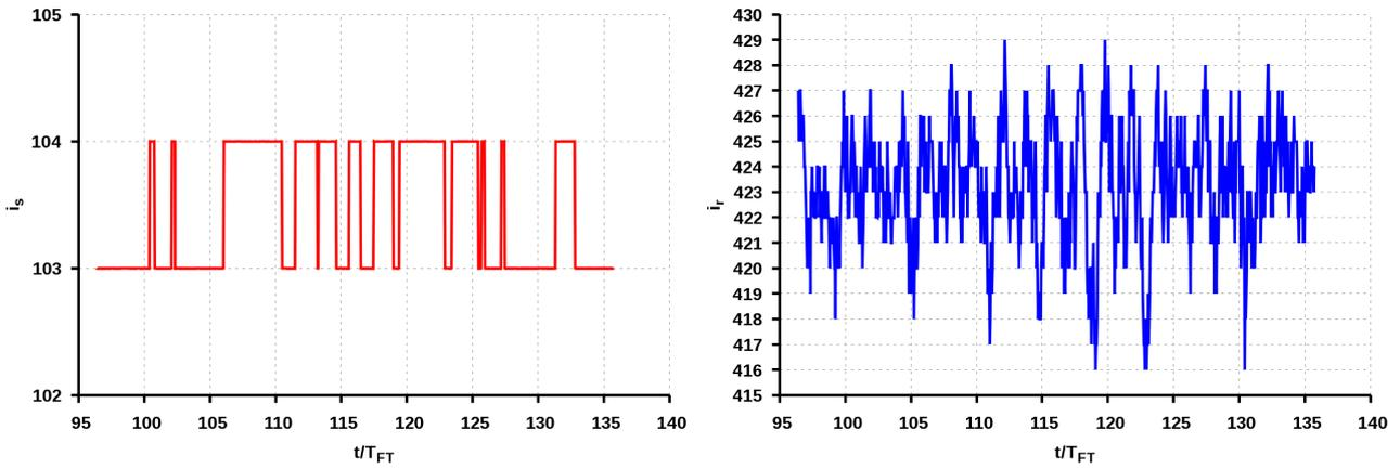
Figure 5.14: SingleRamp: Time evolution of the separation point (left) and reattachment point (right).  $i_s$  and  $i_r$  are the cell indexes at which the separation and reattachment occur, respectively.
