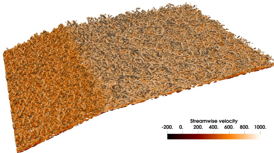
Figure 5.18: CompExp: Vortical structures evidenced by the Q-criterion, coloured by the streamwise velocity. Zoom on the expansion corner.
