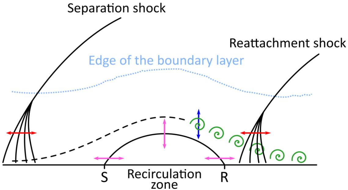
Figure 5.1: Sketch of the separation bubble for compressible flows. The four main unsteady phenomena are highlighted: *shedding* (green), *flapping* (blue), *breathing* (pink) and oscillations of the shock system, known as the unsteadiness of the RB (red). Adapted from [115].
