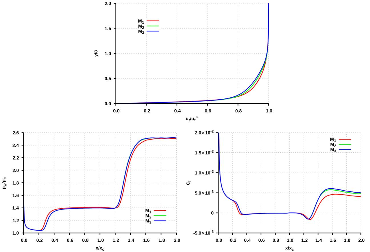
Figure 5.2: SingleRamp: Wall-normal profile of the tangential velocity  $u_t$  at  $x = 8.4 \text{ mm}$  (top), Streamwise evolution of the spanwise-averaged wall-pressure (bottom-left) and friction coefficient (bottom-right) for three different meshes.
