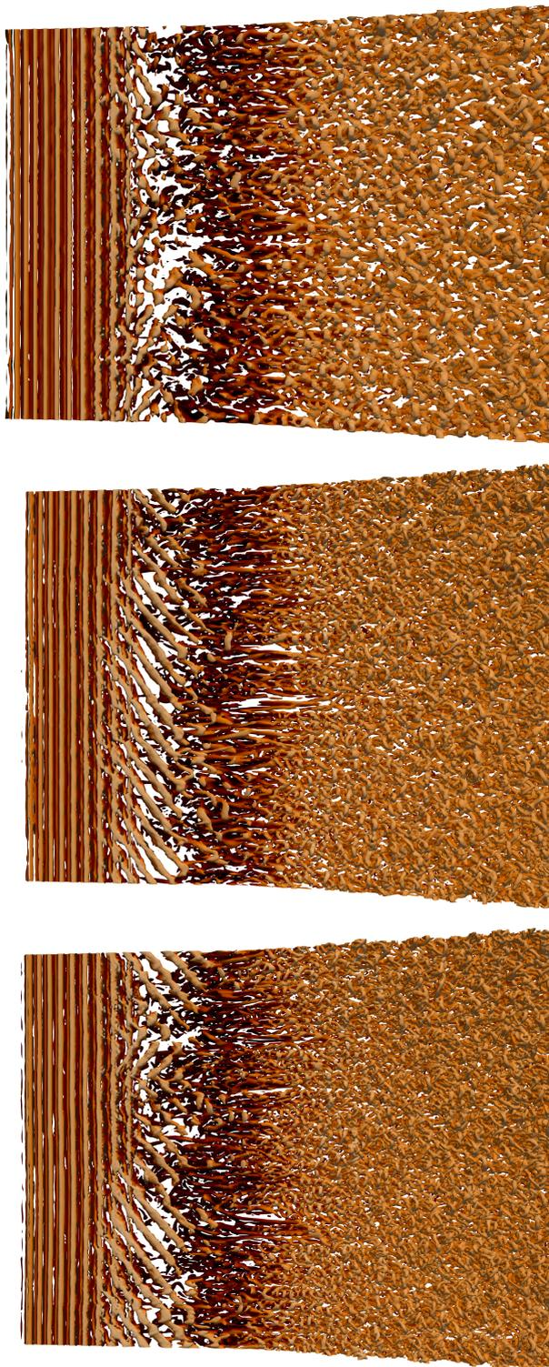
Figure 5.8: SingleRamp: Top view of the vortical structures obtained with three different meshes. Top:  $M_1$ , Middle:  $M_2$  and Bottom:  $M_3$ . It is noteworthy that the transition occurs slightly earlier for  $M_1$  than for the other two meshes.
