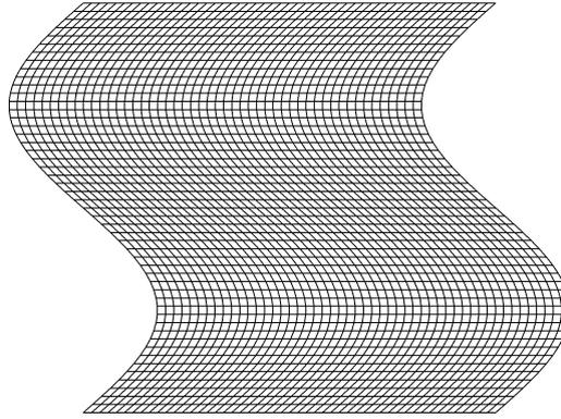
Figure 2.4: Example of a 2D-Sine-Distorted Mesh with  $A = 0.18$ .
