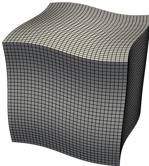
Figure 2.5: Example of a 3D-Sine-Distorted Mesh with  $A = 0.18$ .
