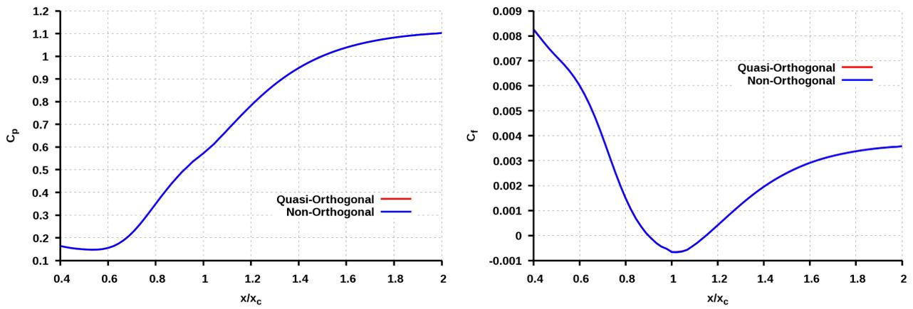
Figure 4.14: Streamwise evolutions of the pressure (left) and skin-friction (right) coefficients for the non-orthogonal and quasi-orthogonal meshes in the Carter test-case configuration.
