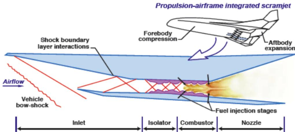
Figure 2: Flow-field characteristics of scramjet engine [145].
