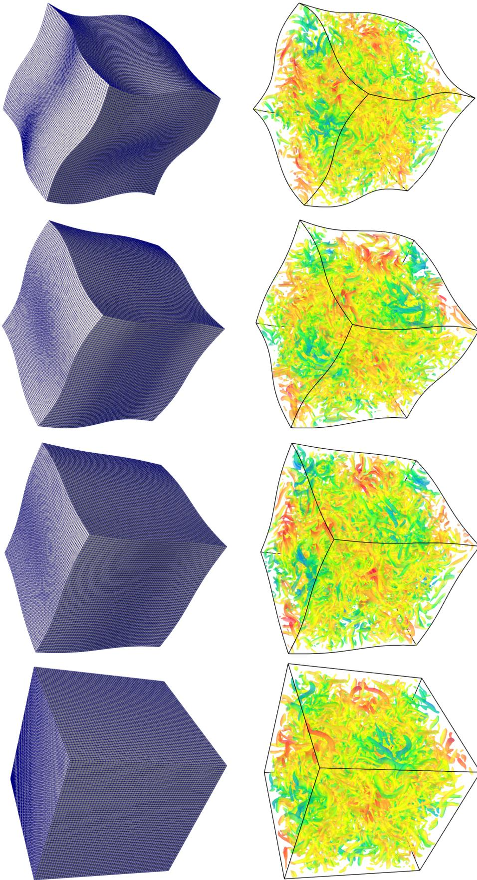
Figure 3.22: Mesh (top) and Isosurfaces of the Q-criterion coloured by the x-component of velocity at  $t = 20$  (bottom) for four different meshes. From left to right: Cartesian mesh,  $A = 0.09$ ,  $A = 0.18$  and  $A = 0.30$ .
