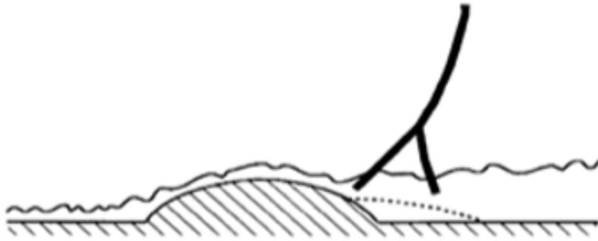
Figure 1.5: Transonic flow over a bump. From [96].
