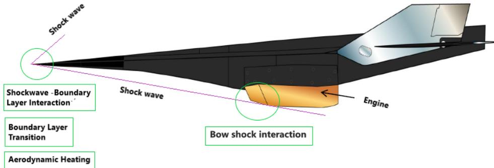
Figure 1: The aerodynamics environment of a supersonic/hypersonic aircraft.
