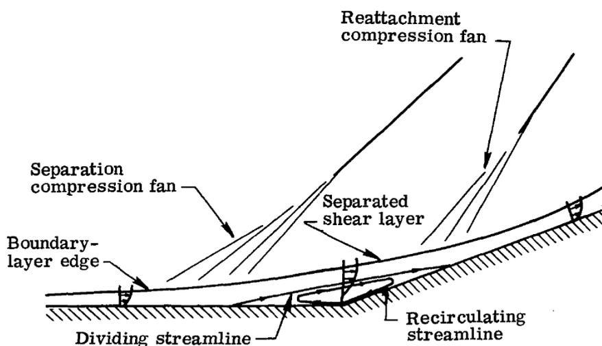
Figure 1.6: Supersonic flow over a compression ramp. From [28].
