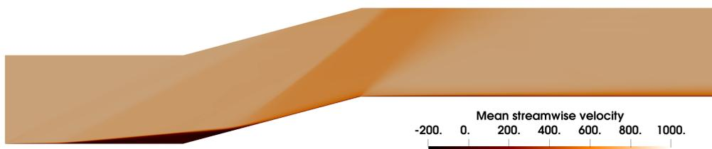
Figure 5.19: CompExp: Time- and spanwise-averaged streamwise velocity contours.
