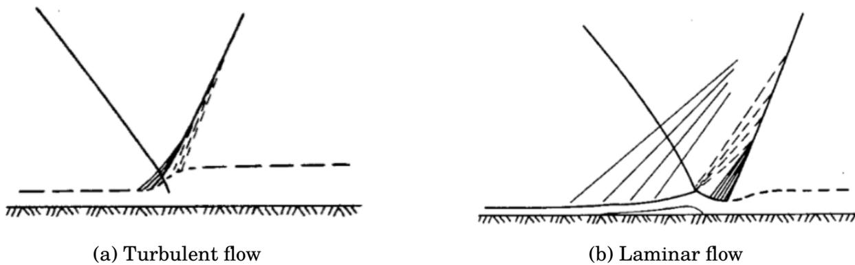
Figure 1.9: Reflected shock pattern. From [102].
