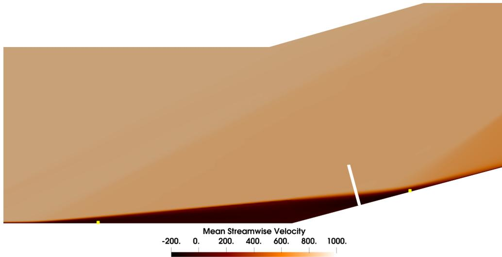
Figure 5.3: SingleRamp: Time- and spanwise-averaged streamwise velocity field showing the extraction line (white) for the  $\overline{u_i' u_j'}$  profiles. The two yellow points are the location for the probes used in section 5.2.3.3.
