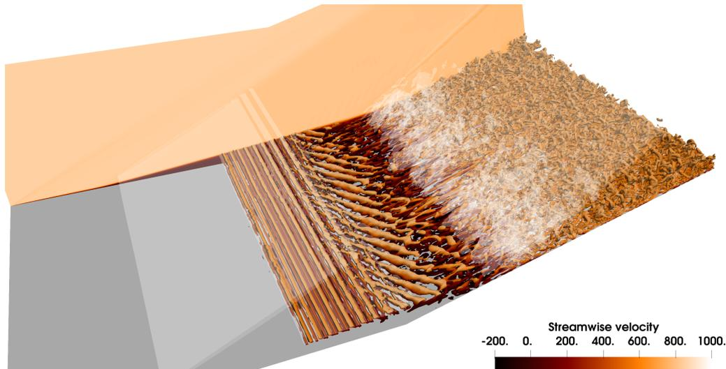
Figure 5.5: SingleRamp: Vortical structures evidenced by the Q-criterion, coloured by the streamwise velocity. The shock system is highlighted by isosurfaces of  $div \mathbf{u}$ .
