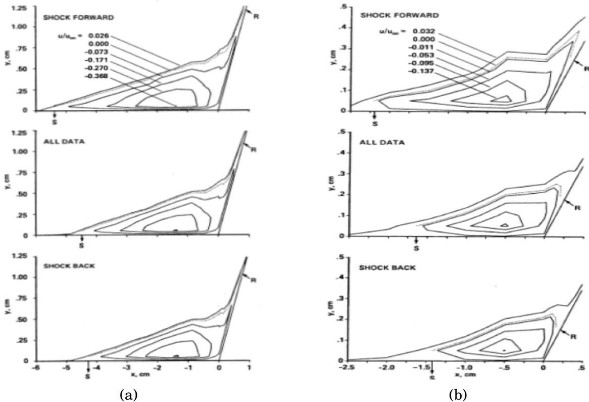
Figure 1.16: The contours of the mean velocity at two different shock angle  $23^\circ$  (a) and  $5^\circ$  (b). From [94].
