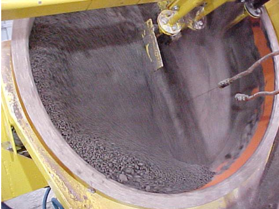
Fig. 2.2: Disc pelletizer (Mars Mineral, 2020). The particles are agglomerated together thanks to their collision, if they do not rebound from each other.
