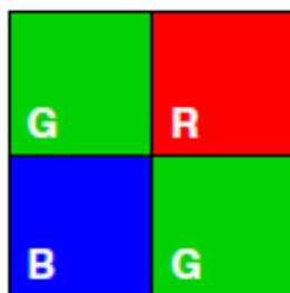
Figure 3.1: Bayer pattern that can be used in color cameras
