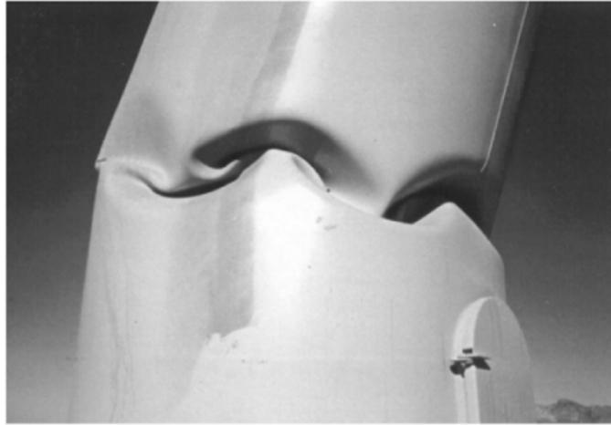
Figure 2.4: Example of wind turbine tower failing by buckling. [Jay et al., 2016]
