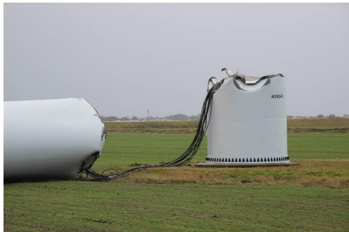
Figure 1.12: Collapsed wind turbine in Bouin, France [Parisien, 2018].
