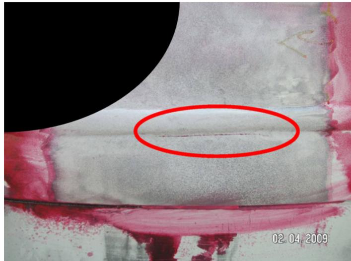
Figure 1.9: Photo of a crack in a weld [Lacalle et al., 2011].
