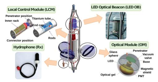
Figure 2.4: The schema of an storey with the three OMs (in purple), the LCM (grey cylinder in the center) and some equipment for the calibration: the hydrophones (orange, bottom left) for the positioning and the LED Optical Beacons (blue capsule on top) for time calibration and monitoring of the water properties.
