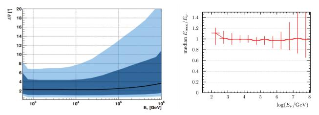
Figure 3.2: Left: Median angular resolution as a function of the neutrino energy for cascade events with ANTARES. The 68% and 98% CL contours are indicated in dark and light blue, correspondingly. Right: Median value of the ratio between the reconstructed shower energy and the true neutrino energy. The error bars indicate the 68% uncertainties for shower events with ANTARES.
