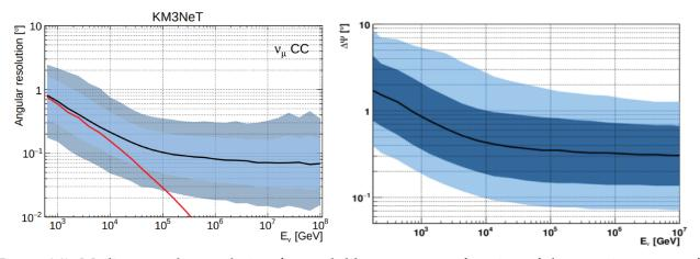
Figure 3.5: Median angular resolution for track-like events as a function of the neutrino energy for ANTARES (left) and full ARCA (right) detectors. The improvement achieved with ARCA is notable for pointing to neutrino sources.
