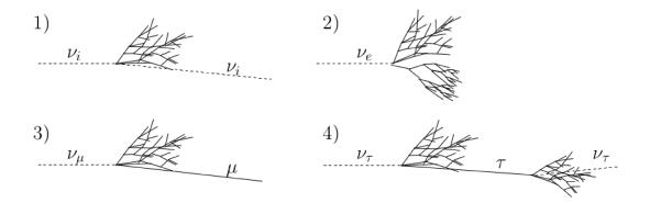
Figure 2.2: Signatures of the event topologies observed for different types of neutrino interactions. 1) NC interaction producing only a hadronic shower. 2) CC interaction of a  $v_e$ , initiating an EM and an hadronic shower. 3) CC interaction of a  $v_{\mu}$  producing a long muon track with an hadronic shower. 4) CC interaction of a  $v_{\tau}$ , generating a  $\tau$  that decays producing the double-bang signature.
