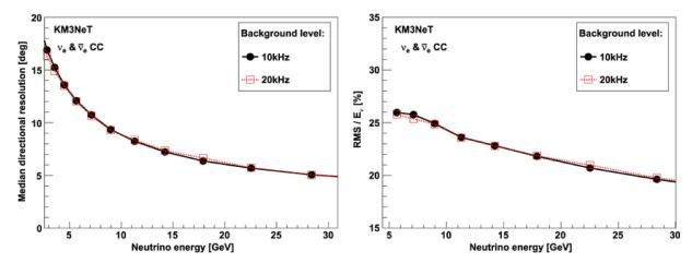
Figure 3.3: Left: Median angular resolution as a function of the neutrino energy for cascade events with the full ORCA detector. Right: Relative energy resolution for shower events with ORCA. The resolution estimates are done for two different background levels considered (black and red).
