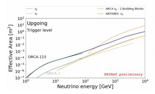
Figure 3.6: Trigger level effective area for upgoing neutrino events for the ANTARES and KM3NeT detectors. For the ORCA detector, 115 and 7 DUs configurations are considered, as well as both  $v_e$  and  $v_{\mu}$ . For ARCA and ANTARES, it is shown only for  $v_{\mu}$ .
