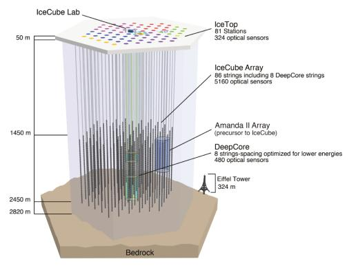
Figure 2.9: Schematic view of the IceCube Neutrino Observatory with the IceTop array and DeepCore. For comparison, the AMANDA detector is illustrated.
