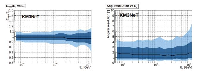
Figure 3.4: Left: Median angular resolution as a function of the neutrino energy for cascade events with the full ARCA detector. Right: Median energy resolution for shower events with ARCA. The 68% and 98% CL contours are indicated in dark and light blue, correspondingly.
