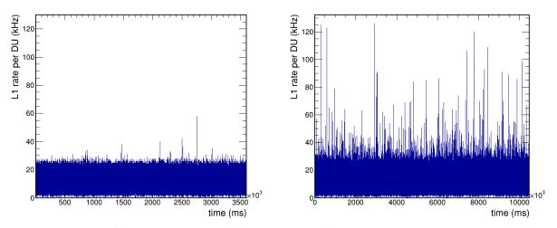
Figure 5.7: Example of background lightcurves measured from raw data, sampled with a 1 ms binning. On the left for ARCA, on the right for ORCA. They are generated with a selection of 5 ns L1 coincidences. The spikes observed in ORCA data (not observed in ARCA due its deeper location and the larger distance between the DOMs, which prevent to detect such coincidences) are correlated at sub-ms scale and thus may be induced by correlated muon coincidences.
