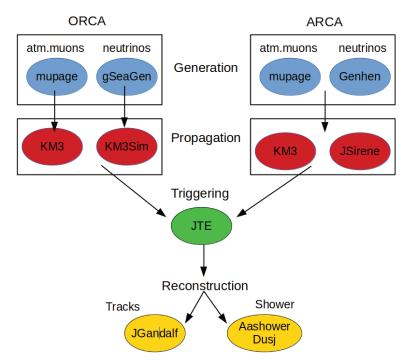
Figure 3.1: A schematic view of the software chain used in the KM3NeT detectors, going from the simulation to the physics trigger and reconstruction.
