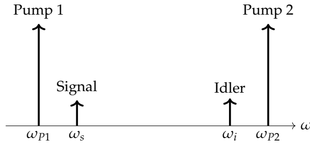
Figure 2.1. General configuration of a FOPA without considering any sidebands. \omega_s , \omega_i , \omega_{p1} and \omega_{p2} are the frequencies of the signal, idler, pump 1 and pump 2 waves respectively. The height of the arrows represent intensity of the waves (not to scale).
