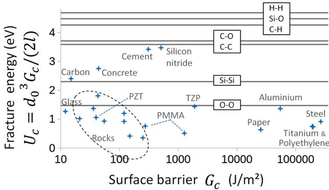
FIG. 4. Microscopic fracture energy  $U_c = d_0^3 G_c / (2l)$  as a function of the macroscopic energy barrier  $G_c$ , for the same materials as Fig. 3. See the supplementary material for the exhaustive list. Note that the accuracy of  $U_c$  is not better than an order of magnitude. The horizontal lines show some typical covalent cohesion energies for comparison [35].
