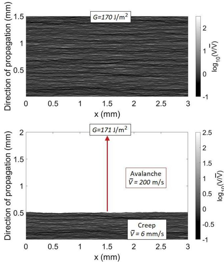
FIG. 2. Spatial crack velocity map for a mean energy release rate of  $170\text{J m}^{-2}$  (top) and  $171\text{J m}^{-2}$  (bottom), with the parameters described in section II. In the latter case, a thermal avalanche is triggered (white area, with an average velocity of  $200\text{m s}^{-1}$ ). The mean velocity defining the colour scale is that of the creep (slow) phase, without an avalanche:  $\bar{V} = 6\text{mm s}^{-1}$ .
