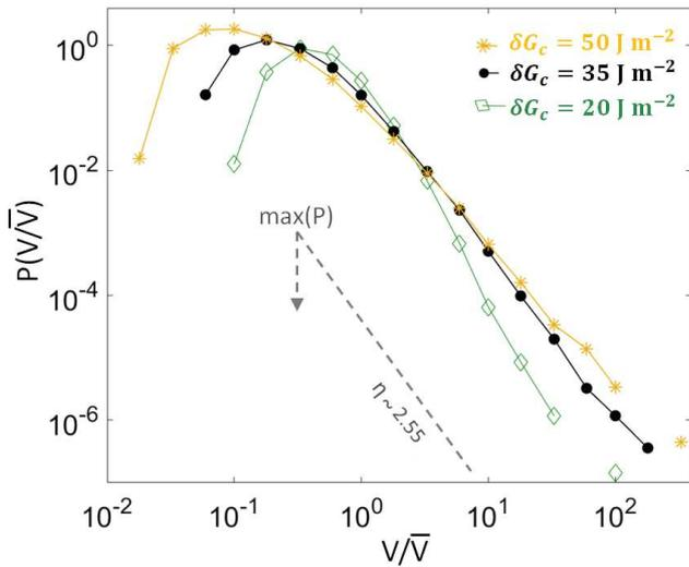
FIG. 8. Probability density function of the local propagation velocity along simulated fronts with three different values of  $\delta G_c = 20 \text{ J m}^{-2}$ . We chose the value of  $\delta G_c$  by tuning it and fitting the slope and maximum of the experimental data, which are illustrated by the dashed line and arrow. The rest of the parameters used in these simulations are as defined in table I.
