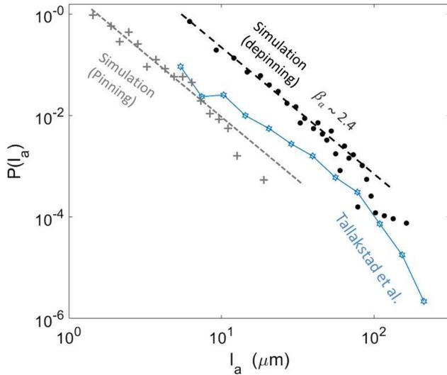
FIG. 17. Probability density function of the inline extent  $l_a$  of the modelled avalanche clusters (plain points) and of the modelled pinning clusters (crosses), for a threshold  $c = 3$ . The two straight dashed lines have a slope  $\beta_x \sim 2.4$ , inline with that of the experimental data Tallakstad et al. [19] for the pinning clusters (hollow stars, from their Fig. 16b, inset,  $c=3$ ).
