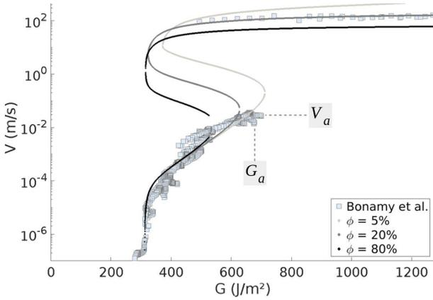
FIG. 12. Effect of varying the ratio of energy converted to heat,  $\phi$ , on the fit to the PMMA data. The maximum velocity increases with  $\phi$  as the tip temperature is higher. The threshold from the slow to the fast branch (i.e., the  $(G_a, V_a)$  point) shifts towards a lower  $G$  as a lighter load is required for the temperature to significantly deviate from  $T_0$ .
