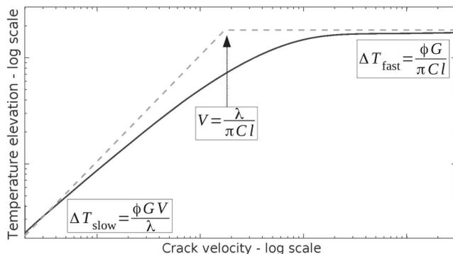
FIG. 2. Steady thermal elevation at a crack tip for various propagation velocities, due to the diffusion equation (5) (plain plot). The approximations  $\Delta T_{\text{fast}}$  and  $\Delta T_{\text{slow}}$ , from Eqs. (6) and (7), are shown for comparison (dotted plots). The axes are not annotated for the sake of generality.
