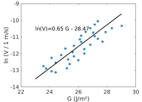
FIG. 6. Creep data of Scioto sandstone, from Holder et al. (6), figure 3.
