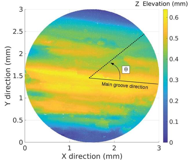
FIG. 2. White light interferometry topography of the Corona Heights fault plane at the millimeter scale. This surface is called  $S_{mm}$ , has a radius of 1.5 mm and is defined on a 2  $\mu$ m grid with a 0.025  $\mu$ m elevation resolution. A parametric angle  $\theta$  is defined from the main groove direction.
