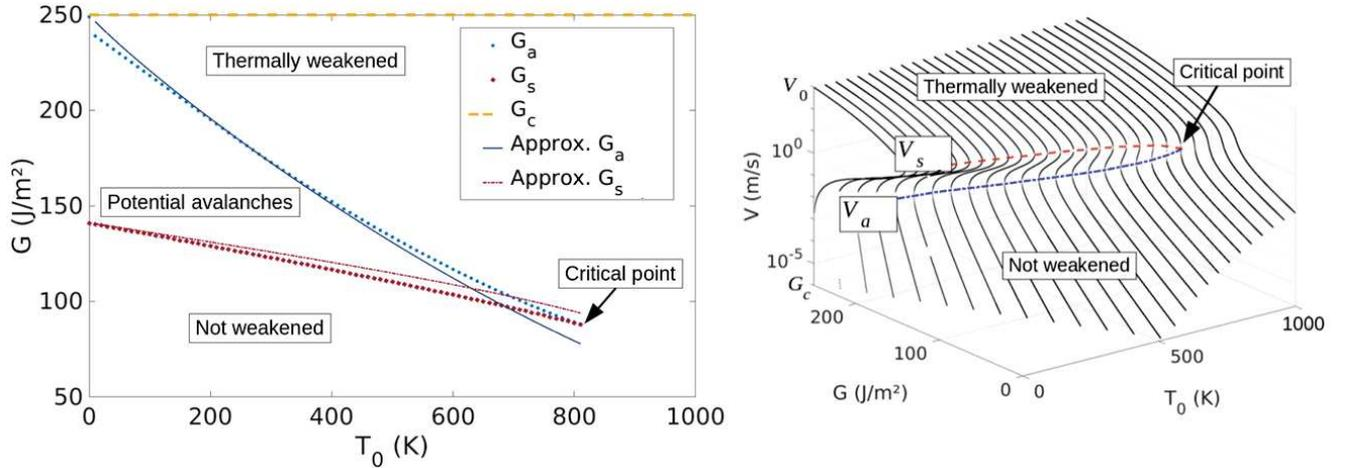
FIG. 1. (left):  $G_a$  and  $G_s$  as functions of the ambient temperature  $T_0$ , both solved numerically as well as using the approximate equations (2) and (4). One can notice the critical point which the approximations are failing to recover quantitatively. The horizontal dashed line at the top is for  $G = G_c$  domain. Note: this plot is a top view of the phase diagram of Vincent-Dospital et al. [1], which I have reinserted here (plot on the right).
