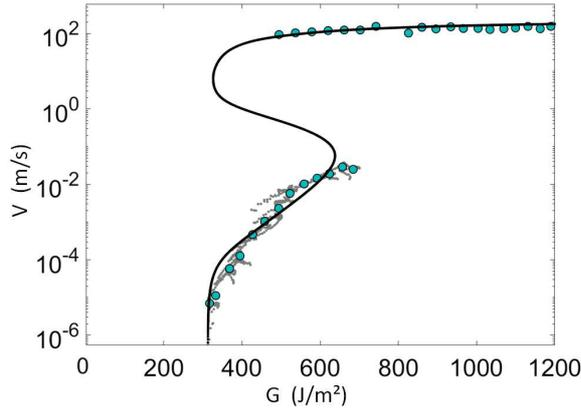
FIG. 15. Under sampled PMMA data (blue circles), using a running average on  $40 \text{ J m}^{-2}$  bins. The dots are the original data points and the black line the fitted model. With this decimated data set, the mean fitting error is  $\bar{\varepsilon} = 4\%$ . The data is only shown to the onset of micro-cracking (i.e., see section III B), beyond which the model does not apply as such.
