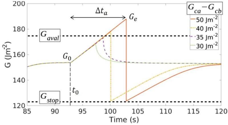
FIG. 2. Numerical simulations for a crack overcoming a rectangular asperity in fracture energy  $G_e$ , for various anomaly strengths  $G_{ca} - G_{cb}$ . The time and load on the entrance of the asperity are  $t_0$  and  $G_0$ . The time needed to overcome it is  $\Delta t_a$  and the load on it exit is  $G_e$ . These two latter parameters are approximated by Eqs. (8) and (9).
