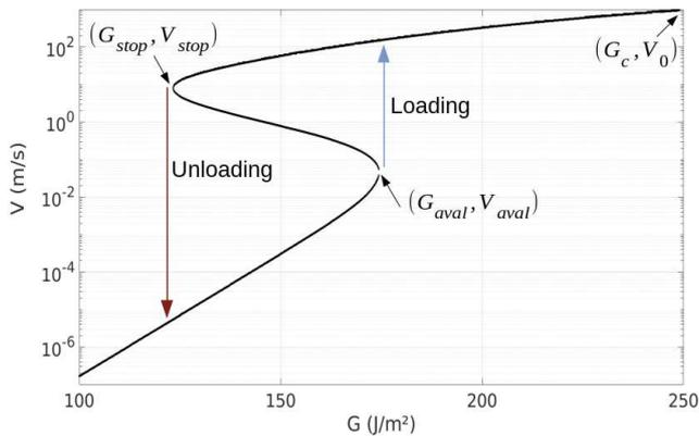
FIG. 3. Solutions for the crack velocity as a function of  $G$  for  $T_0 = 293$  K. All solutions in between  $V_{stop}$  and  $V_{aval}$  are unstable, any other point is a possible crack velocity. The arrows represent how a crack avalanches or slows down at the phase transition thresholds.
