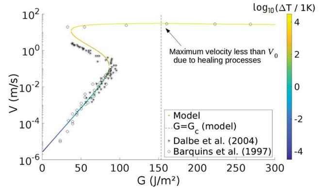
FIG. 17. Fit of the Scotch<sup>®</sup> 3M 600 data [19, 37] with a model including healing processes. The unstable (middle) branch of the model should not necessarily match the data point which are averaged  $G$  and  $V$  values for a front that stick-slips.
