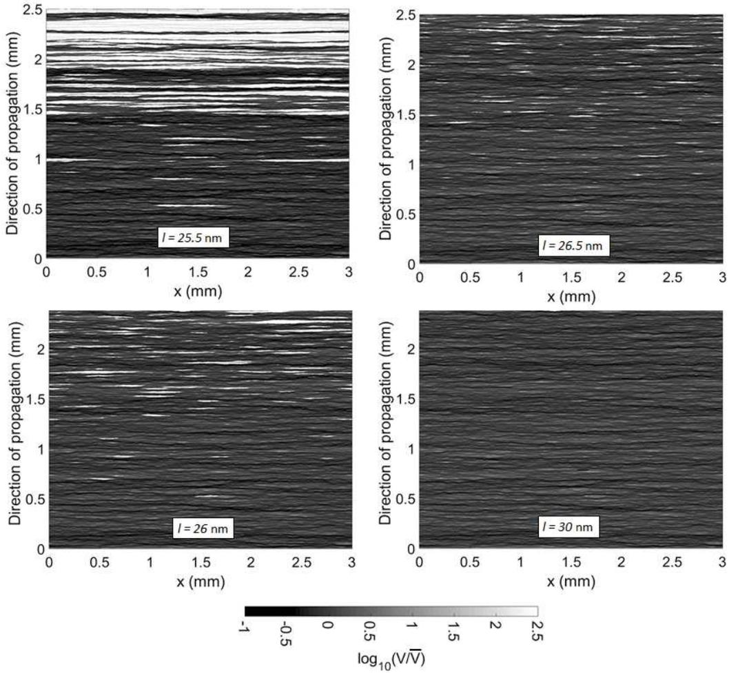
FIG. 3. Spatial crack velocity map for three different sizes  $l$  of the thermal production zone. The average velocity for the creeping zones is  $\bar{V} = 6 \text{ mm s}^{-1}$ . The white areas are thermal avalanches which velocity can reach up to  $200 \text{ m s}^{-1}$ .
