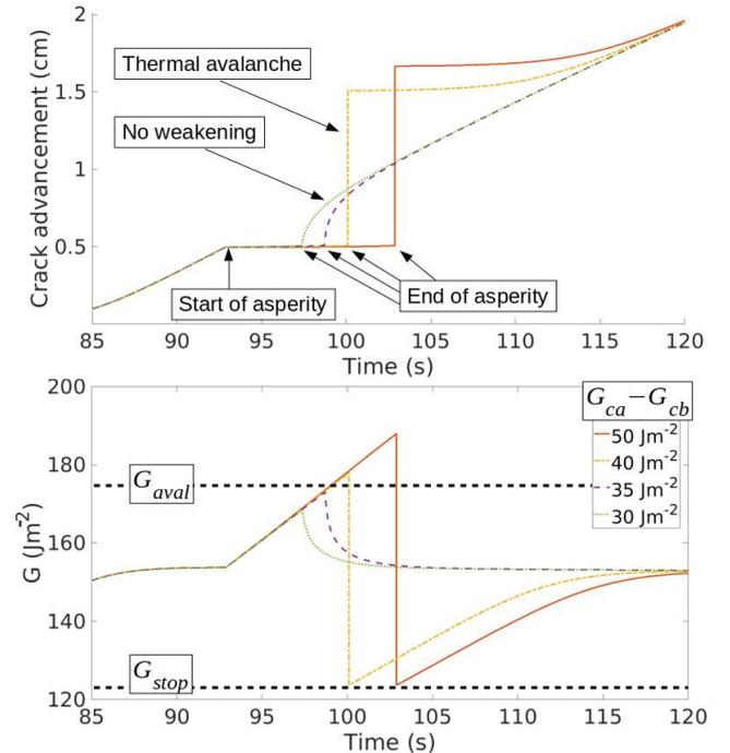
FIG. 6. Numerical simulations for a crack overcoming an asperity as defined by the differential equation from (3) and (10) and for various  $G_{c_a}$ .  $L_a = 100 \mu\text{m}$ ,  $v_u = 120 \mu\text{m s}^{-1}$ ,  $h = 5 \text{ mm}$  and  $E = 3.2 \text{ GPa}$ . The top plot is the crack advancement  $a(t)$ , the bottom one is the energy release rate  $G(t)$ . Thermal weakening is or is not triggered depending on the anomaly strength.
