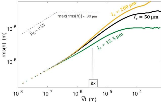
FIG. 6. Standard deviation of the width evolution of the crack front as a function of the mean crack advancement, as defined by Eqs. (3) and (4) for simulations with different correlation lengths  $l_c$ . The rest of the parameters are as defined in table I. The slope and plateau of the experimental data (shown in Fig. 5) is marked by the dashed line for comparison.
