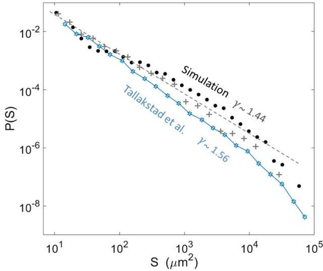
FIG. 13. Probability density function of the surface of the modelled avalanche clusters (plain points) and of the modelled pinning clusters (crosses), for a threshold  $c = 3$ . The straight dashed line has a slope  $\gamma \sim 1.44$ , as per Eq. (14). For comparison, the hollow stars shows the experimental probability density function obtained by Tallakstad et al. [19] for the avalanche and pinning clusters (Both are overlapping, see Fig. 10 of their manuscript).
