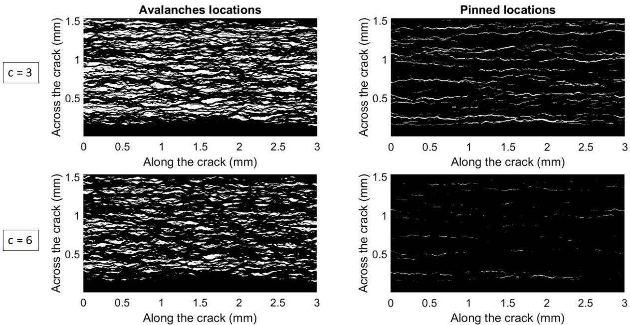
FIG. 11. Positions of the avalanches (left) and pinning locations (right) in the front local velocity map  $V(x, a)$  shown in Fig. 9 a, as per Eqs. (12) and (13). Two thresholds are here used to define these maps relatively to the mean velocity:  $c = 3$  (top) and  $c = 6$  (bottom). The white areas are the locations of interests, of surfaces  $S$ , crossline extents  $l_x$  and inline extents  $l_a$ .
