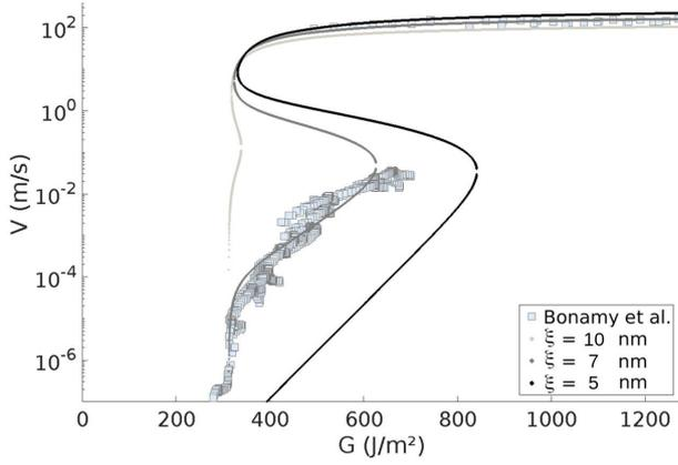
FIG. 11. Effect of varying the stress cut-off scale  $\xi$ , on the fit to the PMMA data.  $\xi$  mainly controls the slope and the intercept of the low velocity branch. A small change in  $\xi$  significantly modifies this branch as well as the threshold to the fast regime.
