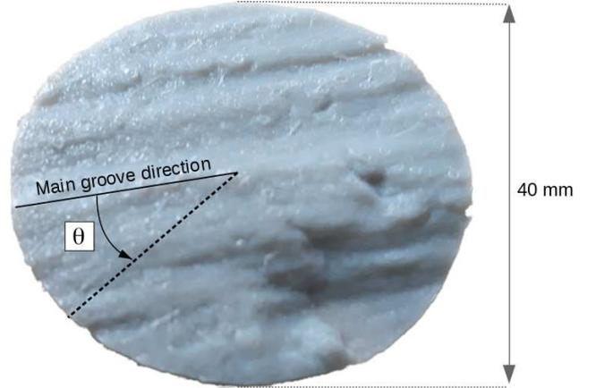
FIG. 3. Polyactic Acid 3D-print of  $S_m$ .
