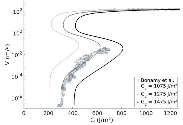
FIG. 9. Effect of varying the breaking energy barrier,  $G_c$ , on the fit to the PMMA data. At a given load  $G$ , the higher  $G_c$ , the slower the crack. The transitions between the three propagation modes (fast, slow, and dominated by healing) are also affected: a medium with a stronger barrier needs a heavier load to transit to a weaker state.
