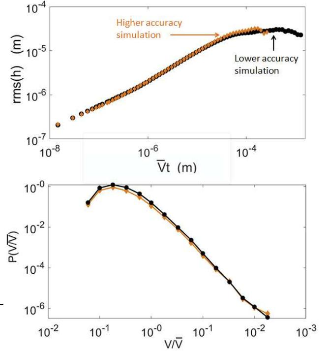
FIG. 20. Crack growth (top) and velocity distribution (bottom) for two simulations with the same physical parameters but different numerical accuracy, as per table III. The points are data from the simulation analysed in this manuscript and the squares were computed on coarser numerical grids. The computed exponents are not significantly affected.
