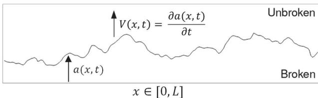
FIG. 1. Crack front  $a$  and crack velocity profile  $V$ , as defined in this manuscript. The front is supposed to have periodic boundary conditions along  $x$ , the coordinate perpendicular to the direction of propagation. The time variable is denoted  $t$ . This figure is a top view of Fig. 2.
