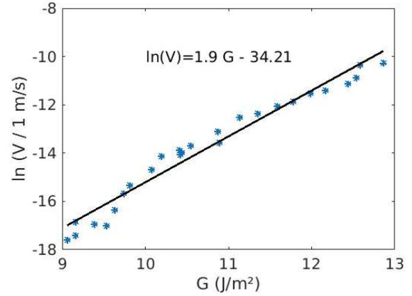
FIG. 5. Creep data of quartz in vacuum, from Dove (5), figure 4.
