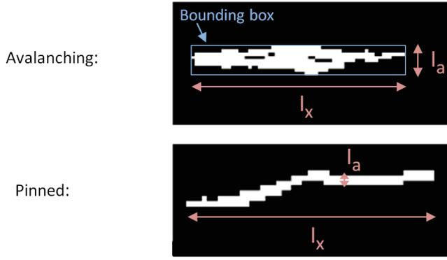
FIG. 12. Difference in definition of  $l_a$  for the avalanche (or depinning) and pinning clusters shown in Fig. 11. For the former,  $l_a$  is the maximum extent along the  $a$  direction. For the latter it is the average width in the same direction. In both cases,  $l_x$  is the maximum extent along the  $x$  direction and  $S$  the full surface (in white) of the cluster. The square pattern marks the pixel size ( $\Delta x = \Delta a = 3 \mu\text{m}$ ).
