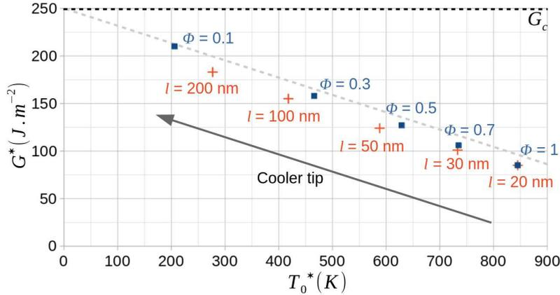
FIG. 2. Critical point location with varying  $\phi$  and  $l$ . Points are for  $l = 20$  nm and varying  $\phi$ . Crosses are for  $\phi = 1$  and varying  $l$ . The dotted line is the domain defined by Eq. (7):  $\alpha^2(G_c - G^*) = 8k_b T_0^*$ . Of course, the warmer a crack front (for higher  $\phi$  and smaller  $l$ ), the higher is the critical temperature. The horizontal dashed line at the top is for  $G = G_c$  domain.
