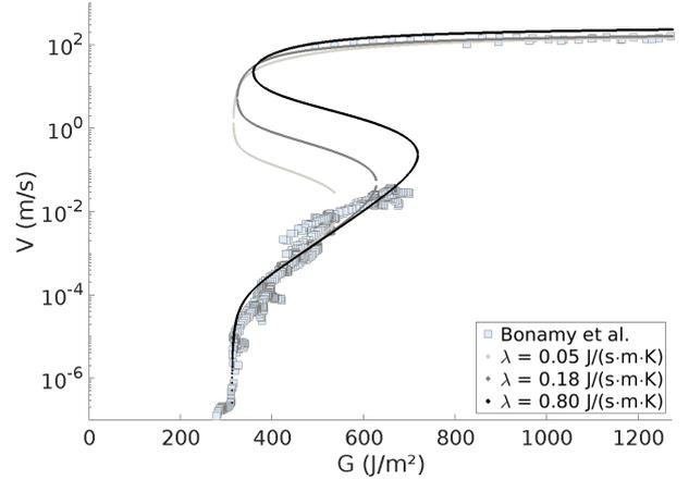
FIG. 13. Effect of varying the thermal conductivity,  $\lambda$ , on the fit to the PMMA data. With a higher  $\lambda$ , the heat is better evacuated: the slow to fast branch threshold shifts towards higher  $G$  and  $V$ . The fast regime is not very sensitive to  $\lambda$ , as  $\Delta T$  is there constrained by  $l$ .
