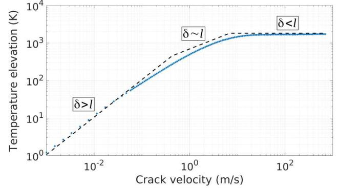
FIG. 2. Steady state values of the temperature elevation (blue dots) obtained by solving the diffusion equation (1) for a crack propagating at constant velocity for  $\phi G = 200 \text{ J m}^{-2}$ . The plotted asymptotes are the approximations (pre-factors included) from Eq. (3) to Eq. (5).
