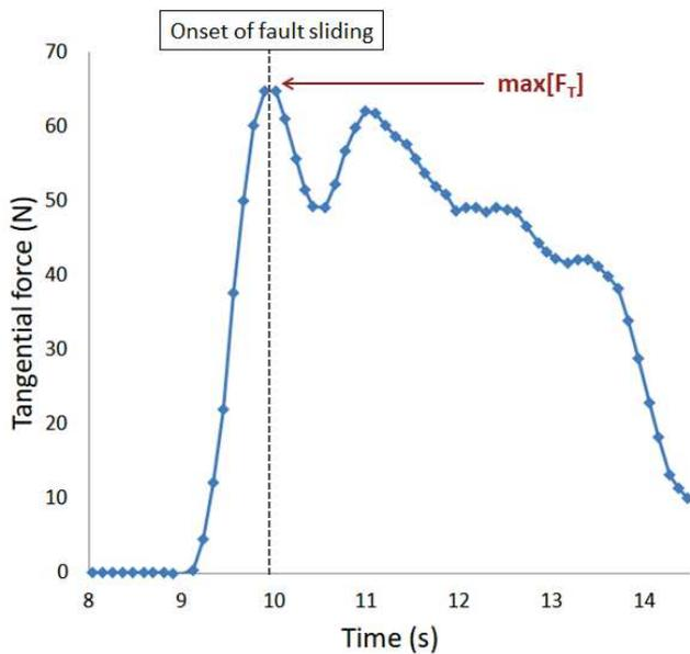
FIG. 6. Typical tangential force versus time for a given slide angle ( $\theta = 90^\circ$ ) and a given normal force ( $F_N = 4.9$  N) applied to the  $S_m$  fault. From the maximal value of the tangential force, a friction coefficient  $\mu_s(4.9 \text{ N}, 90^\circ) = 12.9$  can here be determined, as per Eq. (2).
