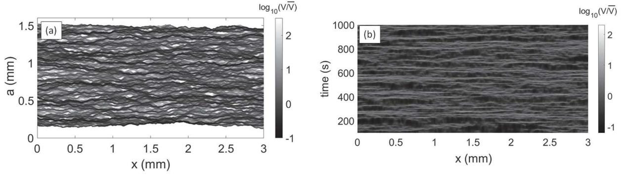
FIG. 9. Local velocity maps  $V(x, a)$  in the space-space domain (left) and  $V(x, t)$  in the space-time domain (right). Both maps are computed on a resolution similar to that of the experiments by Tallakstad et al. [19], using the waiting time matrix. The velocity are plotted related to the average crack velocity  $\bar{V} = 1.5 \mu\text{m s}^{-1}$ . Both maps are shown with the same color scale. All parameters used to run the corresponding simulation are summarised in table I.
