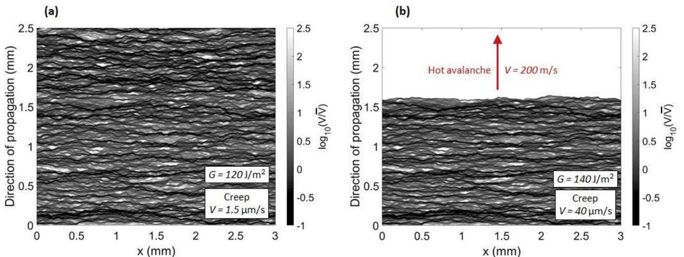
FIG. 1. Spatial crack velocity map for a mean energy release rate of  $120 \text{ J m}^{-2}$  (top) and  $14 \text{ J m}^{-2}$  (bottom), with the same parameters as in the preceding article and thermal parameters from Vincent-Dospital et al. [1]. In the latter case, a thermal avalanche is triggered (Large white area, with an average velocity of  $200 \text{ m s}^{-1}$ ). The mean velocity defining the colour scale is that of the creep (slow) phase, without an avalanche.
