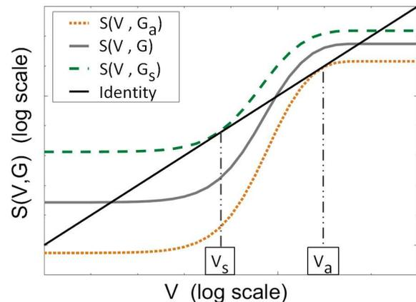
FIG. 1. Representation of  $V = S(V, G)$  for three values of  $G$ :  $G_s$ ,  $G_a$  and a mid-value between  $G_s$  and  $G_a$  (plain plot). The intersections of  $S_G$  with the identity plot (straight line) give the possible crack velocities for a given energy release rate, as per Eq. (4). The axes are not annotated for the sake of generality. See Ref. (2) for further information.
