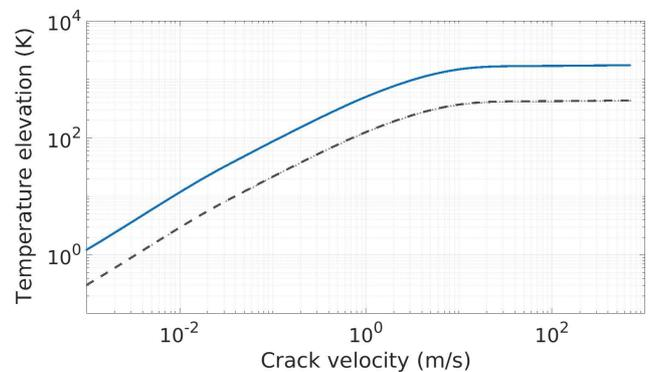
FIG. 1. Steady state values of the temperature elevation. It is obtained by solving Eq. (2) for a crack propagating at constant velocity and for  $\phi G = 200 \text{ J m}^{-2}$  (plain plot) and  $\phi G = 50 \text{ J m}^{-2}$  (dotted plot).
