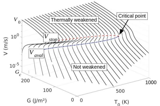
FIG. 4. Solutions for the crack velocity as a function of  $G$  and for various  $T_0$ . The dashed lines show the  $(V_{stop}, G_{stop})$  and  $(V_{aval}, G_{aval})$  couples and converge to the critical point.
