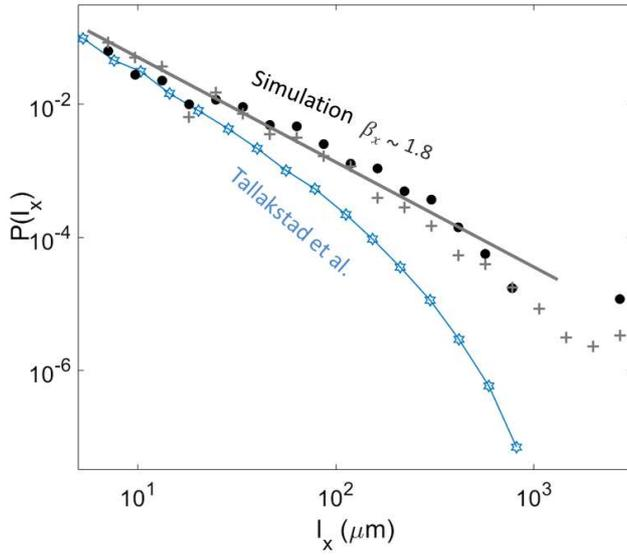
FIG. 16. Probability density function of the crossline extent  $l_x$  of the modelled avalanche clusters (plain points) and of the modelled pinning clusters (crosses), for a threshold  $c = 3$ . The straight line has a slope  $\beta_x \sim 1.8$ , as per Eq. (15). The hollow stars shows the experimental probability density function obtained by Tallakstad et al. [19] for the pinning clusters (from their Fig. 16a, inset,  $c=3$ ).
