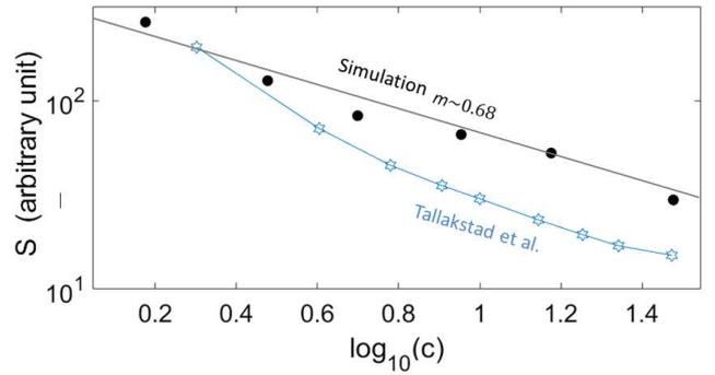
FIG. 15. Variation of the mean avalanche size  $\bar{S}$  as a function of the threshold  $c$  for the simulation (plain points) and the experiments (hollow stars). The modelled  $\bar{S}$  is expressed in pixels (one pixel is  $9 \mu\text{m}^2$ ) and the experimental  $\bar{S}$  reported by Tallakstad et al. [19] (on their Fig. 13) is in an arbitrary unit, so that the magnitude of both should not here be compared. The straight line has a slope 0.68.
