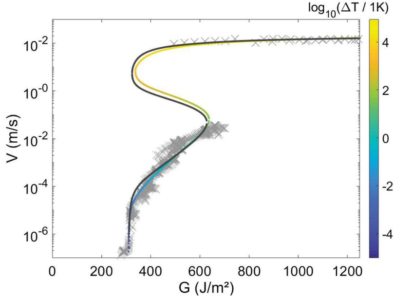
FIG. 1. Model fit to the PMMA data (squares), when considering the sub-critical growth law of Eq. (6) (colored curve, where the colormap describe the tip temperature elevation) or considering the simpler Arrhenius formalism instead (black curve, as considered in the core article). The fit quality in both cases is similar.
