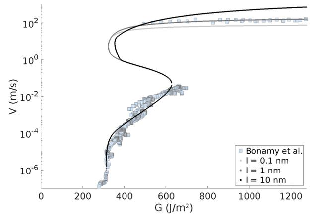
FIG. 14. Effect of varying the heat production zone radius,  $l$ , on the fit to the PMMA data.  $l$  mainly impacts the plot curvature on the high velocity branch. No effect is observed on the slow branch, as the thermal elevation there is constrained by the diffusion skin depth rather than by  $l$  (see Eq. (6)).
