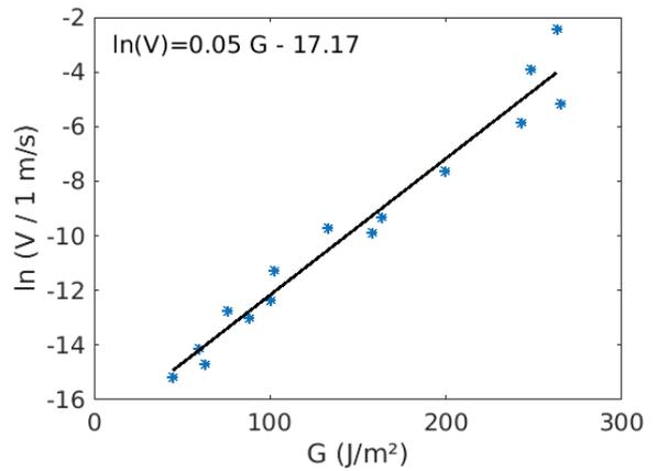
FIG. 13. Creep data of hot silicon nitride at 1200 °C, from Evans and Wiederhorn (13), figure 5.
