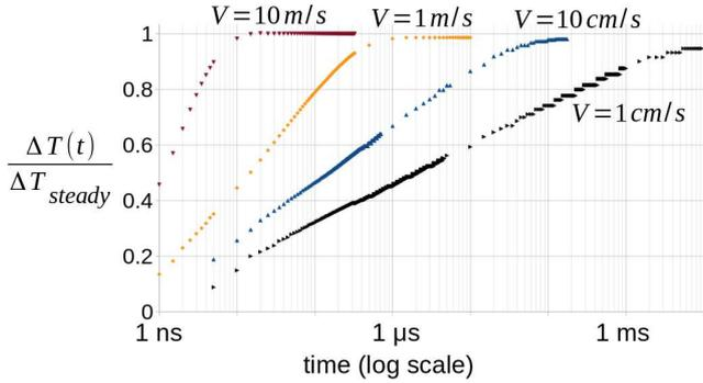
FIG. 3. Transient response for the heating of a crack propagating at constant  $V$  and  $G$ . The ratio of the tip temperature elevation and its steady state is shown for various velocities. One can read the actual value of  $\Delta T_{\text{steady}}$  in Fig. 2.
