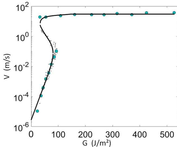
FIG. 16. Under sampled PSA data (blue circles), using a running average on  $10 \text{ J m}^{-2}$  bins. The dots are the original data points and the black line the fitted model. With this decimated data set, the mean fitting error is  $\bar{\varepsilon} = 5\%$ .
