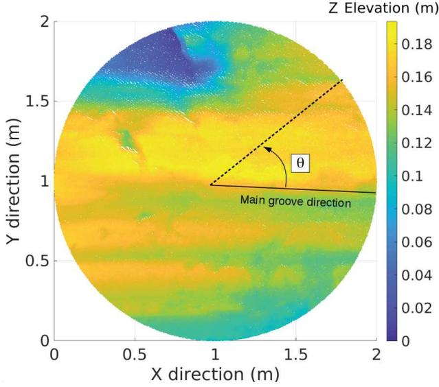
FIG. 1. Topography (i.e. roughness) of the Corona Heights fault at the meter scale [32]. This surface is called  $S_m$ , has a radius of 1 m and is defined on a 5 mm grid with a 1.25 mm elevation resolution. A parametric angle  $\theta$  is defined from the main groove direction.
