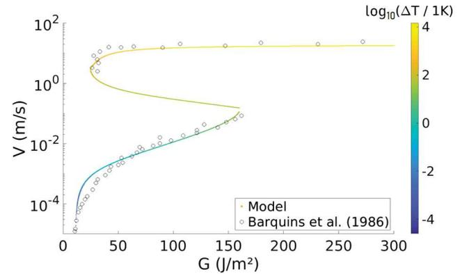
FIG. 18. Fit of the peeling data for another roller tape: Scotch<sup>®</sup> 3M 602 data [95]. The lack of linearity at low velocity calls for healing processes in our model. Note also the curvature on the lower end of the high velocity branch, not present in the other data sets that we show but rather compatible with our proposed model.
