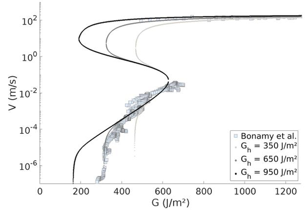
FIG. 10. Effect of varying the healing energy barrier,  $G_h$ , on the fit to the PMMA data. A crack that heals more easily needs a higher load to actually propagate forward or to stay in the high velocity regime.
