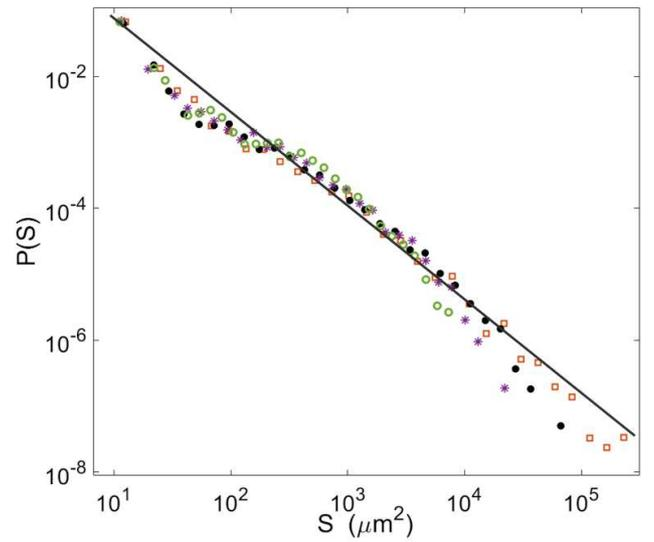
FIG. 14. Probability density function of the surface of the modelled avalanche clusters for various  $c$  values:  $c = 1.5$  (squares),  $c = 3$  (plain points),  $c = 6$  (stars),  $c = 12$  (circles). The straight line has a slope  $\gamma \sim 1.4$ , as per Eq. (14).
