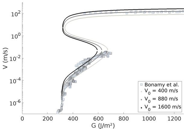
FIG. 8. Effect of varying the nominal velocity,  $V_0$ , on the fit to the PMMA data. The propagation velocity is roughly proportional to  $V_0$ , but also modifies the positions of the phase transitions.
