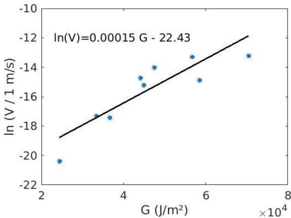
FIG. 17. Creep data of high density polyethylene, from Yoda et al. (17), figure 4.
