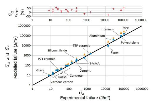
FIG. 3. (Bottom): Modelled  $G_a$  thresholds (squares) and modelled surface energy barrier  $G_c$  (triangles) compared to the experimental thresholds from the literature. The black line is the identity. The labels locate different materials. The unlabelled rock materials are quartz, sapphire, granite and andesite. See the supplementary material for an exhaustive list. (Top): Relative error on the avalanche threshold.
