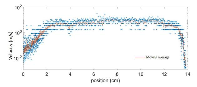
FIG. 7. Crack velocity as a function of the front position (dots). It is a crossplot of Figs. 4c and 4d. The plain line is a moving average.
