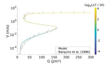
FIG. 18. Fit of the peeling data for another roller tape: Scotch® 3M 602 data [95]. The lack of linearity at low velocity calls for healing processes in our model. Note also the curvature on the lower end of the high velocity branch, not present in the other data sets that we show but rather compatible with our proposed model.
