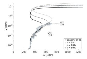
FIG. 12. Effect of varying the ratio of energy converted to heat,  $\phi$ , on the fit to the PMMA data. The maximum velocity increases with  $\phi$  as the tip temperature is higher. The threshold from the slow to the fast branch (i.e., the  $(G_a, V_a)$  point) shifts towards a lower G as a lighter load is required for the temperature to significantly deviate from  $T_0$ .
