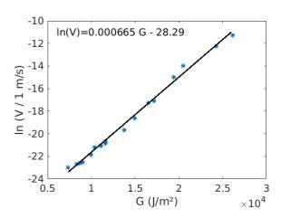
FIG. 18. Creep data of aluminium 2650 T6 alloy in vacuum at 175 °C, from Hénaff et al. (18), figure 6.
