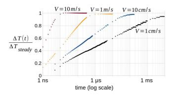
FIG. 3. Transient response for the heating of a crack propagating at constant V and G. The ratio of the tip temperature elevation and its steady state is shown for various velocities. One can read the actual value of  $\Delta T_{\rm steady}$  in Fig. 2.
