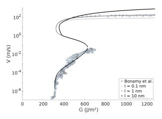
FIG. 14. Effect of varying the heat production zone radius, l, on the fit to the PMMA data. l mainly impacts the plot curvature on the high velocity branch. No effect is observed on the slow branch, as the thermal elevation there is constrained by the diffusion skin depth rather than by l (see Eq. (6)).
