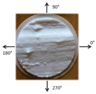
FIG. 7. 3D-print of a Dixie valley fault. The arrows correspond to given sliding directions during the friction tests, for which the coefficient of friction is summarised in Fig. 8. This plastic sample has a diameter of 5.5 cm, which is a magnification accounting for a real - field measured - diameter of 1 mm.
