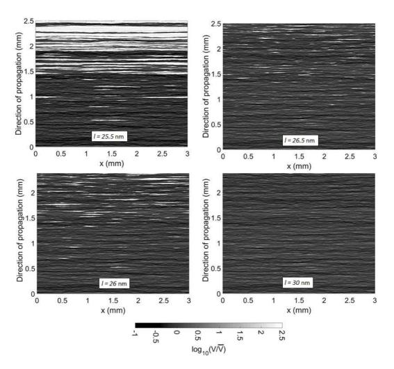
FIG. 3. Spatial crack velocity map for three different sizes l of the thermal production zone. The average velocity for the creeping zones is  $\overline{V} = 6\,\mathrm{mm\,s^{-1}}$ . The white areas are thermal avalanches which velocity can reach up to  $200\,\mathrm{m\,s^{-1}}$ .
