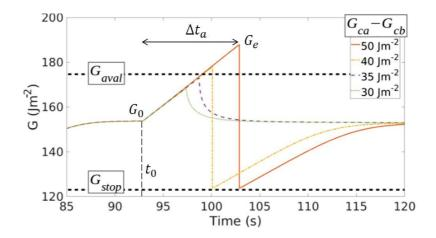
FIG. 2. Numerical simulations for a crack overcoming a rectangular asperity in fracture energy  $G_c$ , for various anomaly strengths  $G_{ca} - G_{cb}$ . The time and load on the entrance of the asperity are  $t_0$  and  $G_0$ . The time needed to overcome it is  $\Delta t_a$  and the load on it exit is  $G_e$ . These two latter parameters are approximated by Eqs. (8) and (9).
