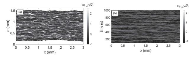
FIG. 9. Local velocity maps V(x,a) in the space-space domain (left) and V(x,t) in the space-time domain (right). Both maps are computed on a resolution similar to that of the experiments by Tallakstad et al. [19], using the waiting time matrix. The velocity are plotted related to the average crack velocity  $\overline{V} = 1.5 \, \mu \mathrm{m \, s^{-1}}$ . Both maps are shown with the same color scale. All parameters used to run the corresponding simulation are summarised in table I.
