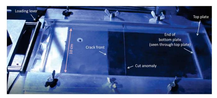
FIG. 5. Top view of the experimental setp-up for the interfacial rupture of PMMA.
