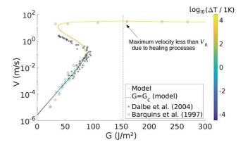
FIG. 17. Fit of the Scotch<sup>®</sup> 3M 600 data [19, 37] with a model including healing processes. The unstable (middle) branch of the model should not necessarily match the data point which are averaged G and V values for a front that stick-slips.
