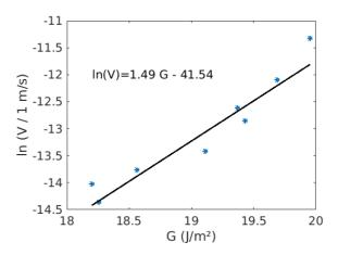
FIG. 4. Creep data of dry sapphire (r-plane), from Wiederhorn and Krause (4).
