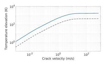
FIG. 1. Steady state values of the temperature elevation. It is obtained by solving Eq. (2) for a crack propagating at constant velocity and for  $\phi G = 200\,\mathrm{J\,m^{-2}}$  (plain plot) and  $\phi G = 50\,\mathrm{J\,m^{-2}}$  (dotted plot).
