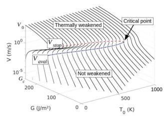
FIG. 4. Solutions for the crack velocity as a function of G and for various  $T_0$ . The dashed lines show the  $(V_{\text{stop}}, G_{\text{stop}})$  and  $(V_{\text{aval}}, G_{\text{aval}})$  couples and converge to the critical point.
