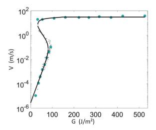
FIG. 16. Under sampled PSA data (blue circles), using a running average on  $10\,\mathrm{J\,m^{-2}}$  bins. The dots are the original data points and the black line the fitted model. With this decimated data set, the mean fitting error is  $\overline{\varepsilon}=5\%$ .
