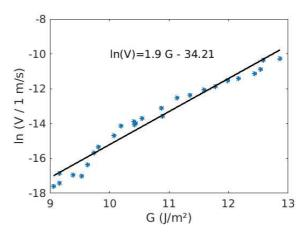
FIG. 5. Creep data of quartz in vacuum, from Dove (5), figure 4.
