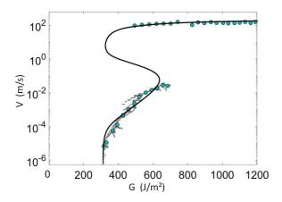
FIG. 15. Under sampled PMMA data (blue circles), using a running average on  $40\,\mathrm{J\,m^{-2}}$  bins. The dots are the original data points and the black line the fitted model. With this decimated data set, the mean fitting error is  $\bar{\varepsilon}=4\%$ . The data is only shown to the onset of micro-cracking (i.e., see section III B), beyond which the model does not apply as such.
