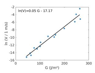
FIG. 13. Creep data of hot silicon nitride at  $1200\,^{\circ}\,\mathrm{C}$ , from Evans and Wiederhorn (13), figure 5.
