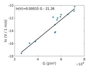
FIG. 19. Creep data in Ti-6A1-6V-2Sn titanium alloy in moist air, from Sastry et al. (19), figure 6a (beta annealed).
