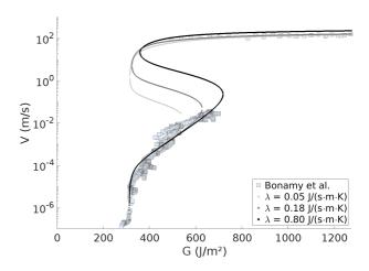
FIG. 13. Effect of varying the thermal conductivity,  $\lambda$ , on the fit to the PMMA data. With a higher  $\lambda$ , the heat is better evacuated: the slow to fast branch threshold shifts towards higher G and V. The fast regime is not very sensitive to  $\lambda$ , as  $\Delta T$  is there constrained by l.
