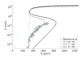
FIG. 11. Effect of varying the stress cut-off scale  $\xi$ , on the fit to the PMMA data.  $\xi$  mainly controls the slope and the intercept of the low velocity branch. A small change in  $\xi$  significantly modifies this branch as well as the threshold to the fast regime.
