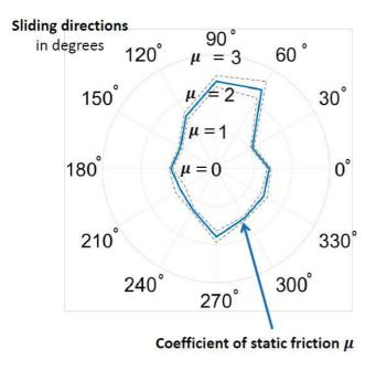
FIG. 8. Anisotropy of the static coefficient of friction for the surface presented in Fig. 7. The plain line is an average of three different tests and the width between the dotted line is the standard deviation. A clear anisotropy, exceeding the noise level, is shown.
