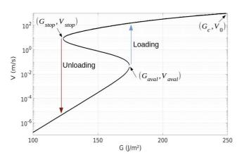
FIG. 3. Solutions for the crack velocity as a function of G for  $T_0=293\,\mathrm{K}$ . All solutions in between  $V_{\mathrm{stop}}$  and  $V_{\mathrm{aval}}$  are unstable, any other point is a possible crack velocity. The arrows represent how a crack avalanches of slows down at the phase transition thresholds.
