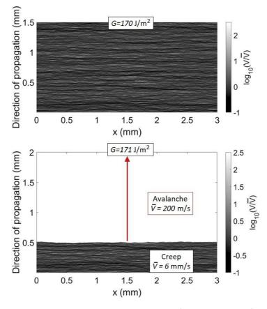
FIG. 2. Spatial crack velocity map for a mean energy release rate of  $170\,\mathrm{J\,m^{-2}}$  (top) and  $171\,\mathrm{J\,m^{-2}}$  (bottom), with the parameters described in section II. In the latter case, a thermal avalanche is triggered (white area, with an average velocity of  $200\,\mathrm{m\,s^{-1}}$ ). The mean velocity defining the colour scale is that of the creep (slow) phase, without an avalanche:  $\overline{V} = 6\,\mathrm{mm\,s^{-1}}$ .
