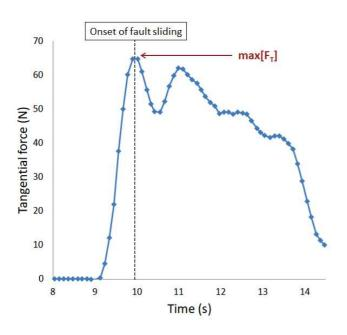
FIG. 6. Typical tangential force versus time for a given slide angle ( $\theta = 90^{\circ}$ ) and a given normal force ( $F_N = 4.9 \text{ N}$ ) applied to the  $S_m$  fault. From the maximal value of the tangential force, a friction coefficient  $\mu_s(4.9 \text{ N}, 90^{\circ}) = 12.9$  can here be determined, as per Eq. (2).
