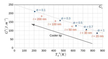
FIG. 2. Critical point location with varying  $\phi$  and l. Points are for  $l=20\,\mathrm{nm}$  and varying  $\phi$ . Crosses are for  $\phi=1$  and varying l. The dotted line is the domain defined by Eq. (7):  $\alpha^2(G_c-G^*)=8k_bT_0^*$ . Of course, the warmer a crack front (for higher  $\phi$  and smaller l), the higher is the critical temperature. The horizontal dashed line at the top is for  $G=G_c$  domain.
