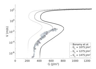
FIG. 9. Effect of varying the breaking energy barrier,  $G_c$ , on the fit to the PMMA data. At a given load G, the higher  $G_c$ , the slower the crack. The transitions between the three propagation modes (fast, slow, and dominated by healing) are also affected: a medium with a stronger barrier needs a heavier load to transit to a weaker state.
