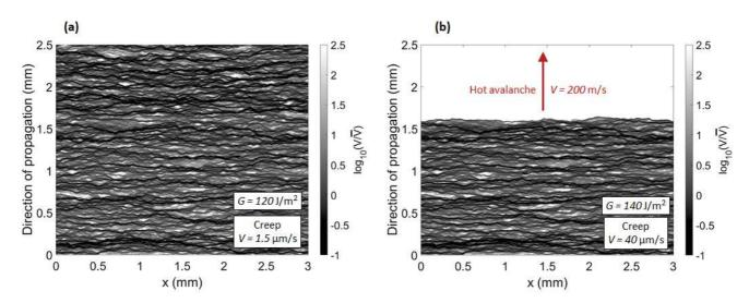
FIG. 1. Spatial crack velocity map for a mean energy release rate of  $120\,\mathrm{J\,m^{-2}}$  (top) and  $14\,\mathrm{J\,m^{-2}}$  (bottom), with the same parameters as in the preceding article and thermal parameters from Vincent-Dospital et al. [1]. In the latter case, a thermal avalanche is triggered (Large white area, with an average velocity of  $200\,\mathrm{m\,s^{-1}}$ ). The mean velocity defining the colour scale is that of the creep (slow) phase, without an avalanche.
