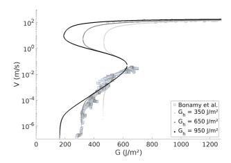
FIG. 10. Effect of varying the healing energy barrier,  $G_h$ , on the fit to the PMMA data. A crack that heals more easily needs a higher load to actually propagate forward or to stay in the high velocity regime.
