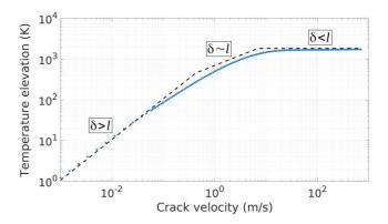
FIG. 2. Steady state values of the temperature elevation (blue dots) obtained by solving the diffusion equation (1) for a crack propagating at constant velocity for  $\phi G = 200 \,\mathrm{J\,m^{-2}}$ . The plotted asymptotes are the approximations (pre-factors included) from Eq. (3) to Eq. (5).
