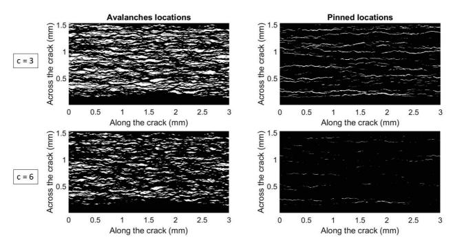
FIG. 11. Positions of the avalanches (left) and pinning locations (right) in the front local velocity map V(x, a) shown in Fig. 9 a, as per Eqs. (12) and (13). Two thresholds are here used to define these maps relatively to the mean velocity: c = 3 (top) and c = 6 (bottom). The white areas are the locations of interests, of surfaces S, crossline extents  $l_x$  and inline extents  $l_a$ .
