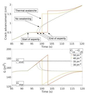
FIG. 6. Numerical simulations for a crack overcoming an asperity as defined by the differential equation from (3) and (10) and for various  $G_{c_a}$ .  $L_a=100\,\mu\mathrm{m}$ ,  $v_u=120\,\mu\mathrm{m}$  s<sup>-1</sup>,  $h=5\,\mathrm{mm}$  and  $E=3.2\,\mathrm{GPa}$ . The top plot is the crack advancement a(t), the bottom one is the energy release rate G(t). Thermal weakening is or is not triggered depending on the anomaly strength.
