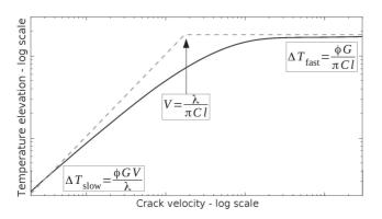
FIG. 2. Steady thermal elevation at a crack tip for various propagation velocities, due to the diffusion equation (5) (plain plot). The approximations  $\Delta T_{\rm fast}$  and  $\Delta T_{\rm slow}$ , from Eqs. (6) and (7), are shown for comparison (dotted plots). The axes are not annotated for the sake of generality.
