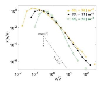
FIG. 8. Probability density function of the local propagation velocity along simulated fronts with three different values of  $\delta G_c = 20 \,\mathrm{J\,m^{-2}}$ . We chose the value of  $\delta G_c$  by tuning it and fitting the slope and maximum of the experimental data, which are illustrated by the dashed line and arrow. The rest of the parameters used in these simulations are as defined in table I.
