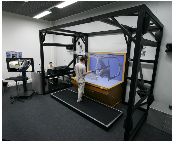
Figure 1.3 – The commercial solution Inca, a cable-driven haptic device from Haption [4].
