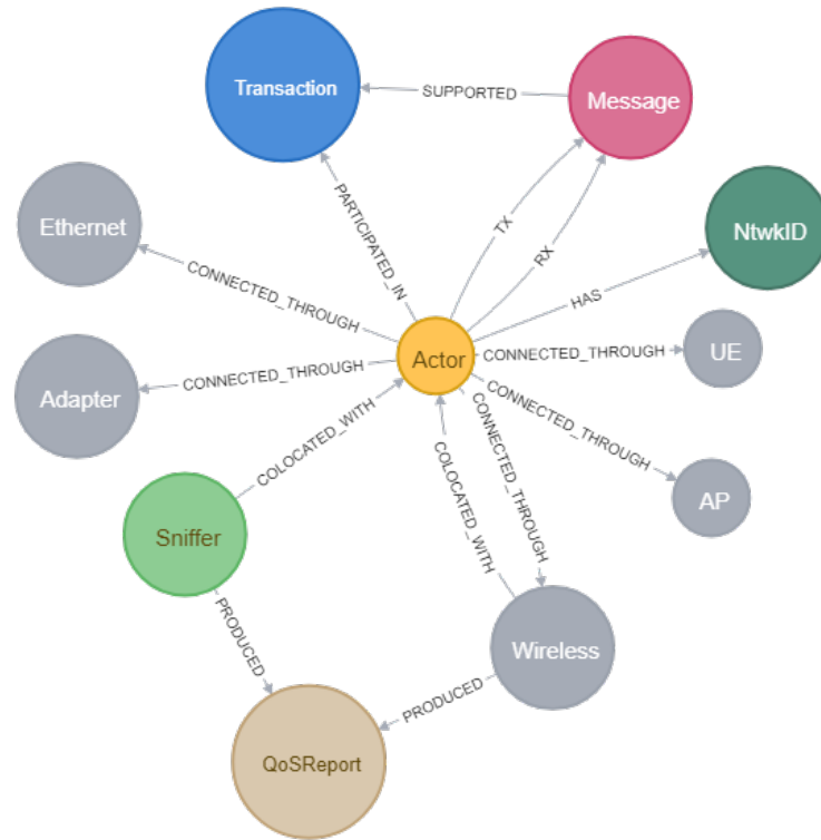
Figure 5.4: Realized schema of the GDB fully populated after capturing network and operational data from the NIST industrial wireless testbed. GDBs do not have enforced schemas; therefore, the schema depict represents the data as is.
