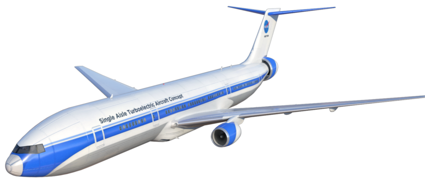
Figure III.4 – View of the STARC-ABL hybrid aircraft configuration, from Gray et al. [29]
