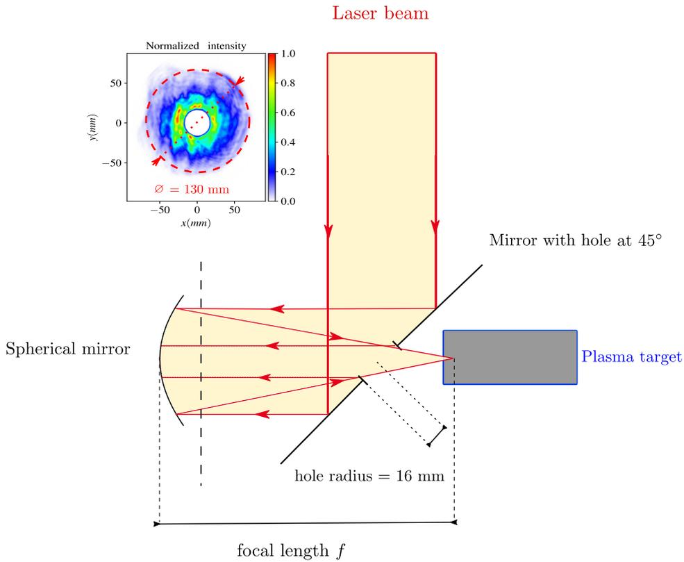
Figure 4.4: Schematic representation of the experimental set-up for the laser beam propagation and focusing in Apollon installation: a laser beam of a  $1/e^2$  diameter  $\simeq 130 mm$  is sent and reflected by a mirror at  $45^\circ$  presenting a hole of a radius =  $16 mm$  where a small fraction from the center of the laser is lost (estimated to be around  $\sim 12\%$ ). The beam is focused by a spherical mirror of a focal length  $f$ .
