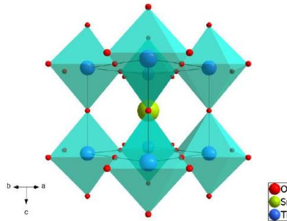
Figure I-2 : Structure Pérovskite SrTiO<sub>3</sub>.
