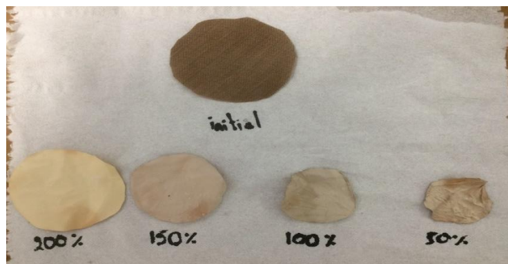
Figure 58. Photograph of ferrocene-doped ZIF-8 grown on cross-linked electrospun PBI nanofibers prepared with different amount of crosslinker as indicated in % compared to their initial size before deposition in MOF precursor solution.
